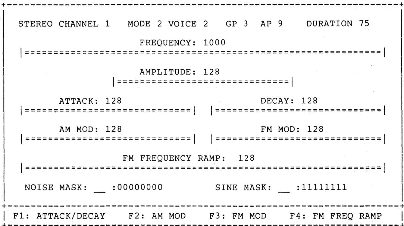
Note: Display shows the positions of the parameter scales; only a subset of these scales actually appears on the screen at any time.
