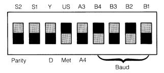
These settings, incidentally, are for no parity and a transmission rate of 9600 baud.
