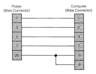
Note that cable pins 2 and 3 are cross-connected. Pin 20 at the plotter connector is connected to pins 5 and 6 at the computer connector.  $_{6-1}$
