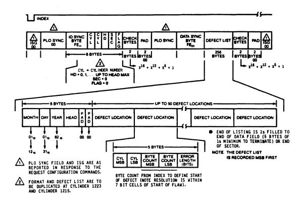
Figure 5-6. Defect List Format
