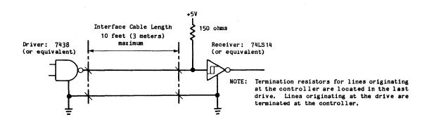
Figure 2-1. Control Signal Driver/Receiver Combination
