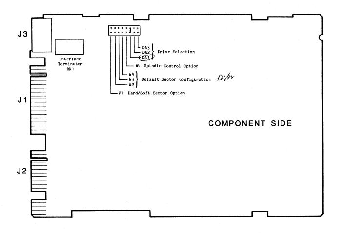
Figure 3-2. Option Jumpers and Interface Terminator
