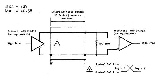
Figure 2-2. Data Line Driver/Receiver Combination
