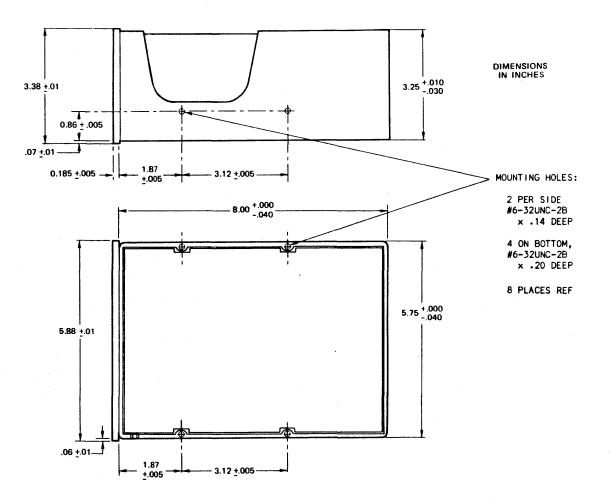
Figure 3-4. Dimensions and Mounting
