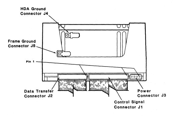
Figure 3-1. Power and Interface Connections
