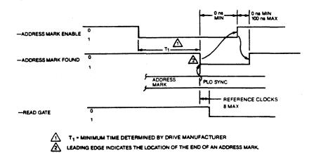
Figure 2-13. Read Address Mark Timing
