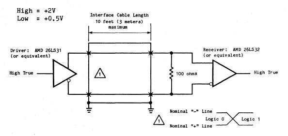
Figure 2-2. Data Line Driver/Receiver Combination
