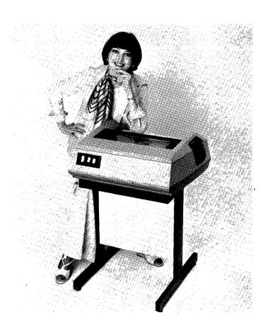
The new "optimized" bi-directional matrix serial printer that increases throughput two to three fold has been introduced by Tally Corp. The Model 1202 uses an internal 8080A microprocessor to compute the shortest distance to the next print position. The 120 cps unit prints left to right and right to left, slews at 7 ups, and moves the print head at an accelerated rate when not printing.
