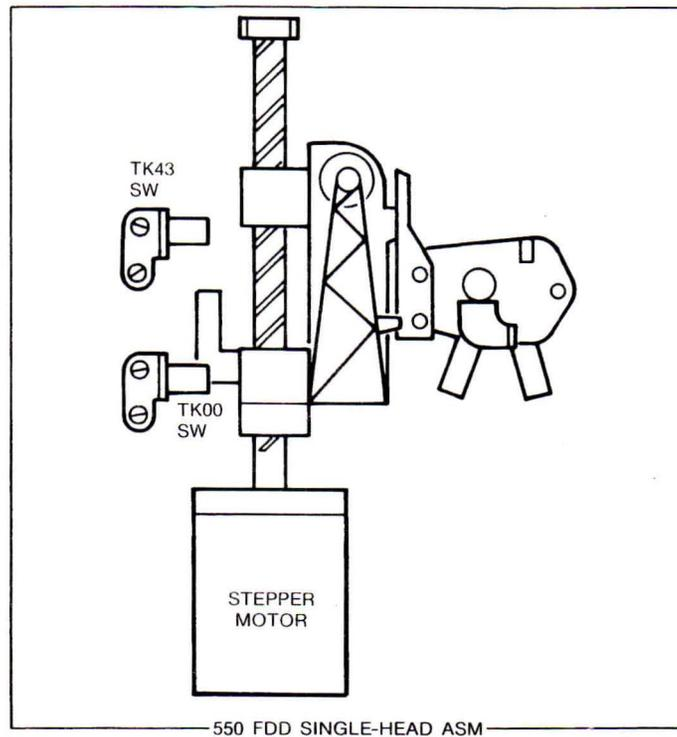
**FIGURE 2-2. 550/552 FLEXIBLE DISC DRIVE FUNCTIONAL DIAGRAM (Part 2 of 2)**
