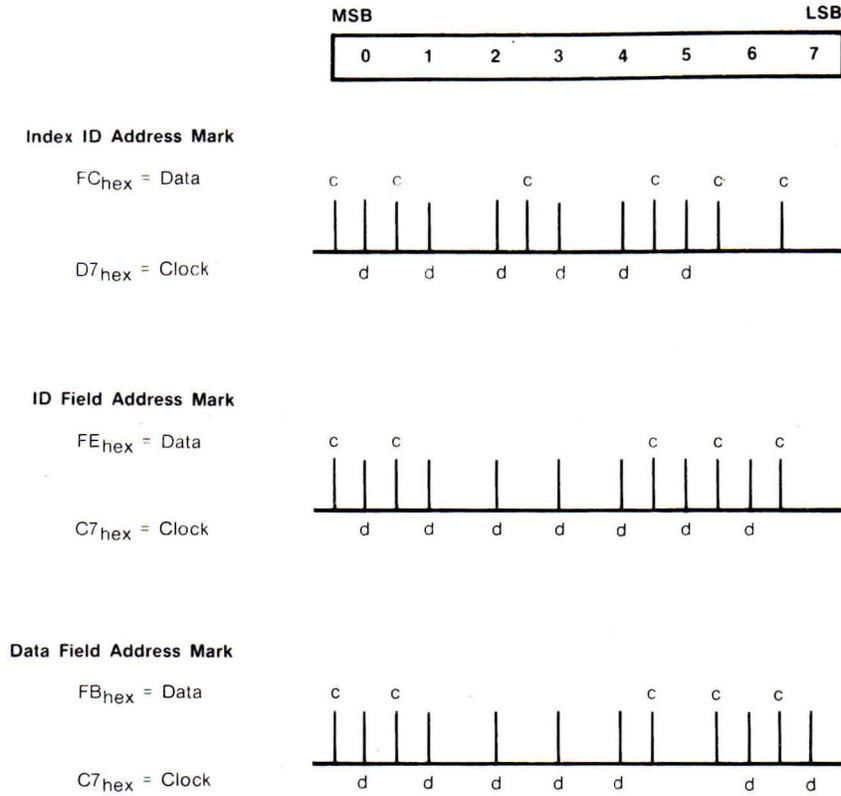
**FIGURE 4-5. SINGLE-HEAD UNIQUE ADDRESS MARKS**
