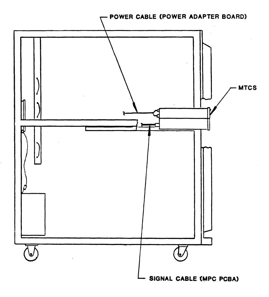
Figure 4-1. MTCS Cable Routing
