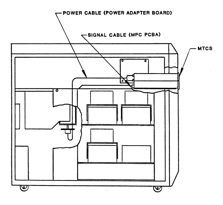
Figure 5-1. MTCS Cable Routing
