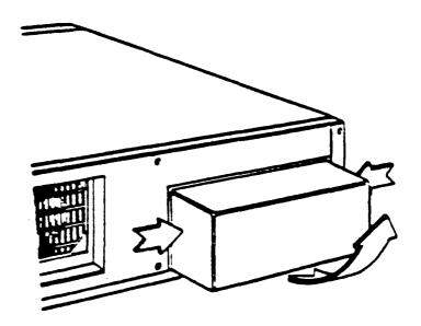
Figure 1-1. Cable Guard Removal/Replacement
