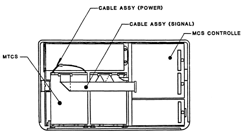
Figure 2-2. Cable Assembly Routing
