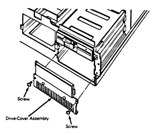
Figure 1-5. Cover Plate Removal
