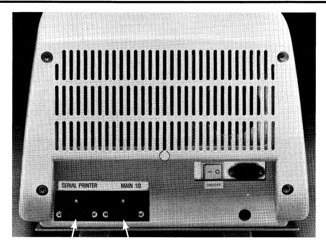
Figure 2-2. The Input/Output Ports
