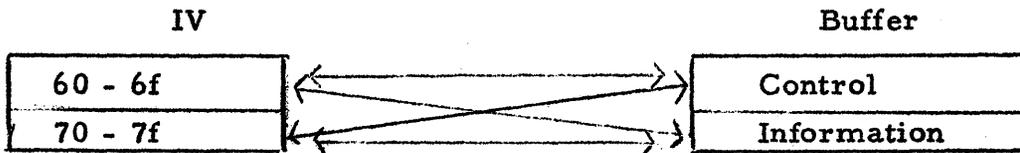
The control half contains pulses that indicate the card columns which correspond to each word of information, and also pulses that indicate in which of the three forms each word is to be interpreted --- alphabetic, hexadecimal, or decimal.
