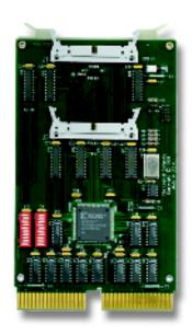
The DCQ-1100 is a plug and play replacement for Digital's DRV11-WA general purpose controller. The DCQ-1100 provides a 16-bit parallel user interface for PIO and DMA transfers between a Q-bus system and external equipment. It can also serve as a link between a Q-bus system and another computer with a DRV11-WA or DR11-W compatible interface.
