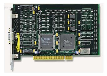
**Two Independent Timers.** Each timer can be independently programmed for an interval ranging from 50 microseconds to over 214 seconds in increments of 50 nanoseconds.
