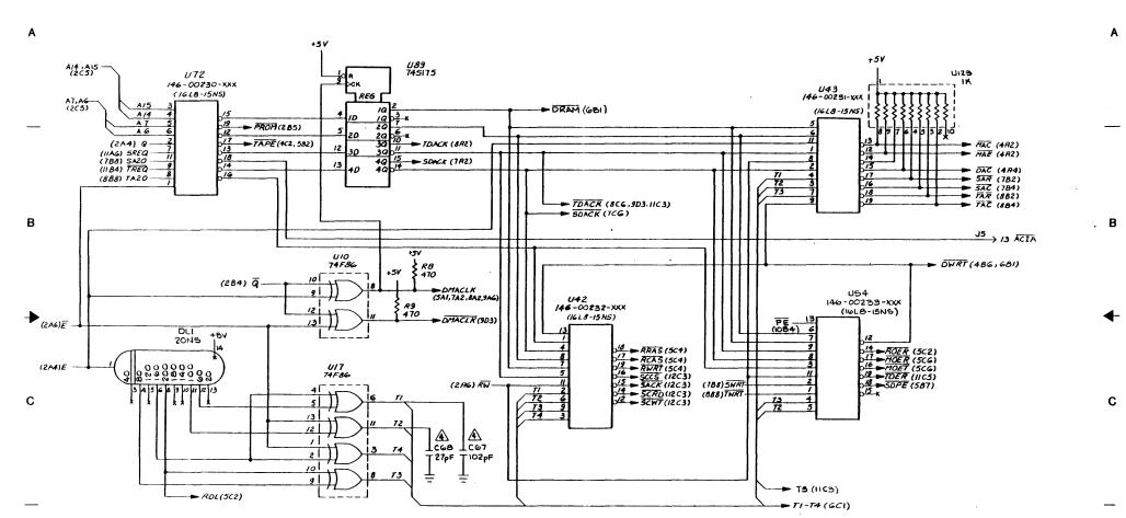
D SCSI Tape Controller Type 9424 Schematic Diagram 1 2 1 з 5 6 7 8 4
