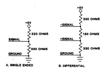
Figure 1-1. Interface Termination Configurations
