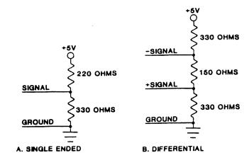
Figure 1-1. Interface Termination Configurations
