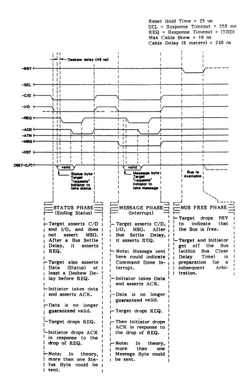
Figure 1-5. SCSI Timing Diagram, Status, Message, and Bus Free Phases
