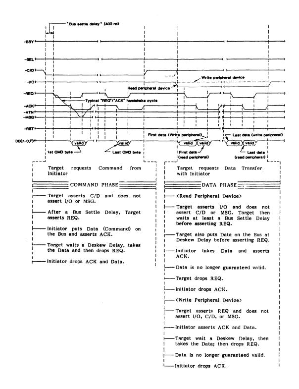
Figure 1-4. SCSI Timing Diagram, Command, and Data Phases
