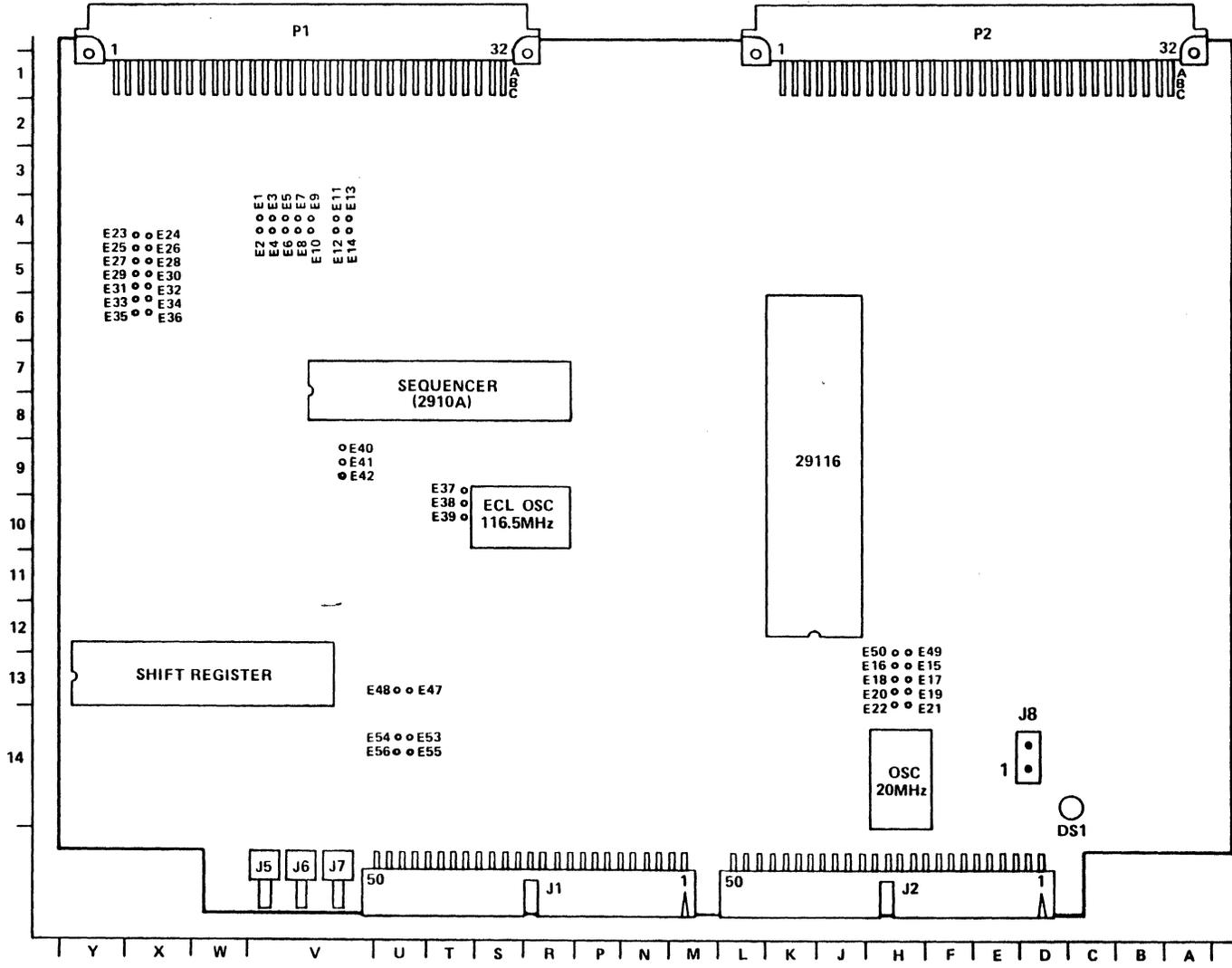
Figure 3-2. Display Controller Board (Rev. D and later)
