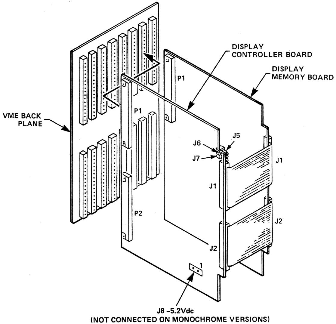
Figure 2-1. VME-Graphics Subsystem Connectors
