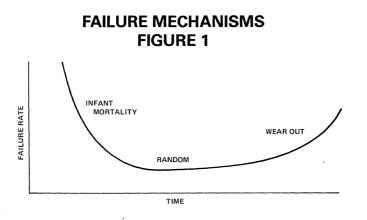
The above curve represents the typical failure rate pattern which can be expected from any group of devices under test. It shows three major regions which concern the reliability engineer; infant mortality, random failures and wear out.
