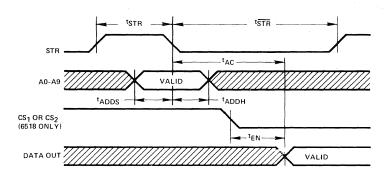
The IM6508 output is active when STR is low. The IM6518 output data latch retains the data when STR returns high.
