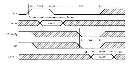
The IM6508 performs a write operation when STR = WE = 0. The IM6518 performs a varie operation when STR =  $CS_1$ =  $CS_2$  = WE = 0. The write operation is terminated on any positive edge from STR or  $CS_1$  or  $CS_2$  or WE.
