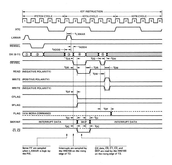
All PIE timing is generated from IM6100 signals LXMAR, DEVSEL, and XTC. No additional timing signals, clocks, or one shots are required. Propagation delays, pulse width, data setup and hold times are specified for direct interfacing with the IM6100.
