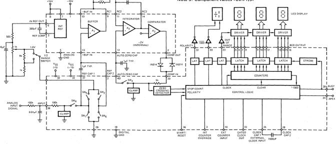
FIGURE 1.3½ DIGIT A/D CONVERTER FUNCTIONAL DIAGRAM
