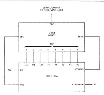
FIGURE 5. SIMPLE 7103/7103A TO UART INTERFACE
