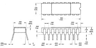
NOTE: Board drilling dimensions will equal standard practice for .020 diameter lead.
