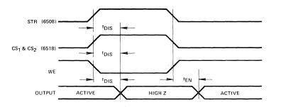
The IM6508 output is high impedance when STR = 1 or WE = 0. The IM6518 output is high impedance when  $CS_1$  or  $CS_2 = 1$  or WE = 0.
