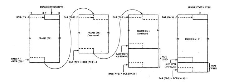
Figure 4-6. Receive DMA Buffer Chaining
