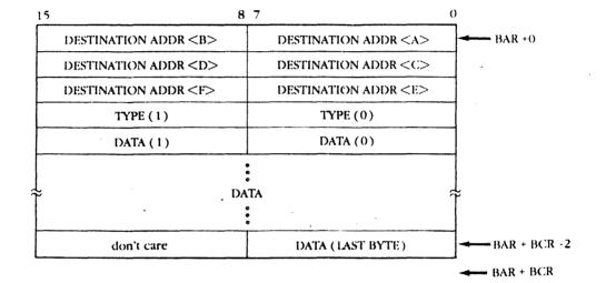
Figure 3-12. Transmit Data Format (source address insertion)
