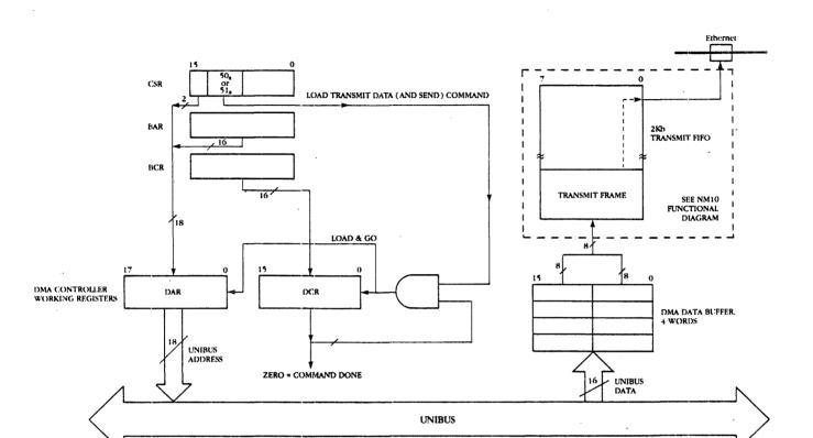
Figure 4-4. Functional Diagram of NI1010A Transmit DMA Operation
