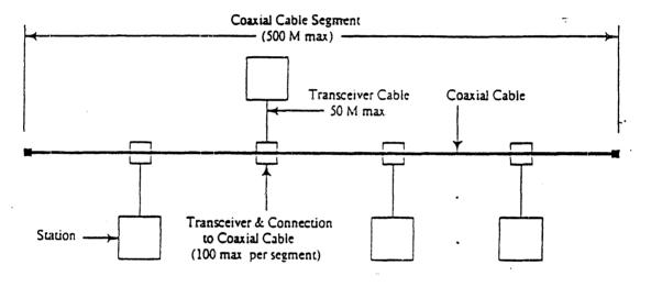
Figure A-1a: The Minimal Configuration
