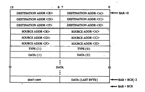
Figure 3-12a. Transmit Data Format (no source address insertion)
