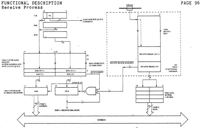
Figure 4-5. Functional Diagram of NI1010A Receive DMA Operation
