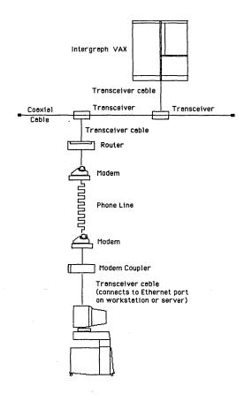
Figure 6-1. An Intergraph Workstation Connected to a Remote Ethernet Network
