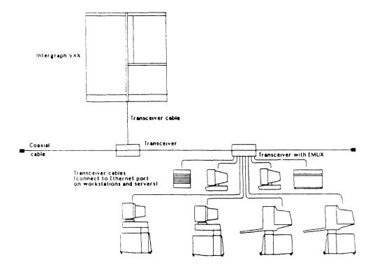
Figure 6-2. Intergraph Workstations and Servers Connected to an EMUX
