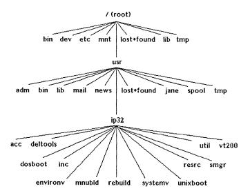
Figure 4-1. System V's Hierarchical Structure
