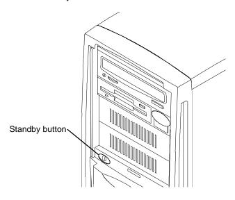
Although the Standby button affects system power management, it is not an "on or off" power switch in the traditional sense. The Standby button is a momentary contact switch, changing system states based upon the length of time the button is pressed. Depending on the operating system running and the system's current power state, you can use the Standby button to start, suspend, wake up, or power down the system.
