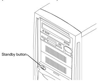
Although the Standby button affects system power management, it is not an "on or off" power switch in the traditional sense. The Standby button is a momentary contact switch, changing system states based upon the length of time the button is pressed. Depending on which operating system is loaded and what the system's current power state is, you can use the Standby button to start, suspend, wake up, or power down the system.
