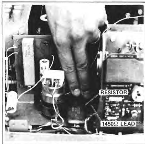
Figure A-2. Current Source Resistor
