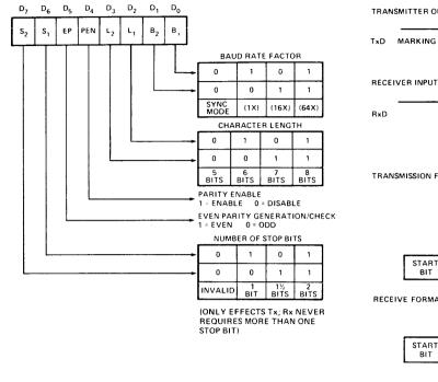
Figure 3-4. USART Asynchronous Mode **Instruction Word Format**
