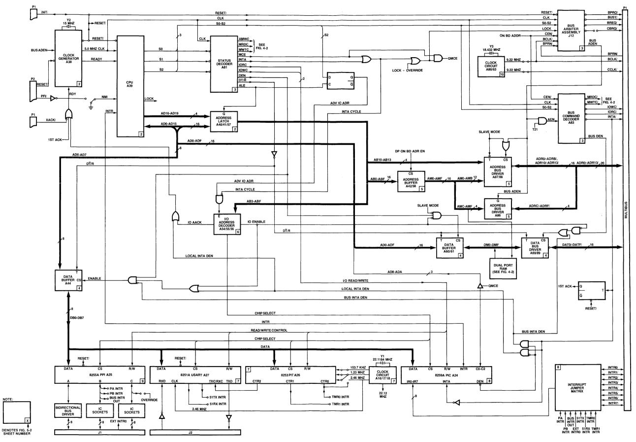
Figure 4-1. iSBC 86/1X Input/Output and Interrupt Simplified Logic Diagram
