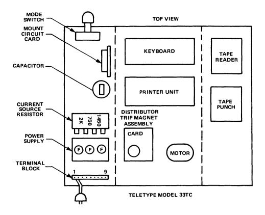
Figure A-1. Teletype Component Layout
