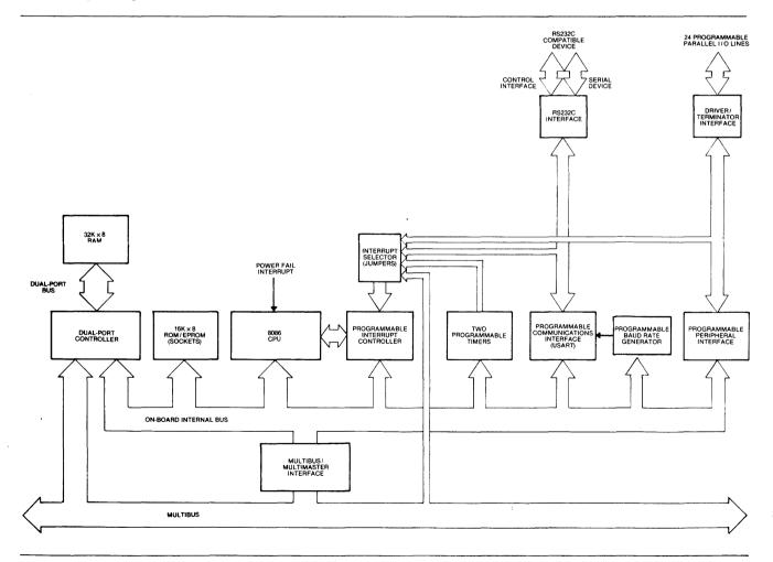
Figure 1. iSBC 86/12 Single Board Computer Block Design
