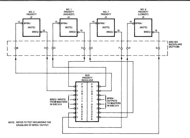
Figure 2-6. Parallel Priority Resolution Scheme
