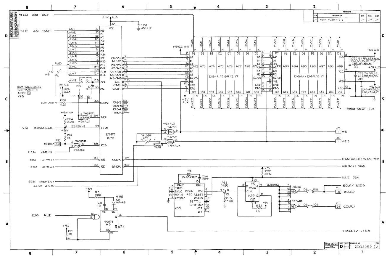
Figure 5-2. iSBC 86/12 Schematic Diagram (Sheet 10 of 11)
