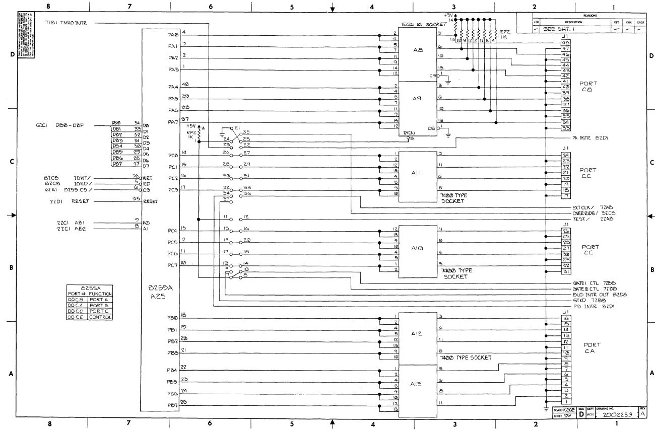
Figure 5-2. iSBC 86/12 Schematic Diagram (Sheet 9 of 11)
