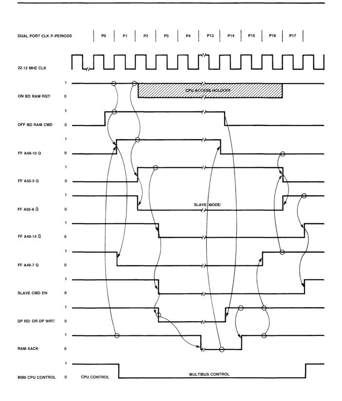
Figure 4-7. Dual Port Control Multibus Access Timing With CPU Lockout
