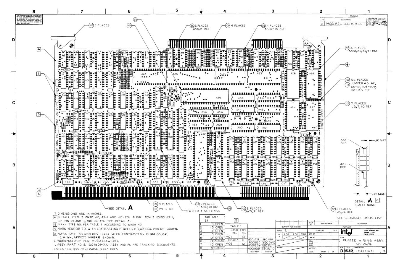
Figure 5-1. iSBC 86/12 Parts Location Diagram
