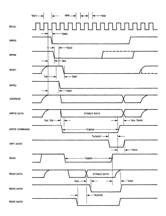
Figure 2-3. Bus Exchange Timing (Master Mode)
