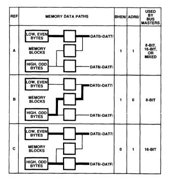
Figure 3-1. Dual Port RAM Addressing (Multibus Access)
