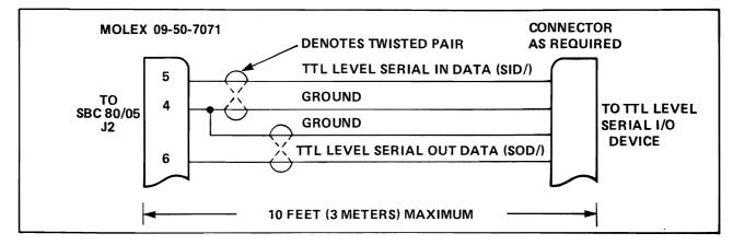
Figure 2-8. TTL Level Serial I/O Device Interface Cabling
