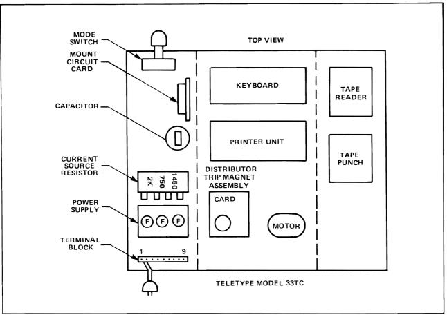
Figure A-1. Teletype Component Layout
