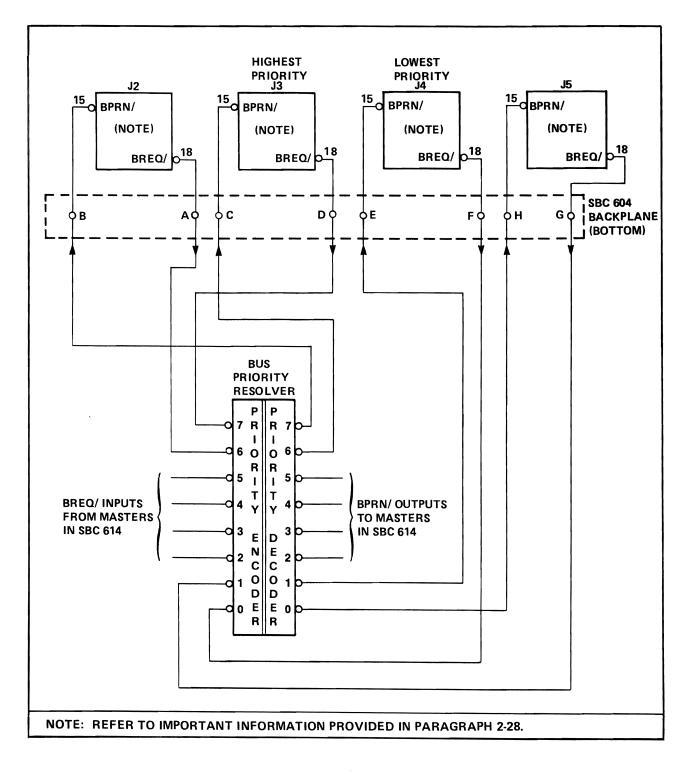
Figure 2-6. Parallel Priority Resolution Scheme
