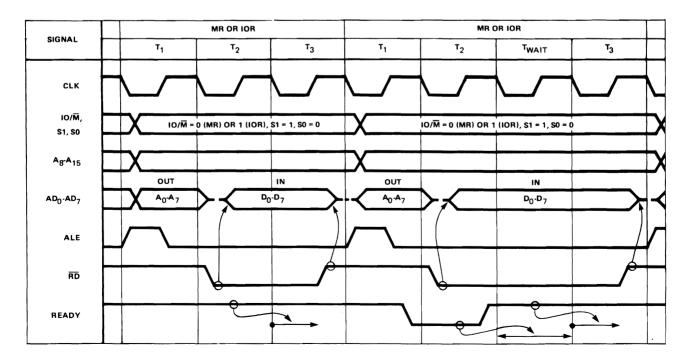
Figure 4-5. Memory Read (or I/O Read) Machine Cycles
