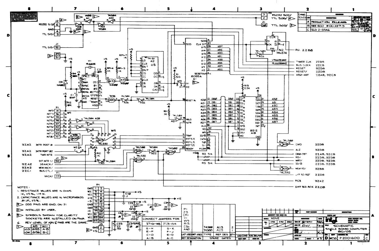
Figure 5-2. SBC 80/05 Schematic Diagram (Sheet 1 of 3)
