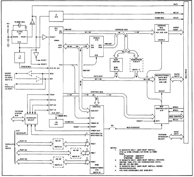
Figure 4-1. SBC 80/05 Block Diagram
