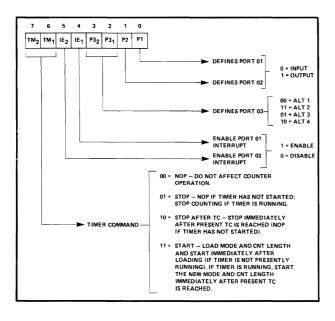
Figure 3-1. Command Register Format (Port 00)
