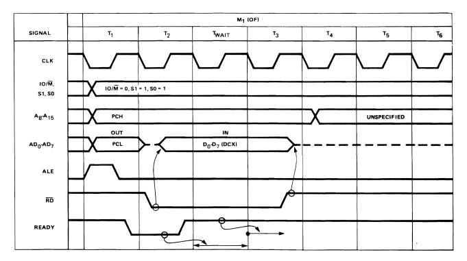
Figure 4-4. Opcode Fetch Machine Cycle (With Wait)
