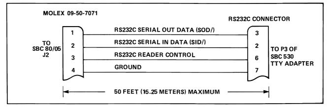
Figure 2-7. RS232C Serial I/O Device Interface Cabling
