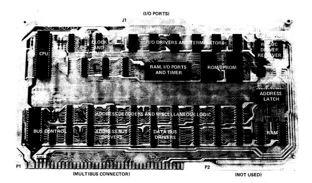
Figure 1-1. SBC 80/05 Single Board Computer
