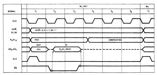
Figure 4-3. Opcode Fetch Machine Cycle
