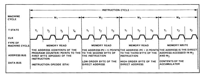
Figure 4-2. Typical CPU Instruction Cycle
