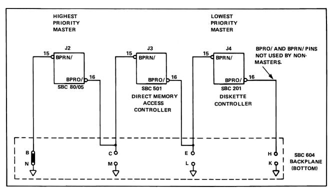
Figure 2-5. Serial Priority Resolution Scheme
