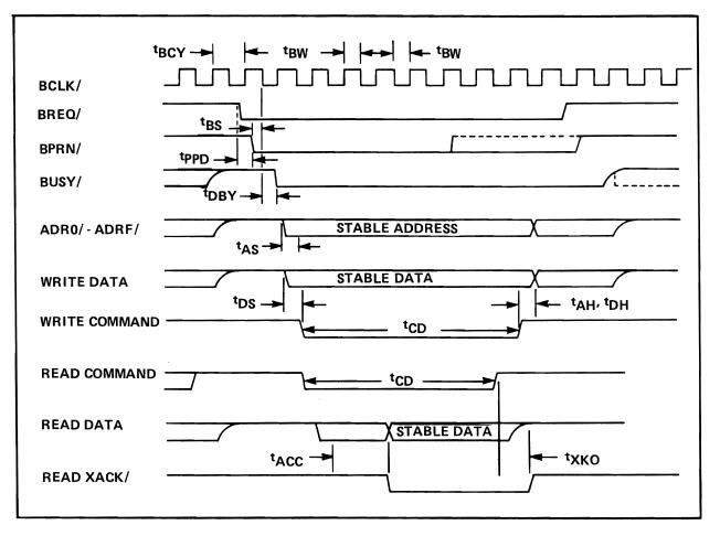
Figure 2-3. SBC 80/05 Bus Exchange Timing
