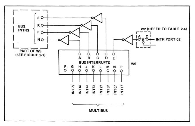
Figure 2-2. Multibus Interrupt Jumpers
