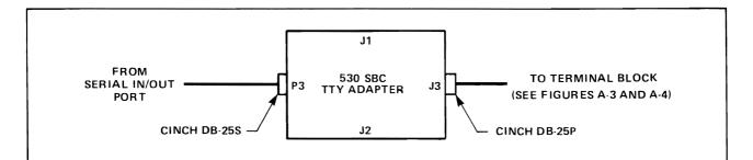
Figure A-8. TTY Adapter Cabling
