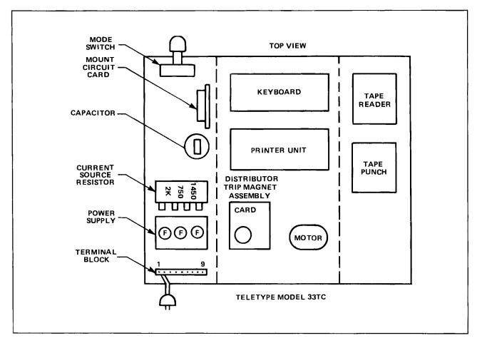
Figure H-1. Teletype Component Layout
