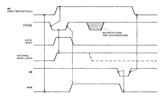
FIGURE 3-20 8255 MODE 1 INPUT TIMING
