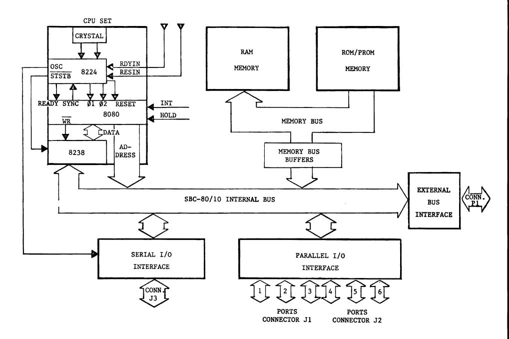
FIGURE 3-1 SBC 80/10 FUNCTIONAL BLOCK DIAGRAM
