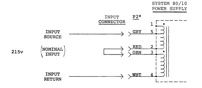
\*Wire from transformer Tl, Pin 1 is moved to Tl, Pin 5.
