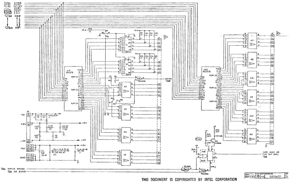
FIGURE B-2. SBC 80/10 SCHEMATIC (5 of 5)
