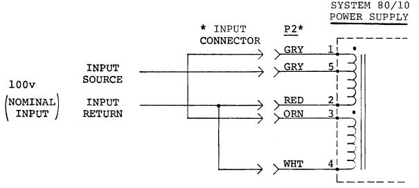
\*5 pin connectors must be used. Use Molex P/N 03-09-2052 for P2 transformer connector and use Molex P/N 03-09-1052 as mating connector.
