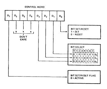
FIGURE 3-16 BIT SET/RESET CONTROL WORD FORMAT
