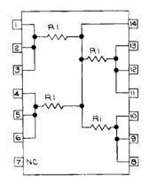
RESISTOR NETWORK SPECIFICATIONS: RESISTANCE VALUES: ±2% (MAX) OPERATING TEMPERATURE: 0°C TO +70°C TEMPERATURE COEFFICIENT: ± 200 PPM / °C OVER TEMPERATURE RANGE OF O°C TO +70°C OPERATING YOLTAGE: 6.0 YDC (MAX) POWER RATING: AT 70°C, 0.7 YVATT PER PACK TRACKING RESISTANCE RATIO: ± 1.0% (MAX) STABILITY: 1 1% YEAR (MAX) LOAD LIFE: 1% (AR) OVER 1000 HOURS PACKAGES DUAL IN LINE - CERAMIC OR PLASTIC NOTES: UNLESS OTHERWISE SPECIFIED,
