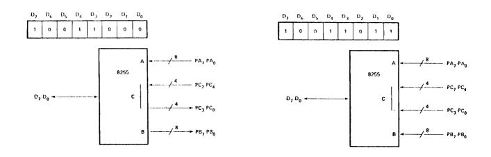
FIGURE 3-18 EXAMPLES OF MODE 0 CONFIGURATION
