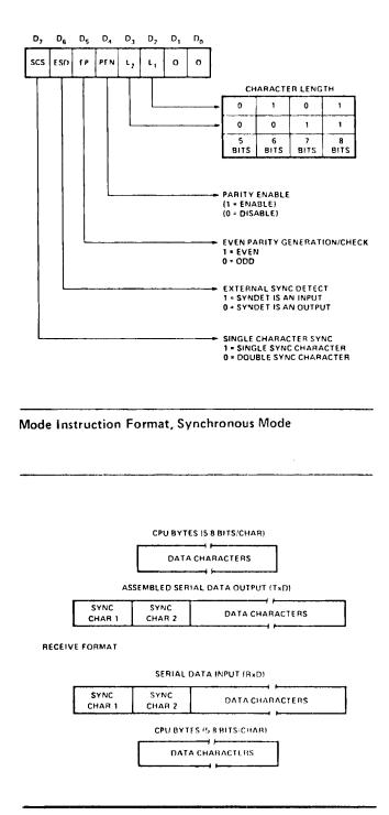
Synchronous Mode, Transmission Format
