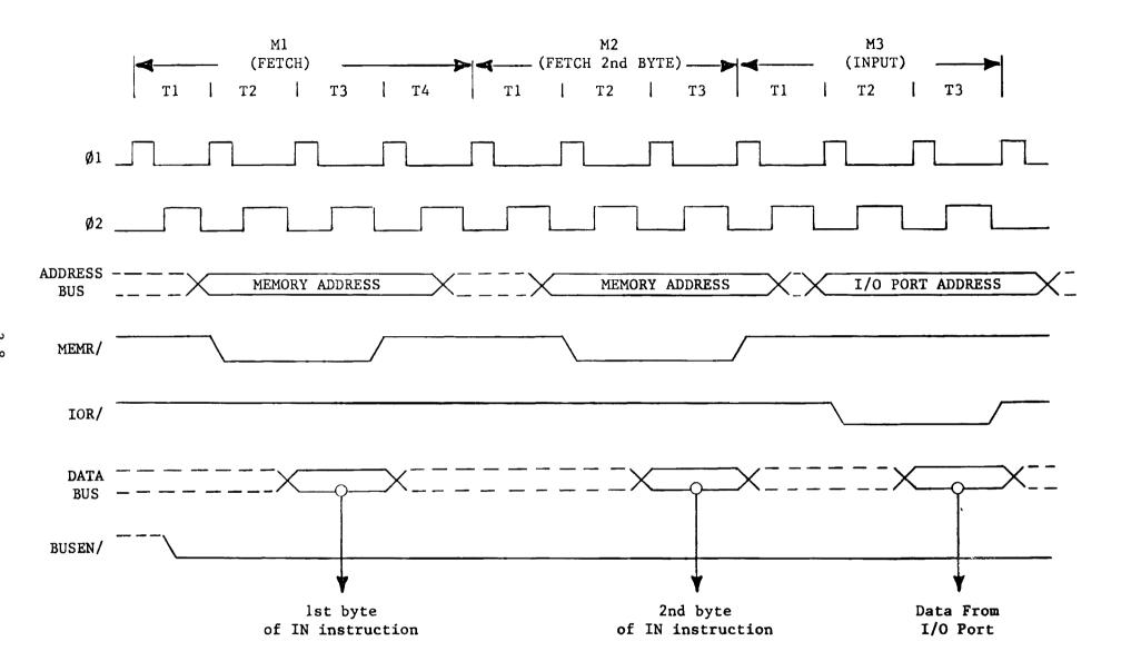
FIGURE 3-3 TYPICAL FETCH MACHINE CYCLE
