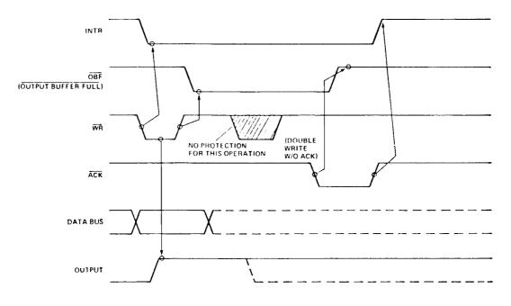
FIGURE 3-22 MODE 1 BASIC OUTPUT TIMING
