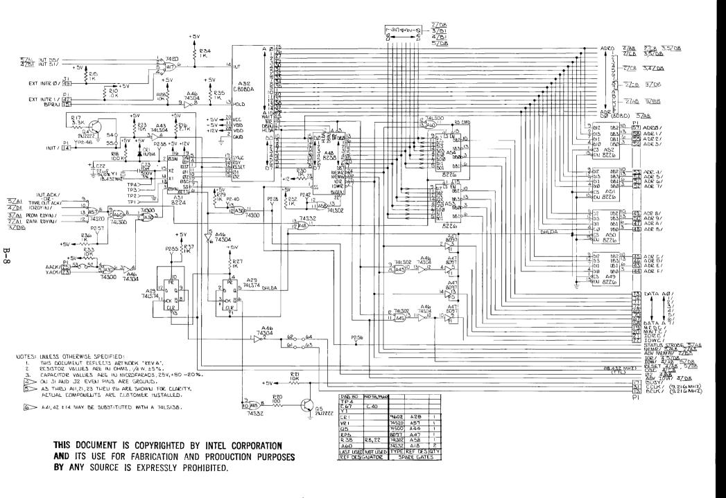
FIGURE B-3. SBC 80/10A SCHEMATIC (SHEET 1 of 5)
