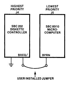
Figure 9-1. Serial Priority Configuration with SBC 80/10 and another Multibus Master
