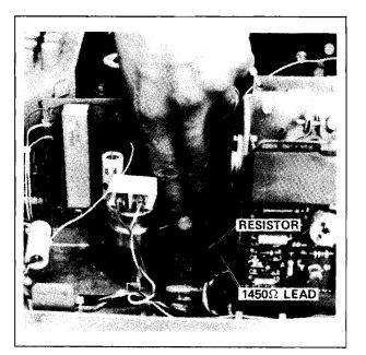
Figure H-2. Current Source Resistor
