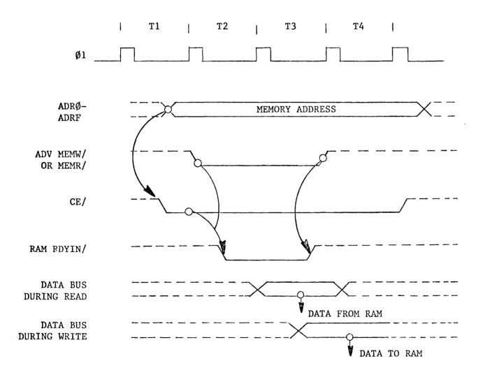
FIGURE 3-7 RAM ACCESS TIMING
