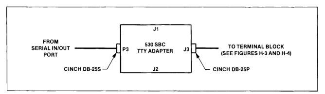
Figure H-8. TTY Adapter Cabling
