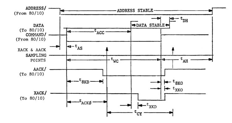
\* FIGURE A-1. MEMORY AND I/O READ TIMING (CONTINUOUS BUS CONTROL)
