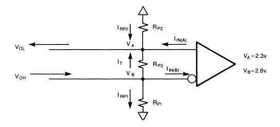
Figure B-3. Case 2 Configuration Example
