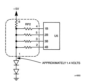
Figure 2-10. RP2 Configurations for RS442A/449 and RS232C
