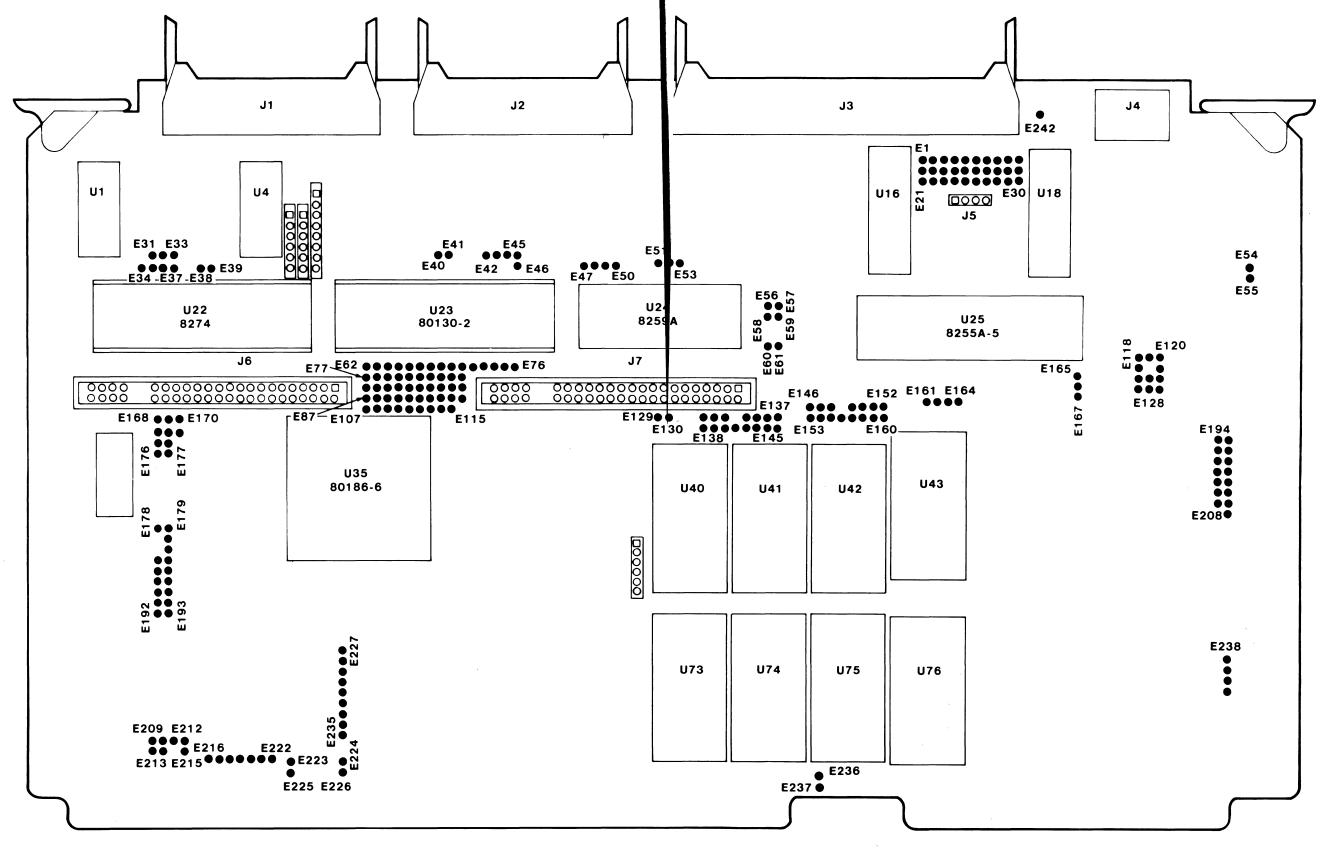
Figure A-1. Jumper Post Location Diagram
