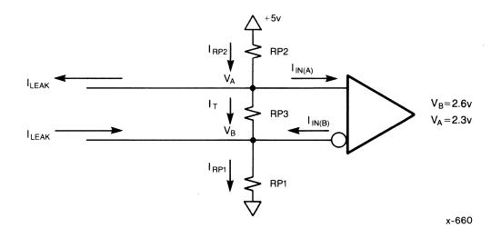
Figure B-2. Case 1 Example Configuration
