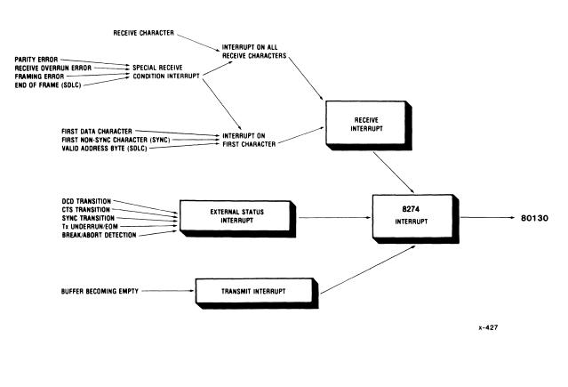
Figure 4-6. Interrupt Structure
