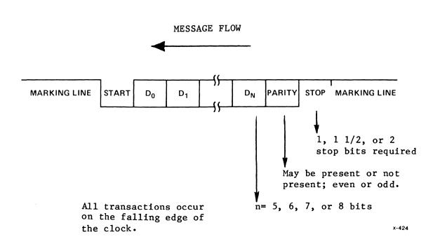
Figure 4-3. Asynchronous Message Format
