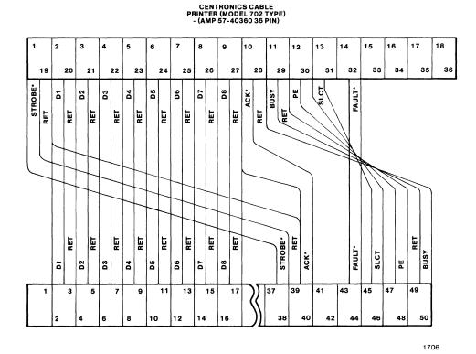
Figure C-8. Cable Fabrication Diagram
