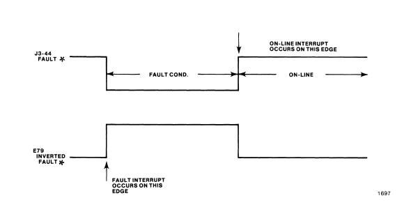
Figure C-9. FAULT\* Timing Specification
