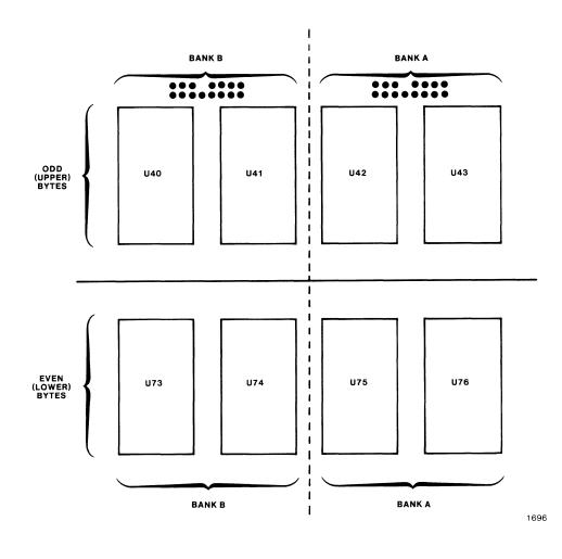
Figure 2-3. Local Memory Socket Pairs and Jumper Matrices
