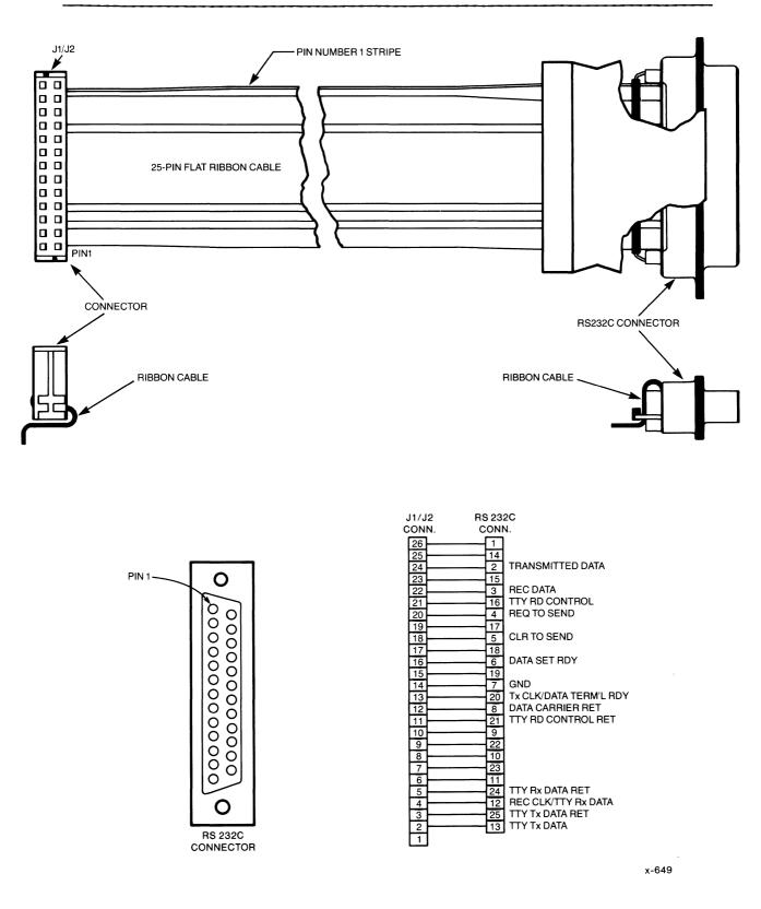
Figure 2-8. RS232C Cable Diagram for Connector J1
