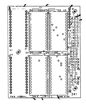
Figure E-2. Parts Location Diagram
