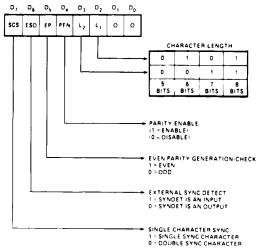
Figure 3-4. PCI Synchronous Mode Instruction Word Format
