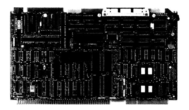
Figure 1-2. iSBC $^{\otimes}$  86/05 Board With Optional Multimodule Boards
