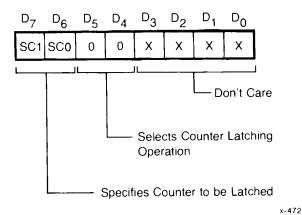
Figure 3-2. PIT Counter Register Latch Control Word Format
