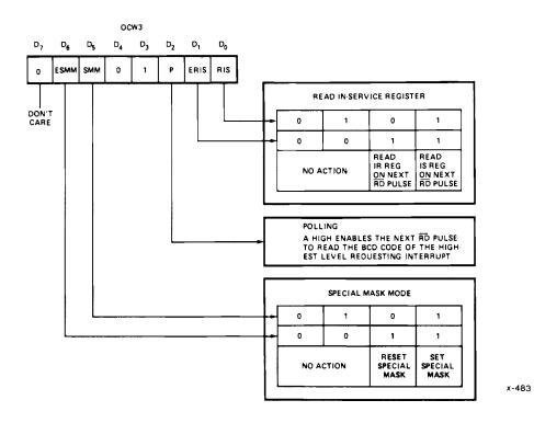
Figure 3-14. PIC Operation Control Word Formats
