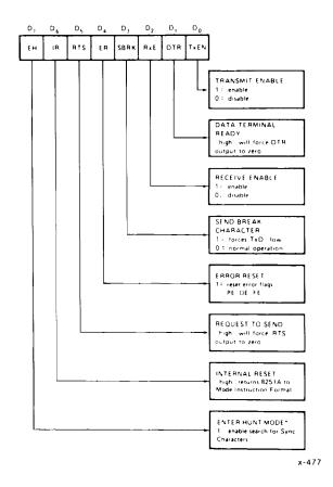
Figure 3-8. PCI Command Instruction Word Format
