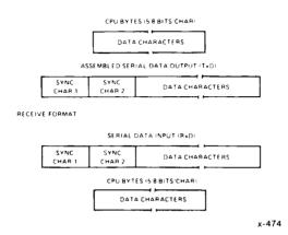
Figure 3-5. PCI Synchronous Mode Transmission Format
