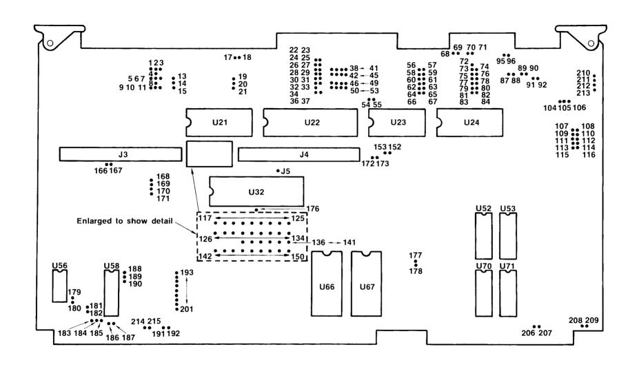
Figure C-1. iSBC® 86/05 Board Jumper Post Location Drawing
