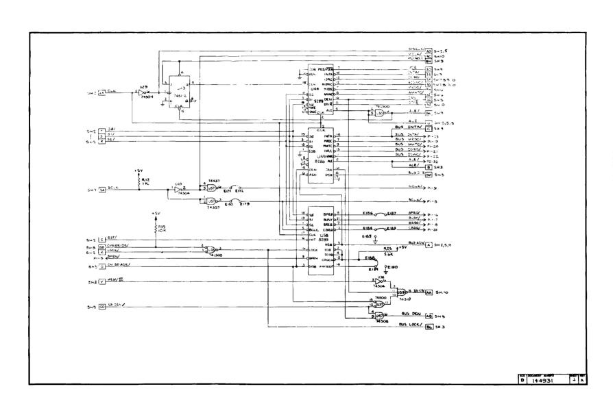
Figure 4iSBC® 86/05 Board Schematic Diagram (Sheet w of. 10)
