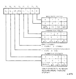
Figure 3-6. PCI Asynchronous Mode Instruction Word Format
