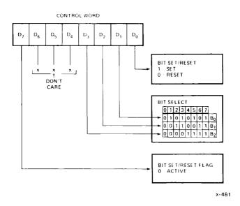
Figure 3-12. PPI Port C Bit Set/ Reset Control Word Format
