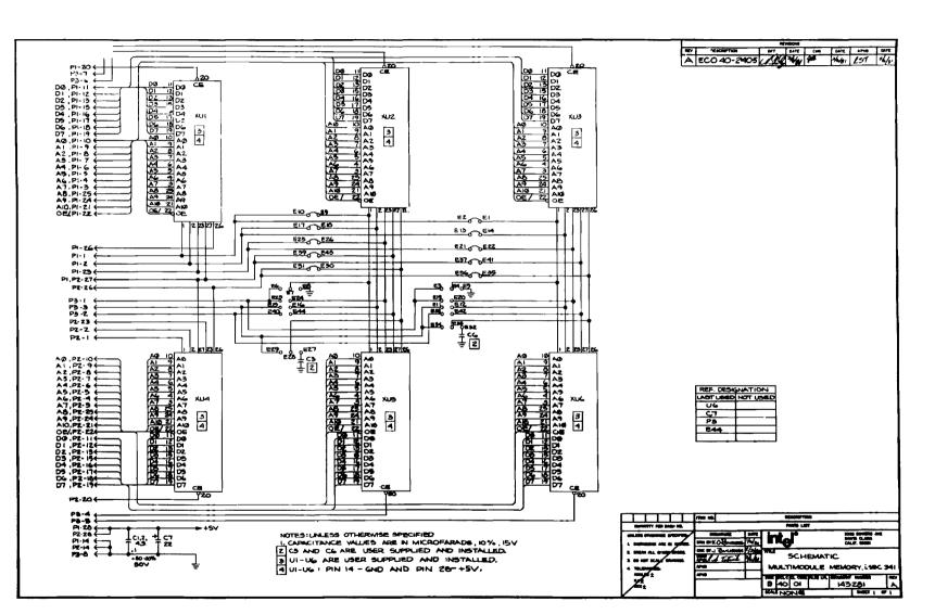
Figure 4iSBC® 341 ROM Expansion Module Schematic Diagram
