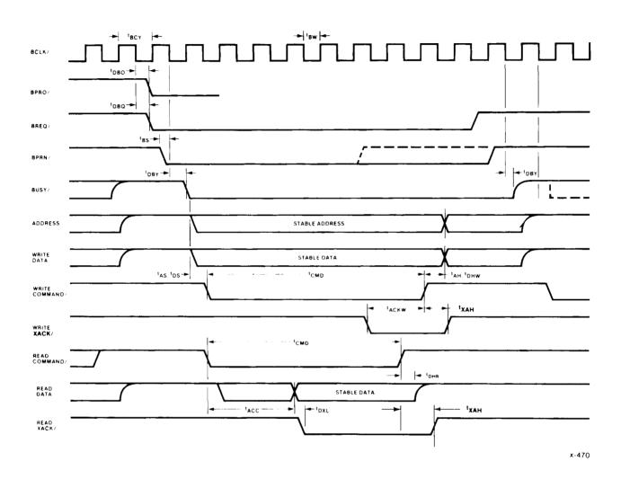
Figure A-1. iSBC® 86/05 AC Timing Diagram
