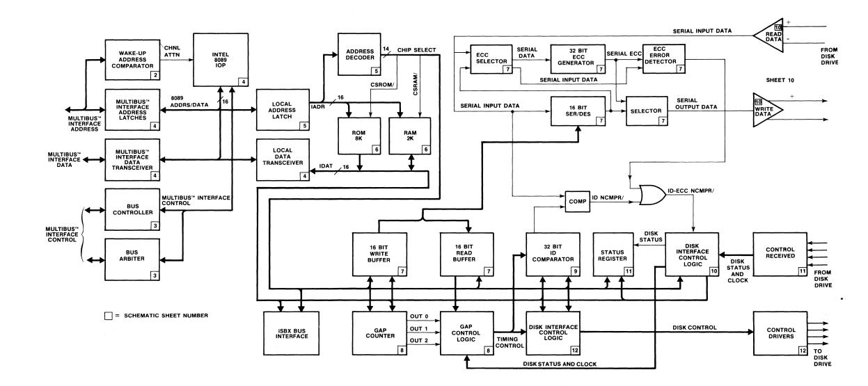
Figure 4-3. iSBC 215<sup>™</sup> Controller Functional Block Diagram
