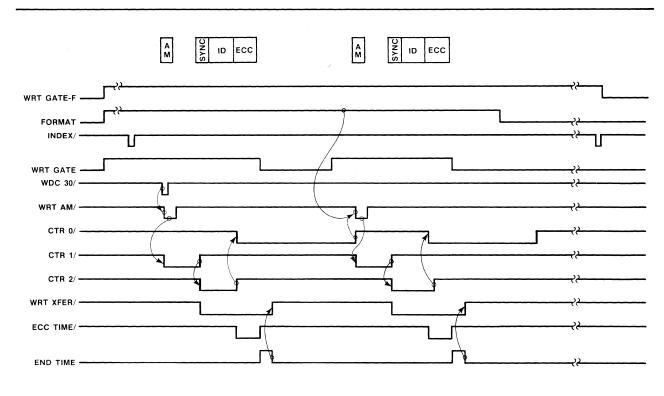
Figure 4-10. Timing Diagram for Disk Formatting Sequence
