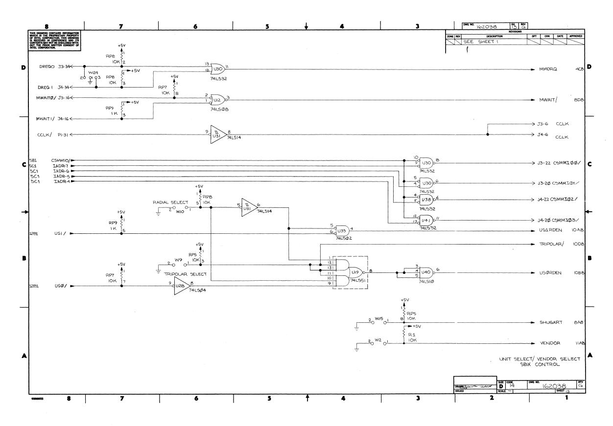
Figure 5-3. iSBC 215<sup>™</sup> Winchester Disk Controller Schematic Diagram (Sheet 13 of 14)
