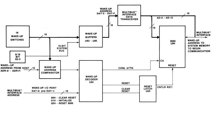
Figure 4-6. Wake-Up Address Logic
