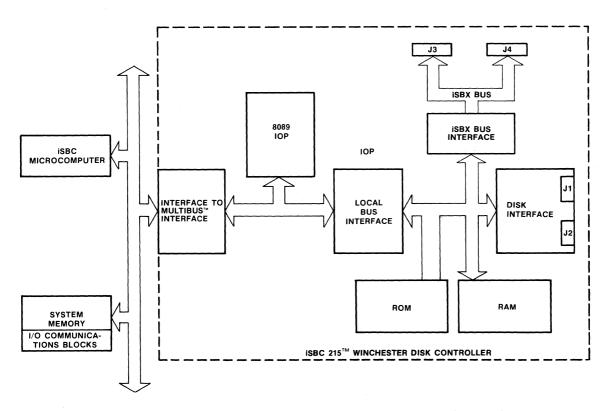
Figure 4-2. Simplified Block Diagram of iSBX 215<sup>™</sup> Controller
