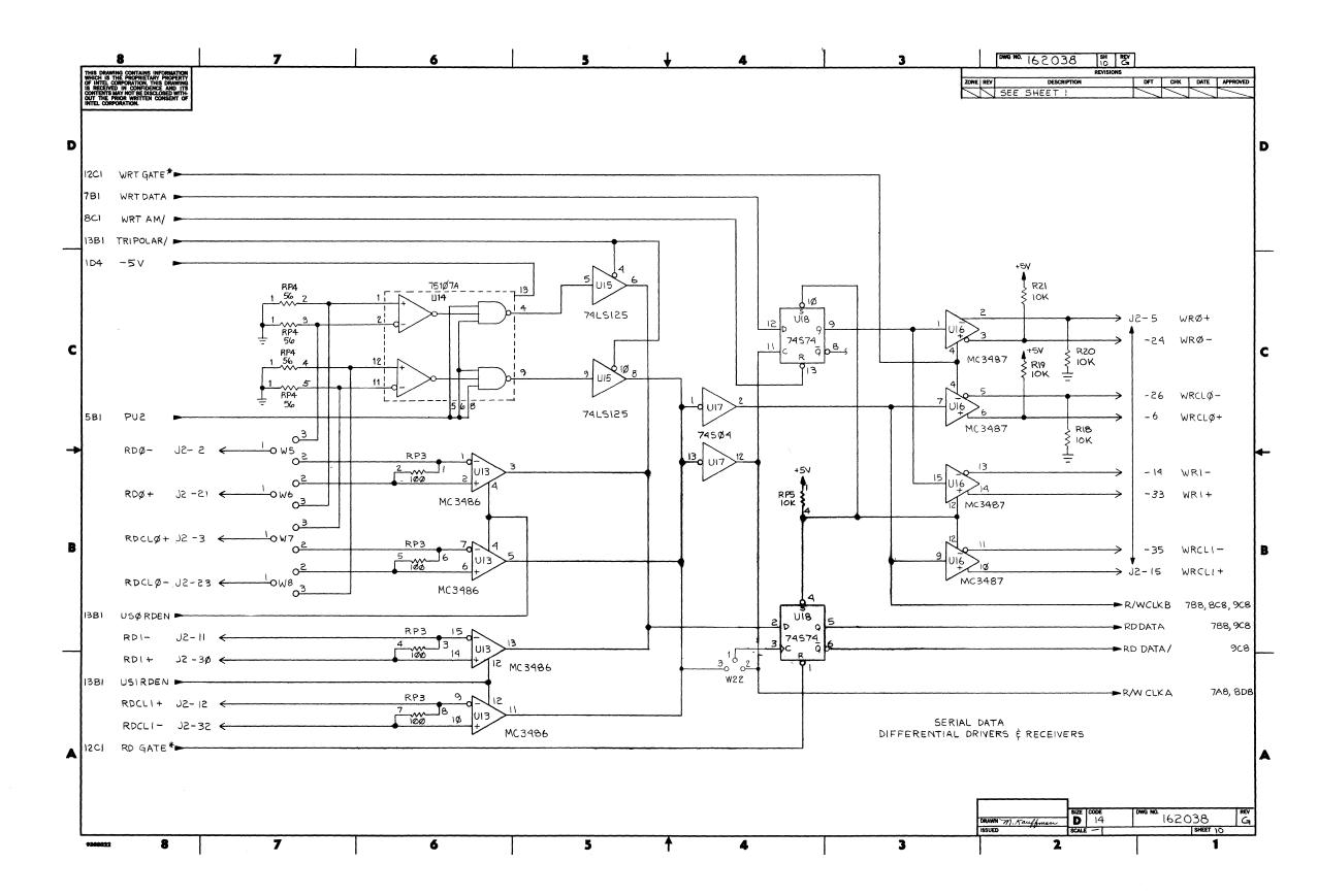
Figure 5-3. iSBC 215<sup>™</sup> Winchester Disk Controller Schematic Diagram (Sheet 10 of 14)
