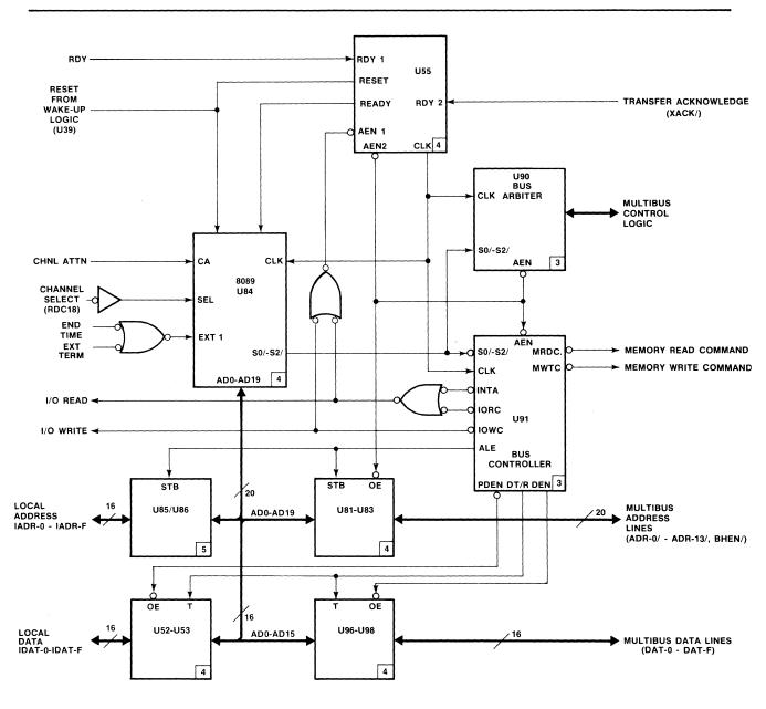
Figure 4-4. Bus Arbiter and Bus Controller Logic
