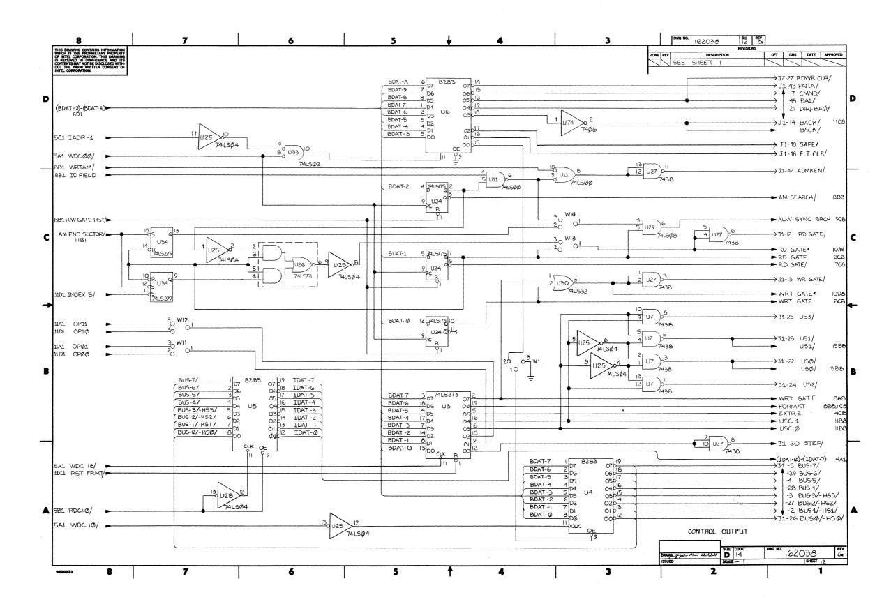
Figure 5-3. iSBC 215<sup>TM</sup> Winchester Disk Controller Schematic Diagram (Sheet 12 of 14)
