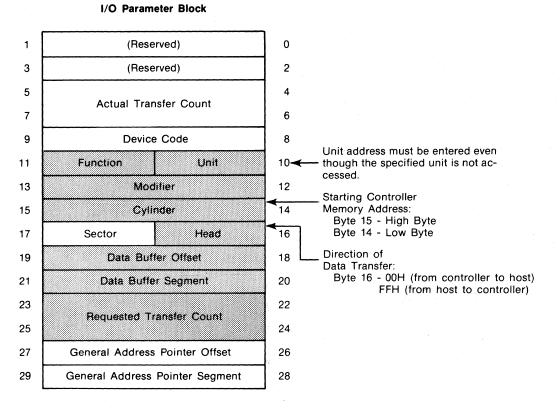
Figure 3-19. Buffer I/O
