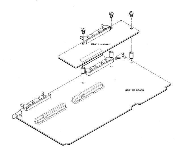
Figure 2-11. Installing the iSBX 218<sup>™</sup> Board on the iSBC 215<sup>™</sup> Controller Board
