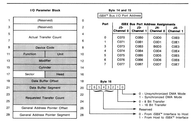
Figure 3-18. I/O Transfers Through iSBX<sup>™</sup> Interface
