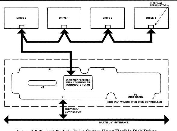
Figure 1-2 Typical Multiple Drive System Using Flexible Disk Drives and iSBX 218<sup>™</sup> Flexible Disk Controller
