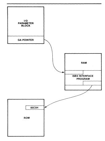
Figure 3-22. Execution of iSBX<sup>™</sup> Bus I/O Program From RAM
