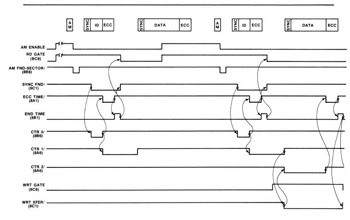
Figure 4-11. Timing Diagram for Write Data
