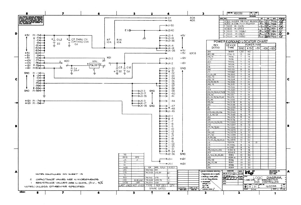
Figure 5-3. iSBC 215<sup>™</sup> Winchester Disk Controller Schematic Diagram (Sheet 1 of 14)
