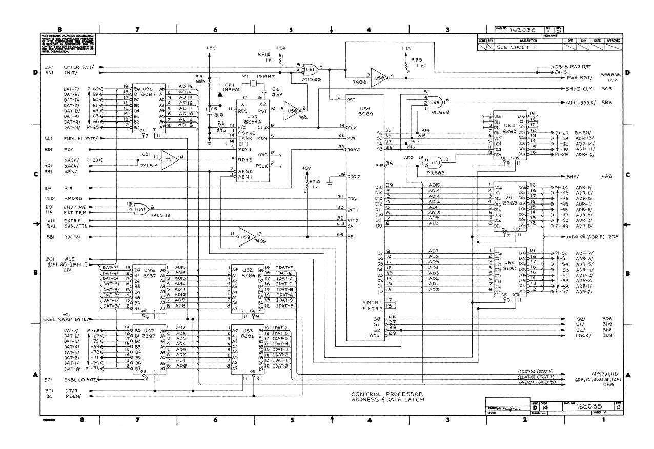
Figure 5-3. iSBC 215<sup>™</sup> Winchester Disk Controller Schematic Diagram (Sheet 4 of 14)
