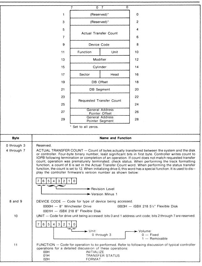
Figure 3-7. I/O Parameter Block Description
