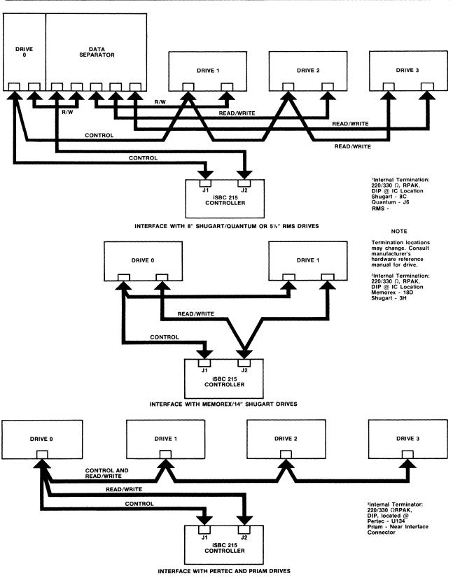
Figure 2-10. Controller to Drive Interfacing
