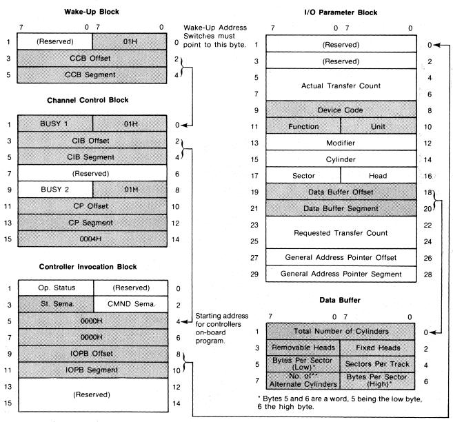
\*\*This byte defines the bit encoding scheme when initializing a flexible disk unit connected to the iSBX 218<sup>TM</sup> controller: 00H for FM (single density) and 01H for MFM (double density). The iSBX 218<sup>TM</sup> controller does not support 128 bytes per sector in the MFM mode.
