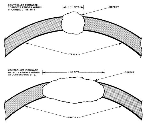
Figure 1-3. Automatic Error Checking and Correction
