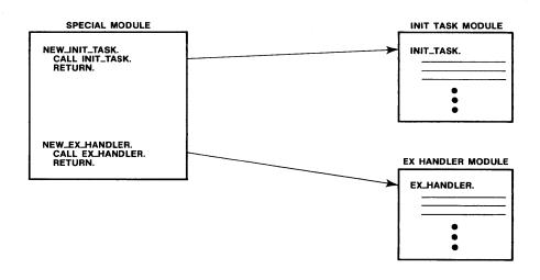
Figure 8-2. Special Module Freezes Entry Points
