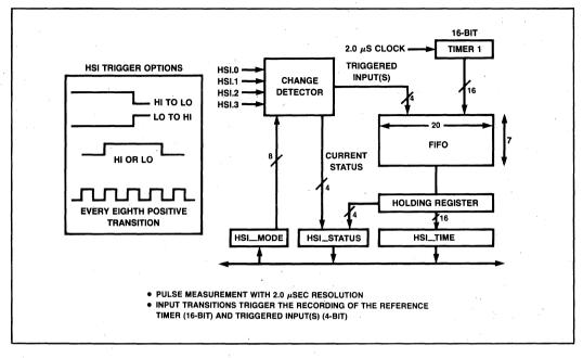
Figure 2-14. High Speed Input Unit
