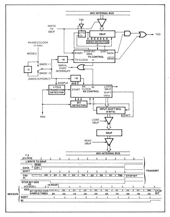
Figure 6-21A. Serial Port Mode 2
