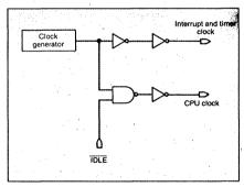
3. The 80C49's low-power idle mode is implemented using dual clocks, allowing the timer-counter and interrupts to remain active while the controller draws just 500  $\mu$ A operating from a 6-V power supply at an 11-MHz clock rate.
