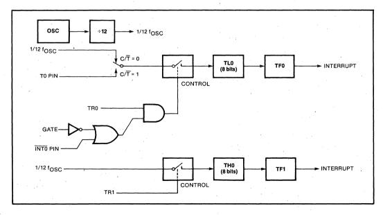
Figure 6-12. Timer/Counter 0 Mode 3: Two 8-bit Counters
