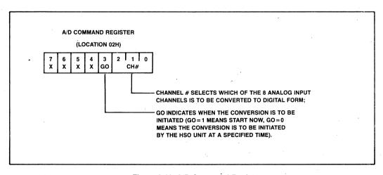
Figure 2-19. A/D Command Register
