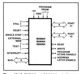
Figure 13-16. 8048AH and 8049AH Logic Symbol
