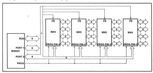
Figure 14-9. Low Cost I/O Expansion
