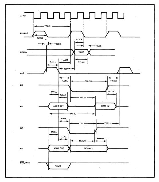
Figure 4-14. Bus Signal Timings
