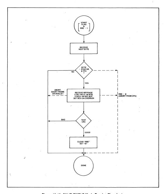
Figure 19-10. SIU FLEXIBLE Mode Receive Flowchart
