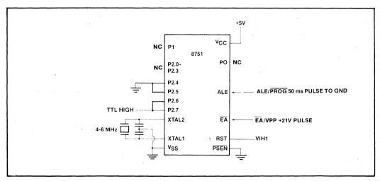
Figure 4. Security Bit Programming Configuration
