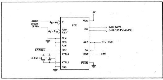
Figure 5. Program Verification Configuration
