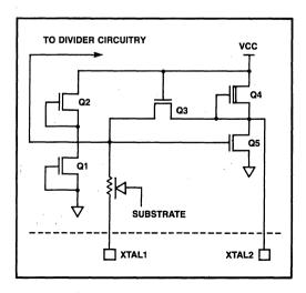
Figure 4-1. 8096 Oscillator Circuit
