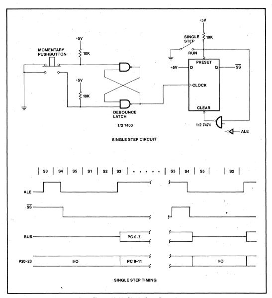
Figure 13-13. Single Step Operation
