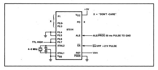
Figure 6-31. Programming the Security Bit in the 8751H
