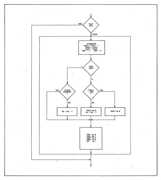
Figure 19-7g. SIU AUTO Mode Receive Flowchart—I Command: Sequence Error Send, Current Received I-Field in Sequence
