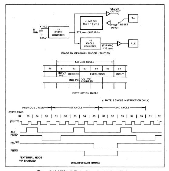
Figure 13-10. MCS®-48 Timing Generation and Cycle Timing
