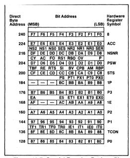
Figure 18-7. Special Function Register Bit Address
