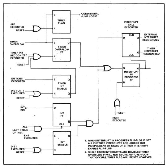
Figure 13-8. Interrupt Logic
