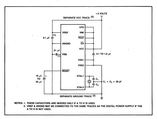
Figure 4-5. Minimum Hardware Connections
