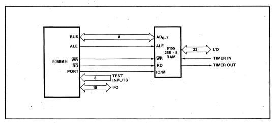
Figure 14-6. 8048AH Interface to 256 x 8 Standard Memories
