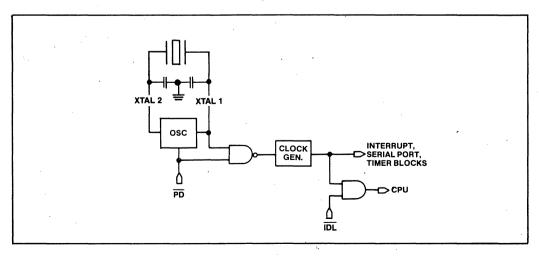
Figure 6-27. Idle and Power Down Hardware
