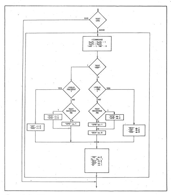
Figure 19-7h. SIU AUTO Mode Receive Flowchart—I Command: Prior Transmitted I-Field Confirmed Sequence Error Receive
