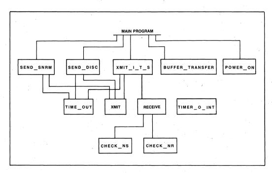
Figure 20.17. Block Diagram of Primary Station Software Structure
