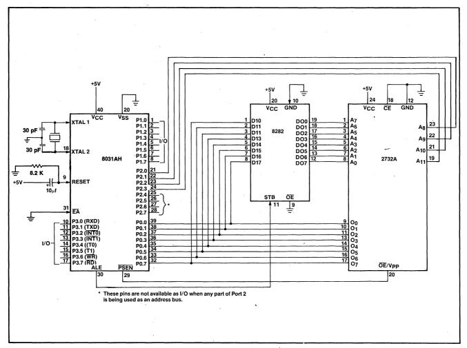
Figure 9-5. External Program Memory Using a 2732
