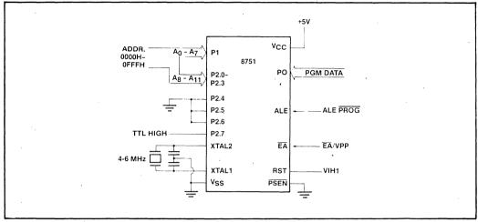
Figure 3. Programming Configuration
