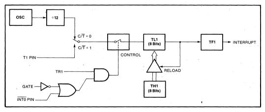
Figure 6-11. Timer/Counter 1 Mode 2: 8-bit Auto-reload
