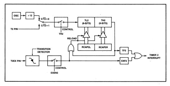
Figure 6-15. Timer 2 in Auto-Reload Mode
