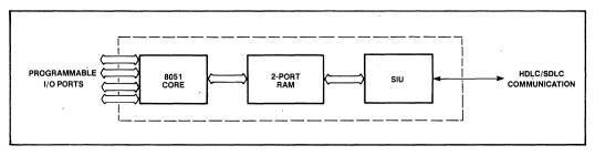
Figure 17-1. RUPI<sup>™</sup>-44 Dual Controller Architecture
