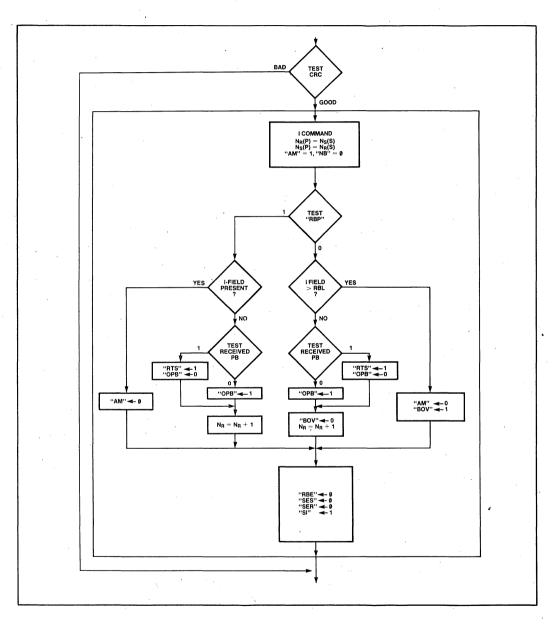
Figure 19-7f. SIU AUTO Mode Receive Flowchart—I Command: Prior Transmitted I-Field Not Confirmed, Current Received I-Field in Sequence
