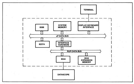
Figure 20-1. Block Diagram of 8088/8044 Interface Test
