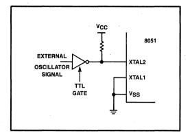
Figure 6-34. Driving the HMOS MCS-51 Parts with an External Clock Source
