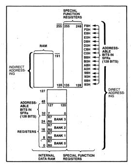
Figure 5. Internal Data Memory Address Space
