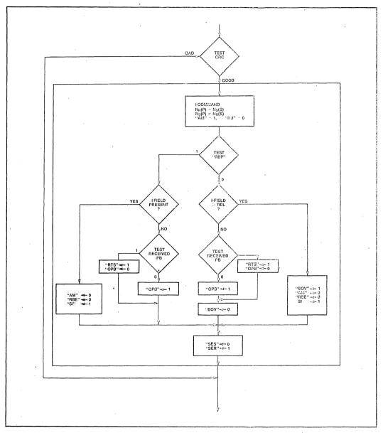
Figure 19-7i. SIU AUTO Mode Receive Flowchart—i Command: Prior Transmitted I-Field Not Confirmed, Sequence Error Receive
