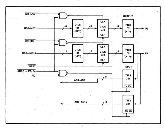
Figure 4-18. I/O Port Reconstruction
