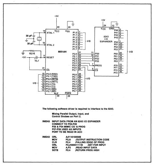
Figure 9-3. I/O Expansion Using an 8243
