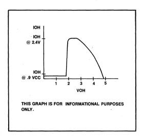
Figure 12-4. CHMOS I/O Current Characteristics
