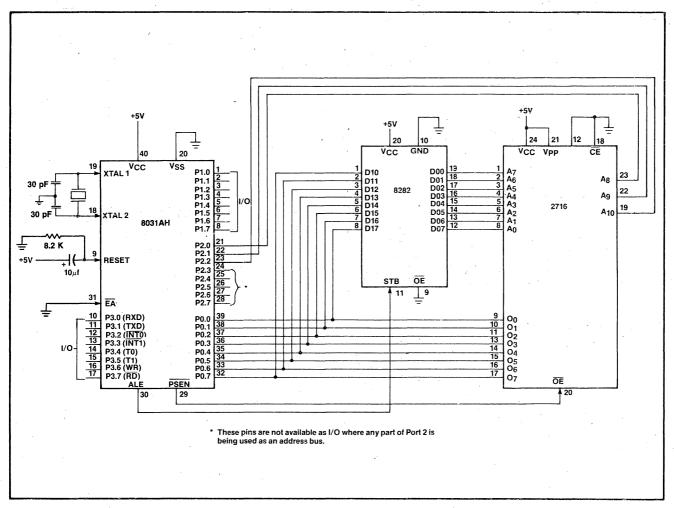
Figure 9-4. External Program Memory Using a 2716
