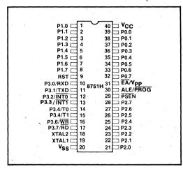
Figure 2. Pin Configuration
