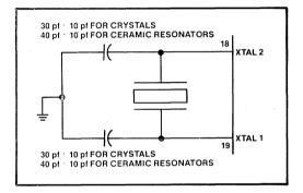
Figure 6-3. Crystal/Ceramic Resonator Oscillator
