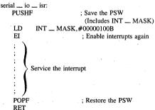
Note that location 200CH in the interrupt vector table would have to be loaded with the value of the label serial \_ io \_ isr and the interrupt be enabled for this routine to execute.
