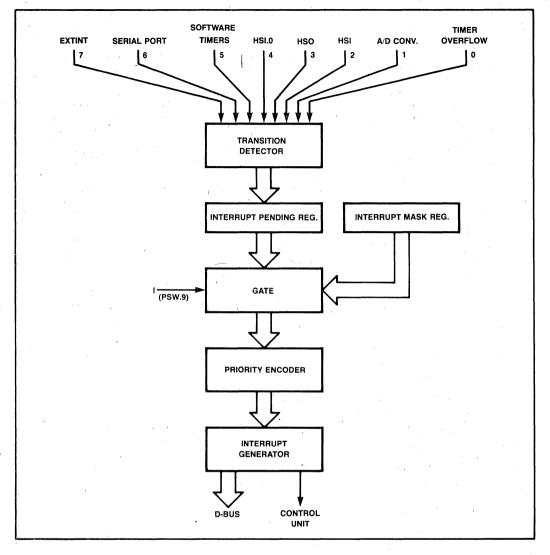
Figure 2-12. Block Diagram of Interrupt System
