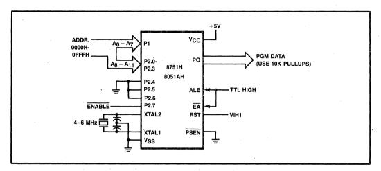
Figure 6-30. Program Verification in the 8751H and 8051AH
