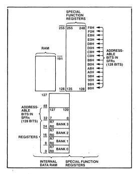
Figure 18-3. Internal Data Memory Address Space
