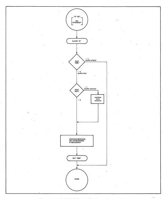
Figure 19-11. FLEXIBLE Mode Response to Receive "SI"
