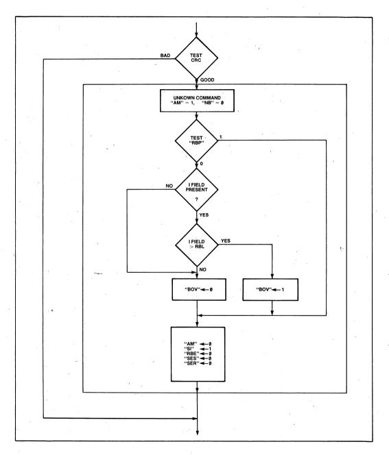
Figure 19-7b. SIU AUTO Mode Receive Flowchart—Unknown Command
