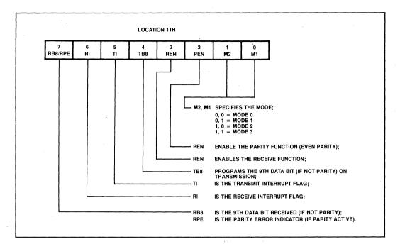
Figure 2-26. Serial Port Control/Status Register
