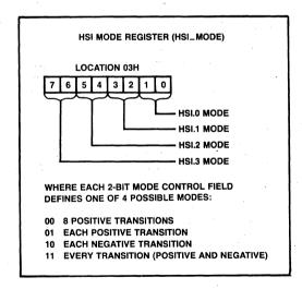
Figure 2-15. HSI Mode Register Diagram
