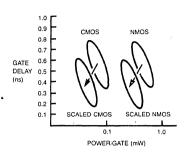
Figure 2: The speed versus power consumption characteristics of NMOS and CMOS technologies. Note the advantages gained by scaling (reducing the size) of the integrated components.
