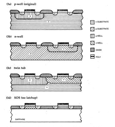
**Figure 3:** Cross sections of transistors formed by each of the four major CMOS processes. Figure 3a is a p-well bulk CMOS transistor; figure 3b shows an n-well bulk device; figure 3c is an example of a twin-tub bulk CMOS transistor; the transistor in figure 3d is formed using silicon-on-sapphire technology.
