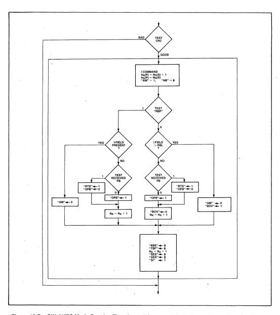
Figure 19-7e. SIU AUTO Mode Receive Flowchart—I Command: Prior Transmitted I-Field Confirmed, Current Received I-Field in Sequence
