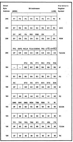
Figure 7-4. Special Function Register Bit Address
