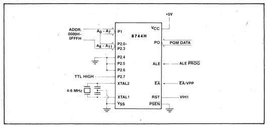
Figure 3. Programming Configuration
