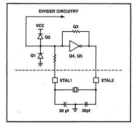
Figure 4-2. Crystal Oscillator Circuit
