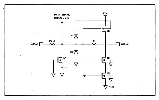
Figure 6-35. On-Chip Oscillator Circuitry in the CHMOS Versions of the MCS-51 Family
