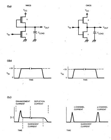
**Figure 1:** A comparison of NMOS and CMOS technologies. Figure 1a shows the schematic diagrams of an inverter as implemented in both NMOS and CMOS. A hypothetical input waveform and the resulting transistor currents are shown in 1b and 1c.
