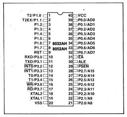
Figure 2. Pin Configuration
