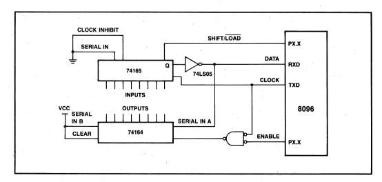
Figure 4-13. Mode 0 Serial Port Example
