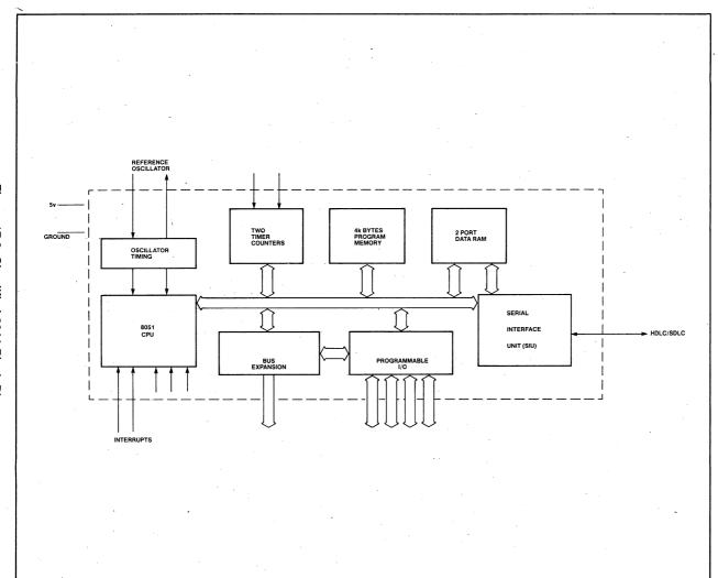
Figure 17-2. Simplified 8044 Block Diagram
