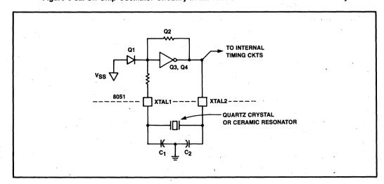
Figure 6-33. Using the HMOS On-Chip Oscillator
