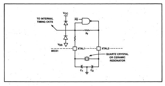
Figure 6-36. Using the CHMOS On-Chip Oscillator
