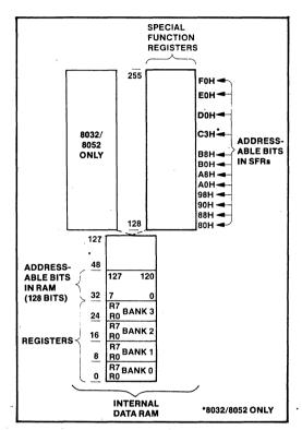
Figure 7-2. Internal Data Memory Address Space
