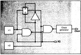
5. The 80C51's power-down mode is activated by a bit in the new on-board PCON register. Setting the register's PD bit turns off the chip's oscillator. This bit actually enables a gate that turns off the oscillator.
