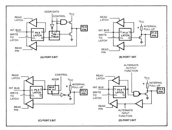
Figure 6-5. 8051 Port Bit Latches and I/O Buffers
