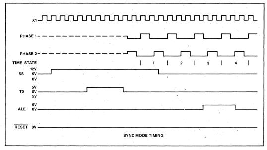
Figure 13-15. Sync Mode Timing
