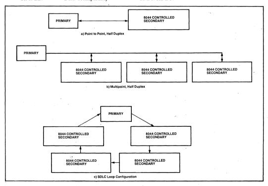
Figure 17-3. RUPI™-44 Supported Network Configurations
