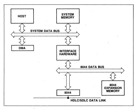
Figure 8. 8044 front end processor
