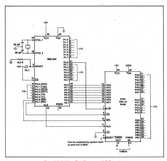
Figure 9-6. Adding a Data Memory and I/O Expander
