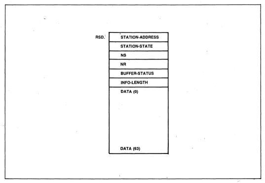
Figure 20-16. Remote Station Database Structure
