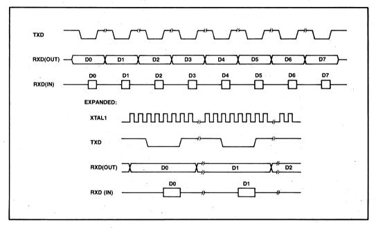
Figure 4-12. Serial Port Timings in Mode 0
