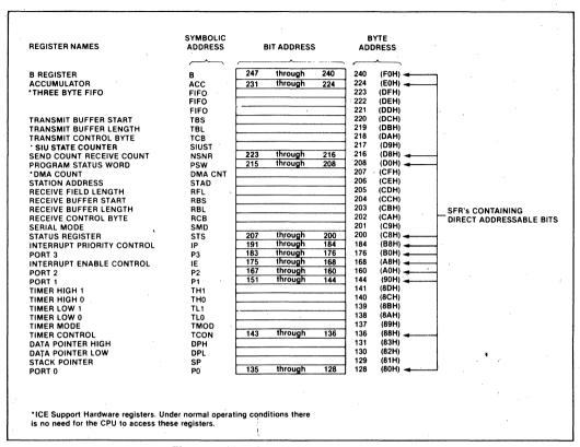
Figure 5. Mapping of Special Function registers
