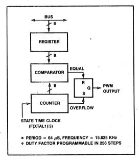
Figure 2-21. Pulse Width Modulated (D/A) Output
