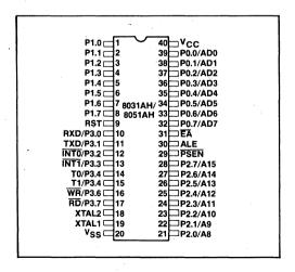
Figure 2. Pin Configuration
