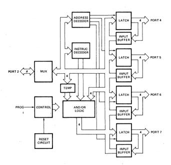
Figure 1. 8243 Block Diagram
