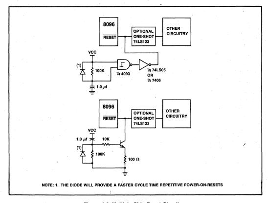
Figure 4-6. Multiple Chip Reset Circuits
