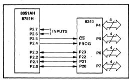
Figure 9-2. Connecting an 8051 with an 8243 I/O Expander
