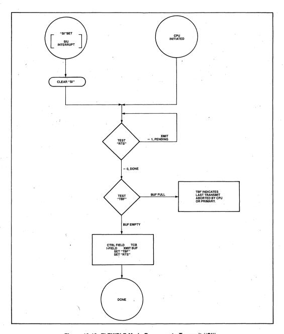
Figure 19-13. FLEXIBLE Mode Response to Transmit "SI"
