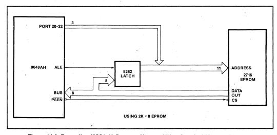
Figure 14-3. Expanding MCS®-48 Program Memory Using Standard Memory Products
