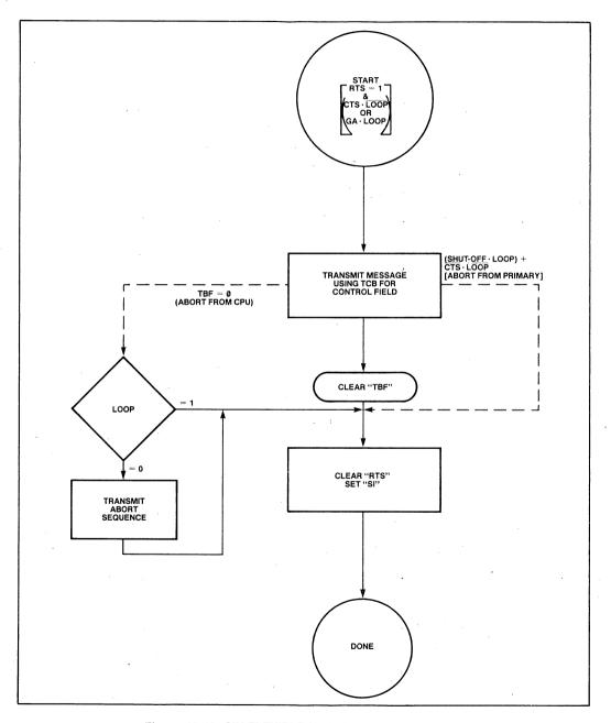
Figure 19-12. SIU FLEXIBLE Mode Transmit Flowchart
