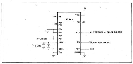
Figure 4. Security Bit Programming Configuration
