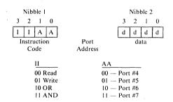
A high to low transition of the PROG line indicates that address is present, while a low to high transition indicates the presence of data. Additional 8243's may be added to the four-bit bus and chip selected using additional output lines from the 8048AH/8748H.
