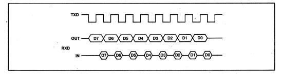
Figure 2-23. Serial Port Mode 0 Timing
