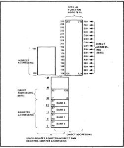
Figure 18-10. Addressing Operands in Internal Data Memory
