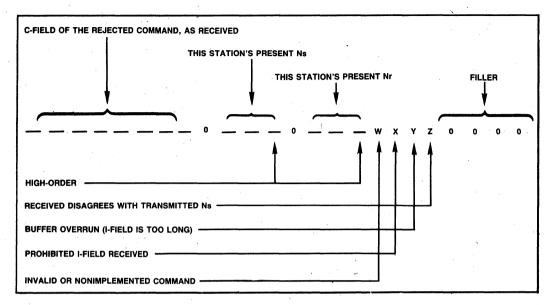
Figure 20.11. Information Field of the FRMR Response, as Transmitted
