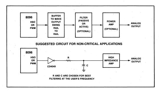
Figure 4-11. D/A Buffer Block Diagram
