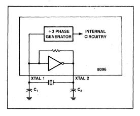
Figure 2-3. Block Diagram of Oscillator
