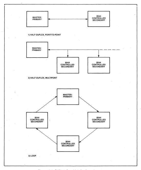
Figure 19-2. RUPI-44 Data Link Configurations
