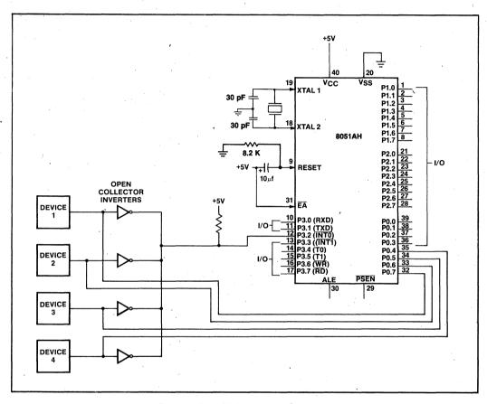
Figure 9-8. Multiple Interrupt Sources
