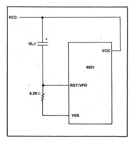
Figure 6-26. Power on Reset Circuit
