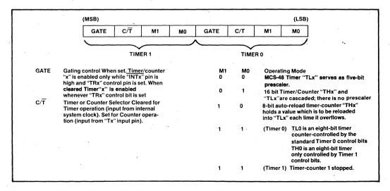
Figure 6-8. TMOD: Timer/Counter Mode Control Register
