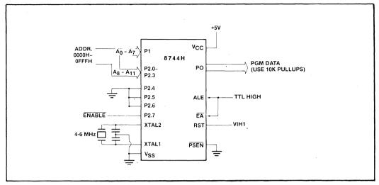
Figure 5. Program Verification Configuration
