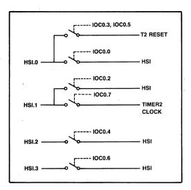
Figure 2-16. IOC0 Control of HSI Pin Functions
