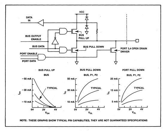
Figure 4-10. Bus and Port 3 and 4 Pins
