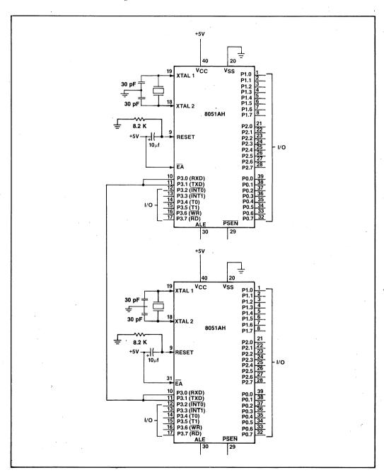
Figure 9-7. Multiple 8051's Using Half-Duplex Serial Communication
