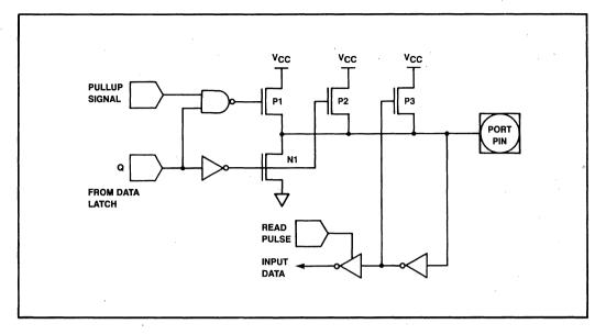
Figure 12-3. CHMOS Quasi-Bidirectional I/O Port Structure
