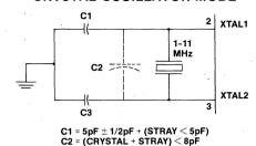
Crystal series resistance should be less than  $30\Omega$  at 11 MHz; less than  $75\Omega$  at 6 MHz; less than  $180\Omega$  at 3.6 MHz.
