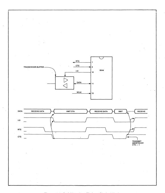
Figure 19-3. Serial Interface Timing—Clocked Mode
