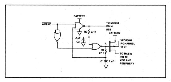
Figure 12-2. MCS®-48 Power Down Circuit
