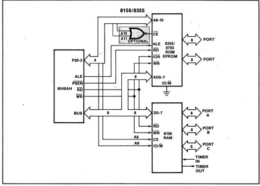
Figure 14-11. The Three-Component MCS®-48 System
