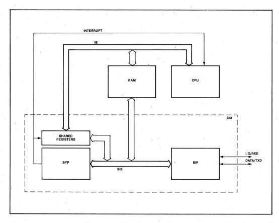
Figure 19-14. The Bit and Byte Processors
