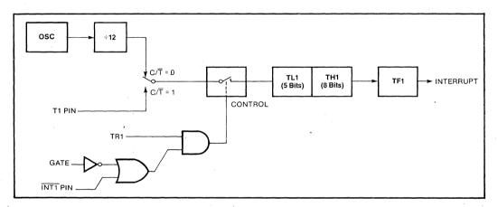
Figure 6-9. Timer/Counter 1 Mode 0: 13-bit Counter
