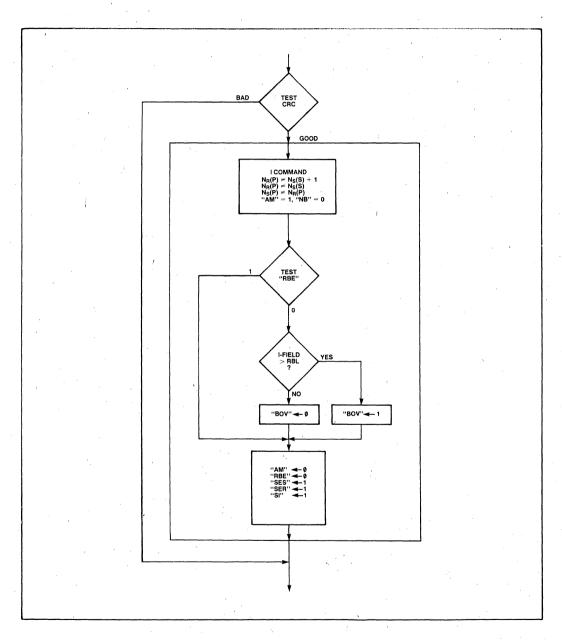
Figure 19-7j. SIU SUTO Mode Receive Flowchart—I Command: Sequence Error Send and Sequence Error Receive
