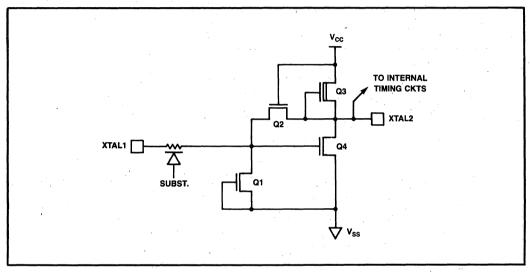
Figure 6-32. On-Chip Oscillator Circuitry in the HMOS Versions of the MCS-51 Family
