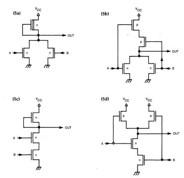
**Figure 5:** A comparison of typical logic gates in NMO5 and CMOS form. Figure 5a is an NMOS NOR gate, while figure 5b is a CMOS version; figure 5c is an NMOS NAND gate, and figure 5d is a CMOS version.
