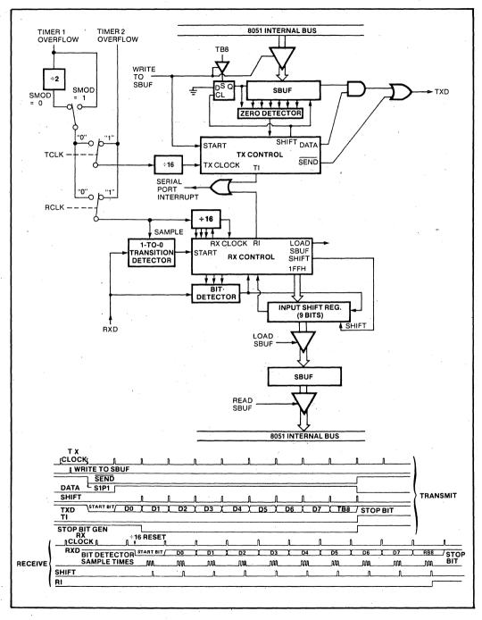
Figure 6-21B. Serial Port Mode 3 TCLK, RCLK, and Timer 2 are present in the 8052/8032 only.
