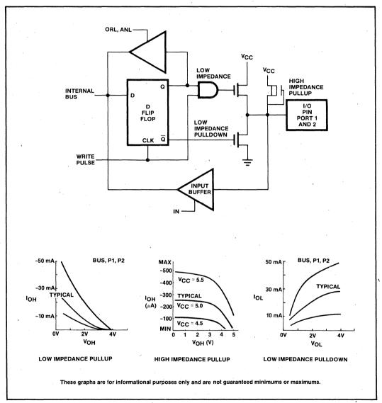
Figure 13-4. "Quasi-bidirectional" Port Structure
