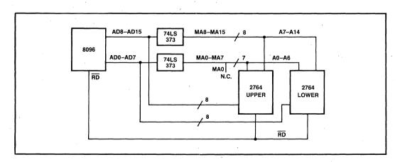
Figure 4-16. Memory Wiring Example—EPROM Only System
