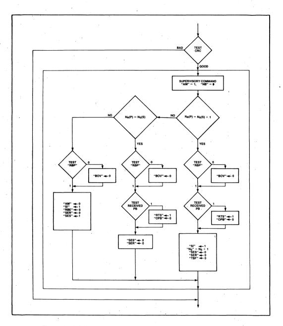
Figure 19-7d. SIU AUTO Mode Receive Flowchart—Supervisory Command
