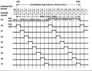
Figure 9. Individually Scanned Display Mode Timing.
