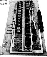
4K x 12 to 4K x 16 RAM Memory System with external timing and control. Used to replace an expensive core memory in an intelligent terminal CRT display.
