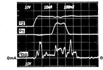
Figure 1. I<sub>DD</sub> transient current during shift cycles. I<sub>DD</sub> scale: 10mA/div.
