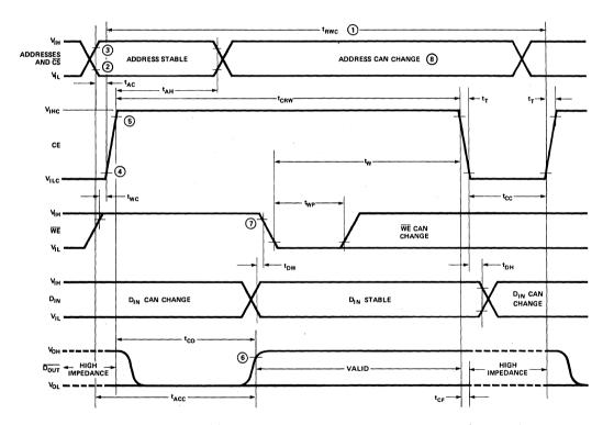
NOTES: 1. Minimum cycle timing is based on t<sub>T</sub> of 20ns.
