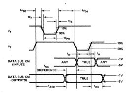
Figure 2. Timing Detail
