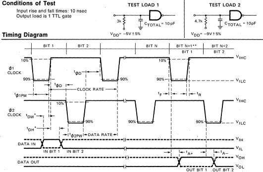
$t_{DW}$  and  $t_{DH}$  same for  $t_{02}$   $t_{N} = 256$  for 1402A, N = 512 for 1403A, N = 1024 for 1404A
