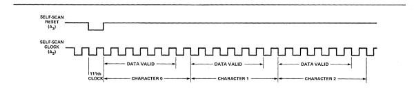
Figure 13. Gas Discharge (Self-Scan) Mode Timing - 18 Character Mode.
