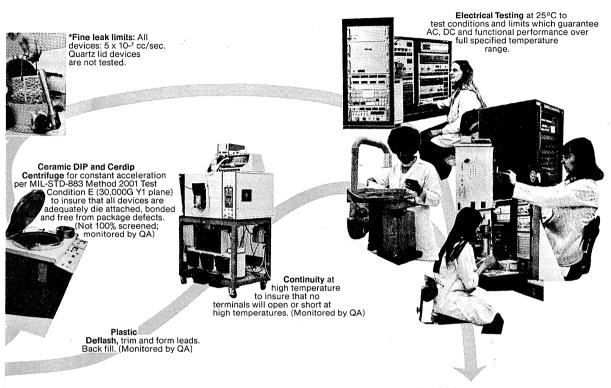
Final QA Acceptance per MIL-STD-883 Method 2009 External Visual, and Electrical AC, DC, Functional Tests at 25°C with correlated limits to guarantee performance over full specified temperature range (AQL 1%)
