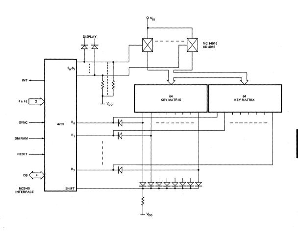
Figure 7. 128 Scanned Input Keys.
