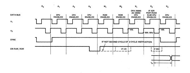
Figure 1. Timing Diagram.
