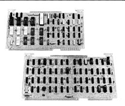
**DOS Channel and Interface Controller Boards**
