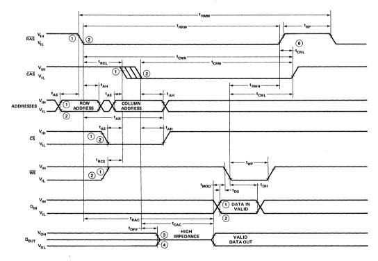
Notes: 1,2. VIHMIN and VILMAX are reference levels for measuring timing of input signals.
