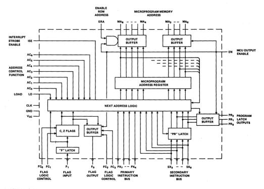
Figure 2. 3001 Block Diagram
