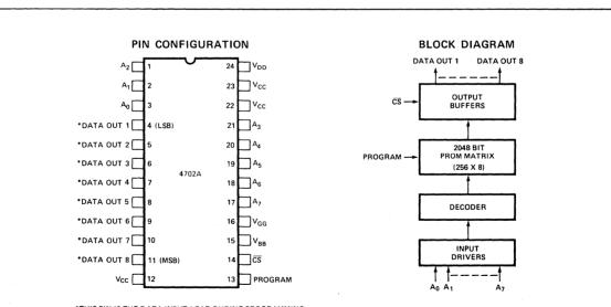
\*THIS PIN IS THE DATA INPUT LEAD DURING PROGRAMMING.
