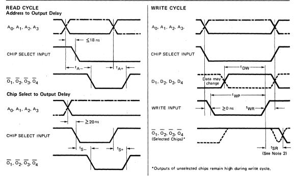
NOTE 2: t<sub>SR</sub> is associated with a read cycle following a write cycle and does not affect the access time.
