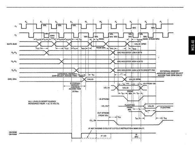
Figure 7. MCS-40 Timing Diagram for 4289.
