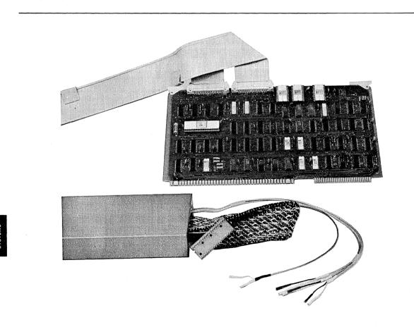
ICE-30 Module Board with External Cable and 40 Pin Connector
