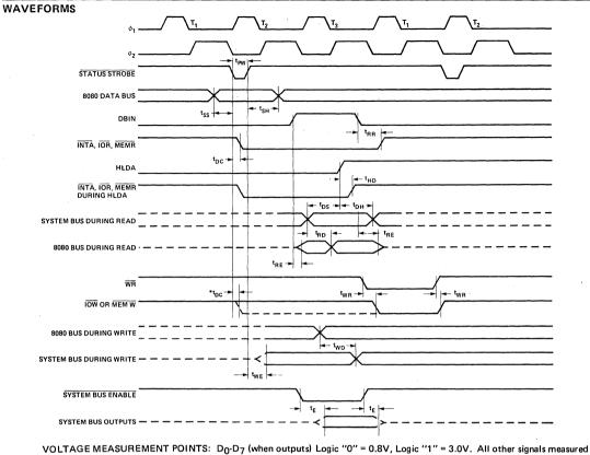
VOLTAGE MEASUREMENT POINTS: D<sub>0</sub>-D<sub>7</sub> (when outputs) Logic "0" = 0.8V, Logic "1" = 3.0V. All other signals meas at 1.5V.
