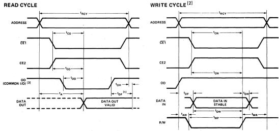
NOTES: 1.  $t_{DF}$  is with respect to the trailing edge of  $\overline{CE1}$ , CE2, or OD, whichever occurs first.
