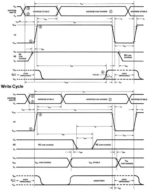
NOTES: 1. For Refresh cycle row and column addresses must be stable before t<sub>AC</sub> and remain stable for entire t<sub>AH</sub> period. 2. V<sub>IL</sub> MAX is the reference level for measuring timing of the addresses, <u>CS</u>, <u>WE</u>, and D<sub>IN</sub>.
