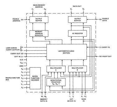
Figure 2. 3002 Block Diagram
