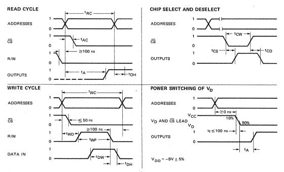
Note 1: Maximum value for  $\mathbf{t}_{\mathsf{AC}}$  measured at minimum read cycle.
