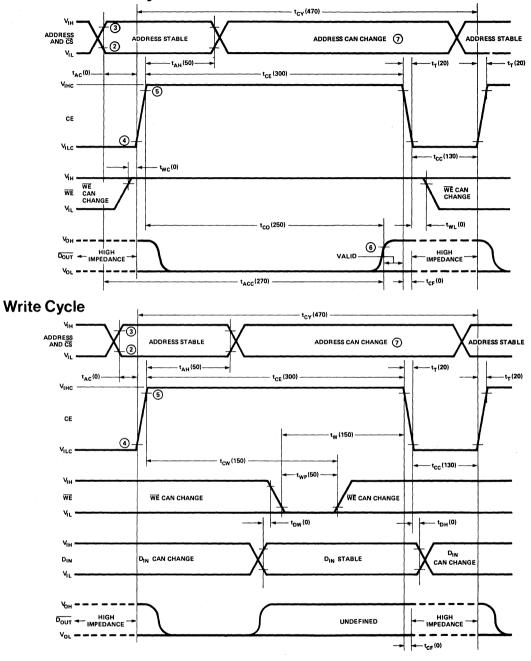
Read and Refresh Cycle <sup>[1]</sup> (Numbers in parentheses are for minimum cycle timing in ns)
