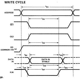
4. OD should be tied low for separate I/O operation.
