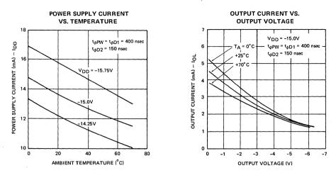
**A.C. Characteristics**  $T_A = 0^{\circ}C \text{ to } 70^{\circ}C, V_{SS} - V_{DD} = 15V \pm 5\%$
