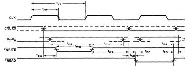
•WRITE AND READ PULSES HAVE NO TIMING LIMITATION WITH RESPECT TO CLK.
