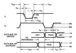
Figure 2. Timing Detail.
