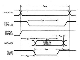
NOTE: 1. tDF is with respect to the trailing edge of CE1, CE2, or OD, whichever occurs first.
