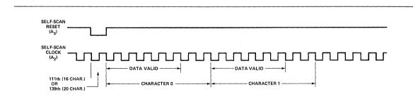
Figure 12. Gas Discharge (Self-Scan) Mode Timing - 16 or 20 Character Mode.
