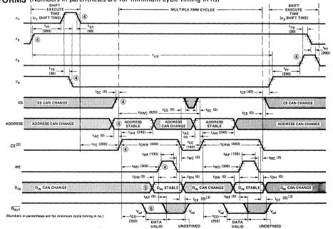
Notes: 2. When CE is off, the 2416 output level is determined by the external output termination.
