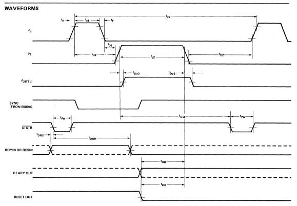
VOLTAGE MEASUREMENT POINTS:  $\phi_1, \phi_2$  Logic "0" = 1.0V, Logic "1" = 8.0V. All other signals measured at 1.5V.
