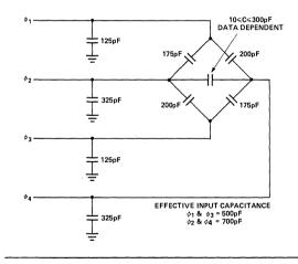
Figure 2. 2416 Equivalent Capacitance Circuit. (Maximum values shown.)
