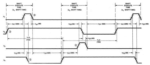
Note: 2. +2.0V and V<sub>DD</sub>-2.0V are the reference low and high level respectively for measuring the timing of  $\phi_1$ ,  $\phi_2$ ,  $\phi_3$  and  $\phi_4$ .
