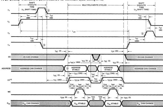
Notes: 2. +2.0V and V<sub>DD</sub>-2.0V are the reference low and high level respectively for measuring the timing of φ<sub>1</sub>...φ<sub>4</sub>, CE, CS, WE, and addresses. 3. +1.5V and +3.0V are the reference low and high level respectively for measuring the timing of D<sub>IN</sub>.
