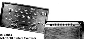
This system exercisor is designed to test up to 36 bits of information and address up to 262 thousand words of memory. The tester is mountable on the front of the memory unit by use of self-contained magnetic devices and is set up to be pluggable into the backplane of the memory system.
