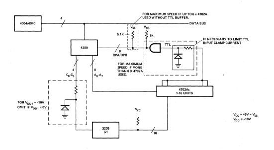
Figure 4. 4289 and 4702A Block Diagram.
