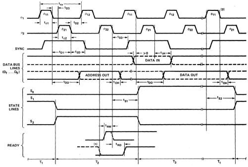
Notes: 1. READY line must be at "0" prior to  $\phi_{22}$  of T<sub>2</sub> to guarantee entry into the WAIT state. 2. INTERRUPT line must not change levels within 200 ns (max.) of falling edge of  $\phi_1$ .
