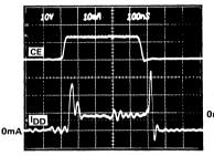
Figure 2. I<sub>DD</sub> transient current during I/O cycles. I<sub>DD</sub> scale: 10mA/div.
