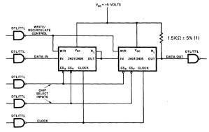
NOTE (1): The 2401/2405 is directly compatible device to device. An external  $1.5K\Omega$   $\pm$  5% load resistor is recommended for driving one TTL load with the 2401/2405 output.
