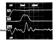
Figure 3. I<sub>BB</sub> transient current during a shift cycle. I<sub>BB</sub> scale: 50mA/div.
