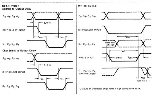
NOTE 1: t<sub>SR</sub> is associated with a read cycle following a write cycle and does not affect the access time.
