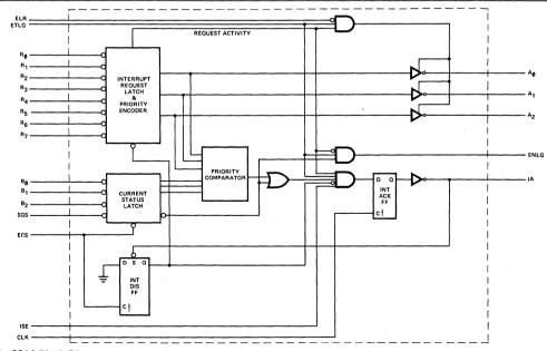
Figure 1. 3214 Block Diagram.
