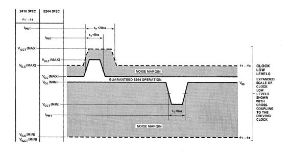
Figure 3. Noise Margins Between 5244 Output Specs and 2416  $\phi_1 \dots \phi_4$  Input Requirements.
