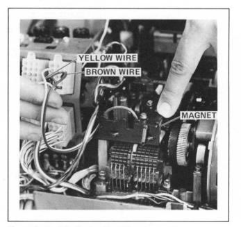
Figure 3-5. Distributor Trip Magnet
