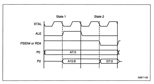
Figure 12-8. External Data Read Bus Cycle (Page Mode)
