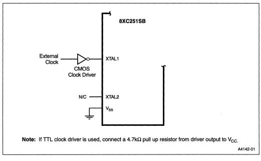
Figure 10-3. External Clock Connection
