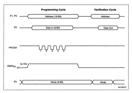
Figure 13-2. OTPROM Programming Waveforms
