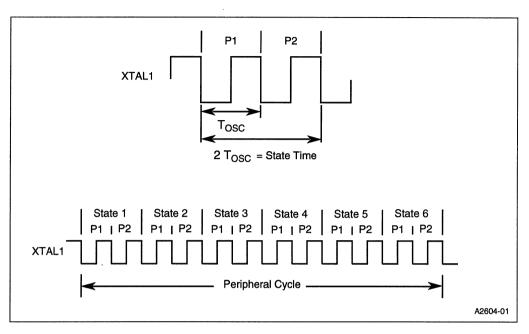
Figure 2-3. 8XC251SB Timing
