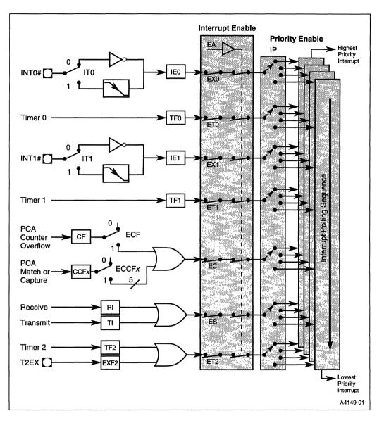
Figure 5-1. Interrupt Control System
