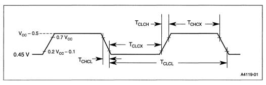
Figure 10-4. External Clock Drive Waveforms
