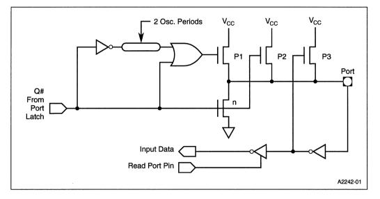
Figure 6-4. Internal Pullup Configurations
