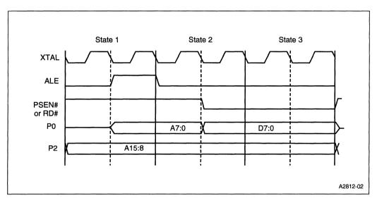
Figure 12-10. External Code Fetch or Data Read Bus Cycle with One PSEN#/RD# Wait State (Nonpage Mode)
