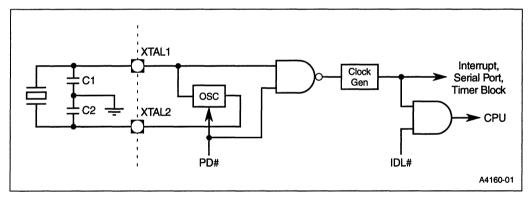
Figure 11-2. Idle and Powerdown Clock Control
