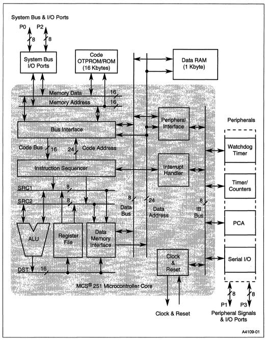
Figure 2-1. Functional Block Diagram of the 8XC251SB
