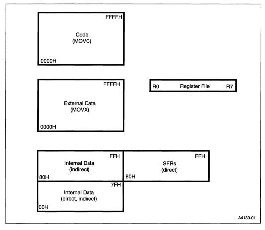
Figure 3-2. Address Spaces for the MCS<sup>®</sup> 51 Architecture
