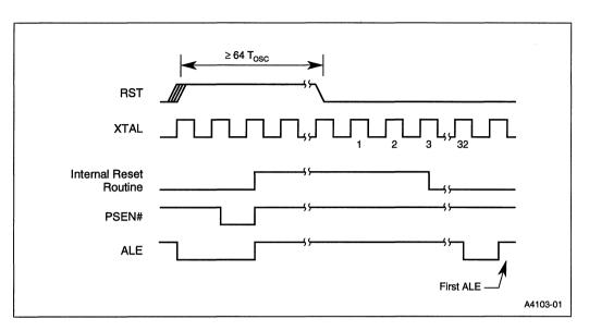
Figure 10-5. Reset Timing Sequence
