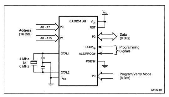
Figure 13-1. Setup for Programming and Verifying
