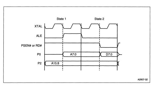
Figure 12-4. External Code Fetch or Data Read Bus Cycle (Nonpage Mode)
