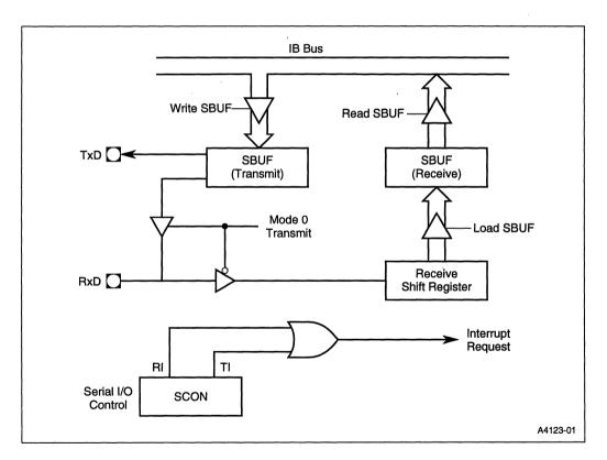
Figure 9-1. Serial Port Block Diagram
