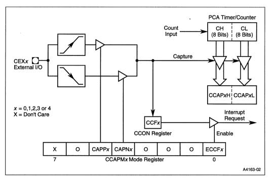
Figure 8-2. PCA 16-bit Capture Mode
