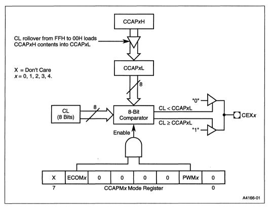
Figure 8-5. PCA 8-bit PWM Mode
