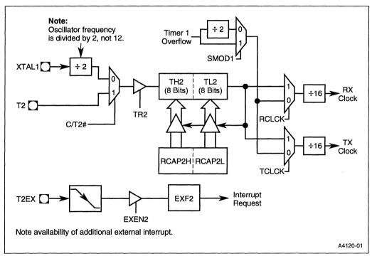
Figure 9-5. Timer 2 in Baud Rate Generator Mode
