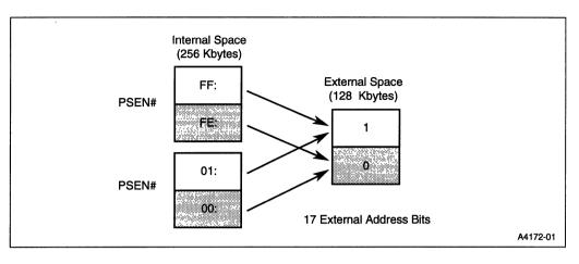
Figure 12-2. Internal and External Memory Spaces for RD1 = 0, RD0 = 1
