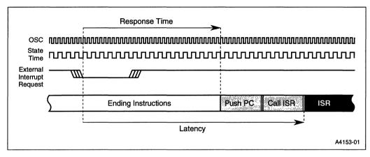
Figure 5-5. The Interrupt Process
