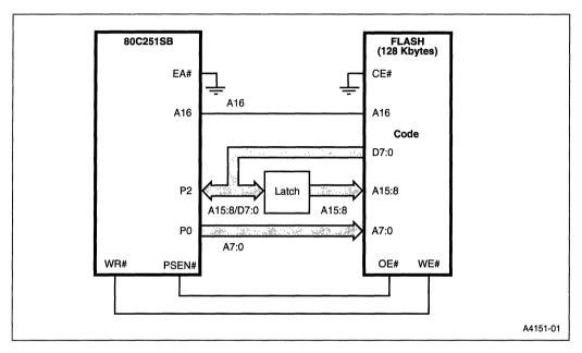
Figure 12-17. 80C251SB in Page Mode with External Flash
