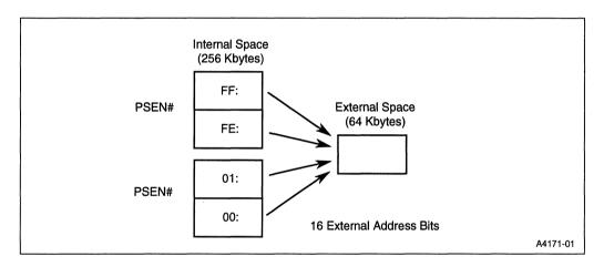
Figure 12-1. Internal and External Memory Spaces for RD1 = 1, RD0 = 0
