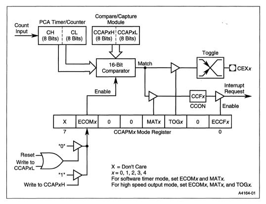
Figure 8-3. PCA Software Timer and High-speed Output Modes
