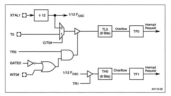
Figure 7-3. Timer 0 in Mode 3, Two 8-bit Timers
