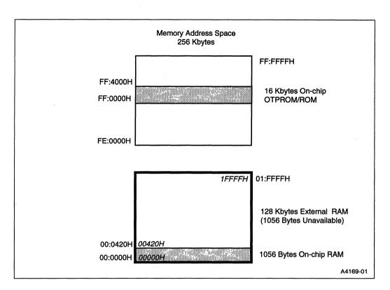
Figure 12-16. The Memory Space for the System of Figure 12-15
