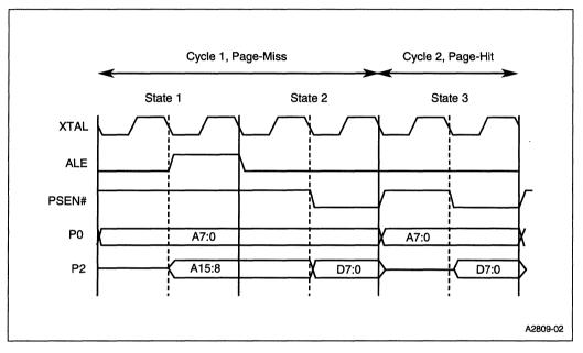
Figure 12-7. External Code Fetch Bus Cycle (Page Mode)
