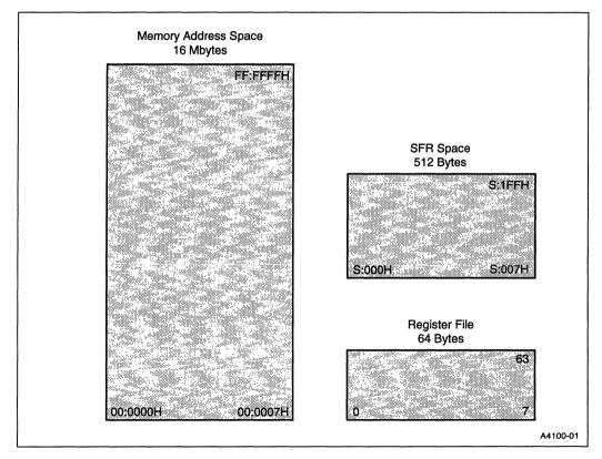
Figure 3-1. Address Spaces for MCS<sup>®</sup> 251 Microcontrollers
