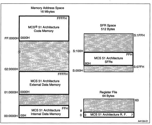
Figure 3-3. Address Space Mappings MCS<sup>®</sup> 51 Architecture to MCS<sup>®</sup> 251 Architecture
