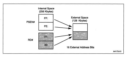
Figure 12-3. Internal and External Memory Spaces for RD1 = 1, RD0 = 1
