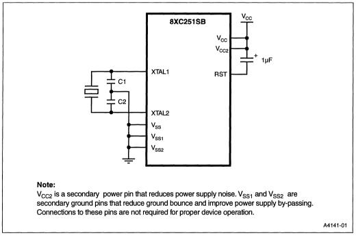
Figure 10-1. Minimum Setup
