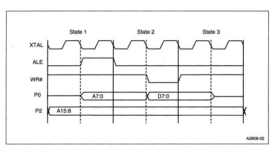
Figure 12-5. External Write Bus Cycle (Nonpage Mode)
