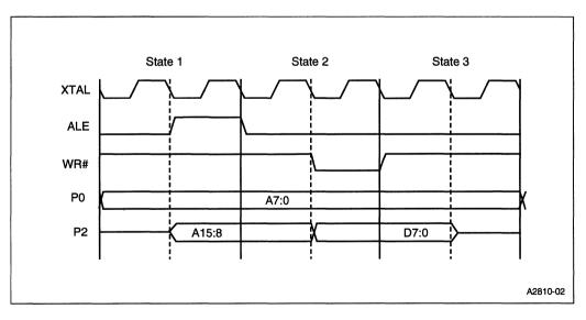
Figure 12-9. External Write Bus Cycle (Page Mode)
