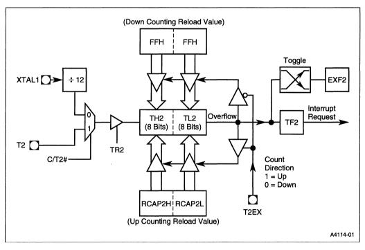
Figure 7-8. Timer 2: Auto Reload Mode (DCEN = 1)
