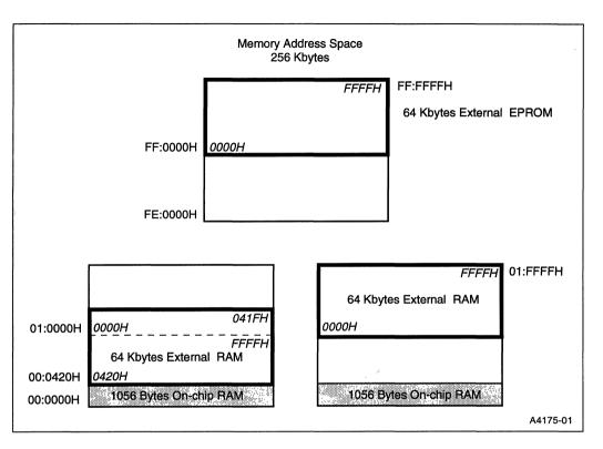
Figure 12-14. The Memory Space for the Systems of Figure 12-13 and Figure 12-18
