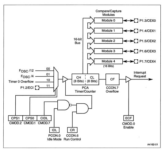
Figure 8-1. Programmable Counter Array
