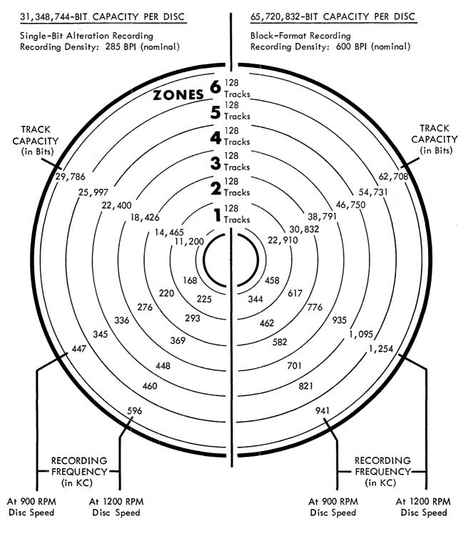
Figure 5. MAXIMUM CAPACITIES OBTAINED WITH SIX-ZONE DISC FORMAT
