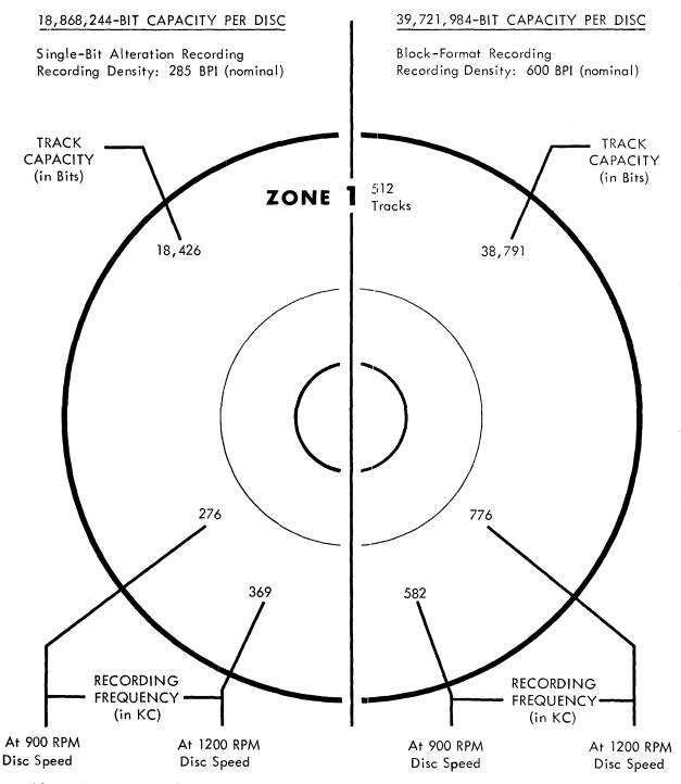
Note: Maximum single-zone capacities are achieved by using only the four outermost heads serving each disc face and the total of 512 tracks they access (128 tracks per head). In short, 768n<512N where n and N are the maximum permissible track capacities in bits for the innermost and the third head out, respectively.
