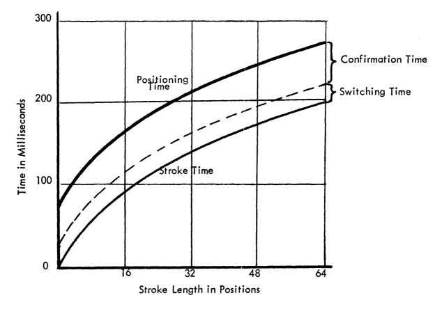
Figure 2. ACCESS TIME OF MODEL dp/f-5020
