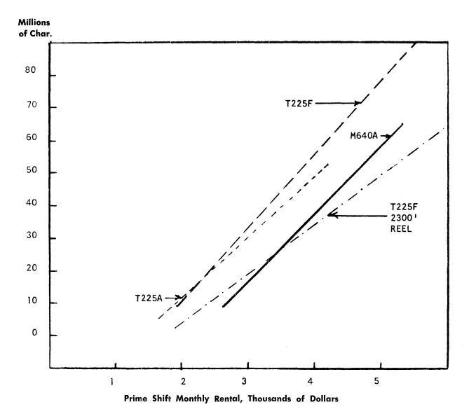
Figure 2. EFFECTIVE ON LINE STORAGE COSTS FOR GE 225 M640A DISC AS COMPARED TO GE TAPE UNITS T225A, T225F AND T225F WITH 2300' REEL
