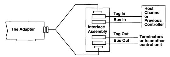
**Note:** Refer to *System/370, 4300, and 9370 Processors Input/Output Equipment Installation Manual – Physical Planning,* GC22-7064, for details and restrictions regarding channel cabling. The Interface Assembly is wired for "high" channel priority.
