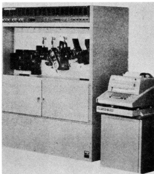
120.100.3-.4 Figure 10-12.—UNIVAC 1549 card reader-punch-interpreter (CRPI).
