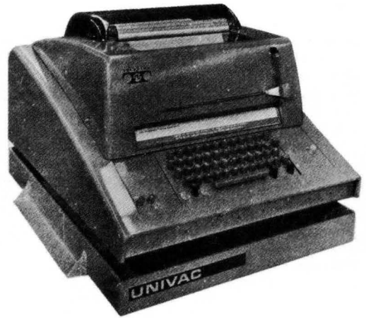
120.100.4 Figure 10-21.—Input-Output keyboard-printer.
