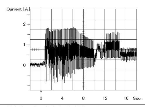
Figure 55. Typical Current Form of 12V at Start Up of DTLA-307060/307075
