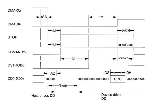
Figure 32. Ultra DMA cycle timing chart (Device terminating Read)
