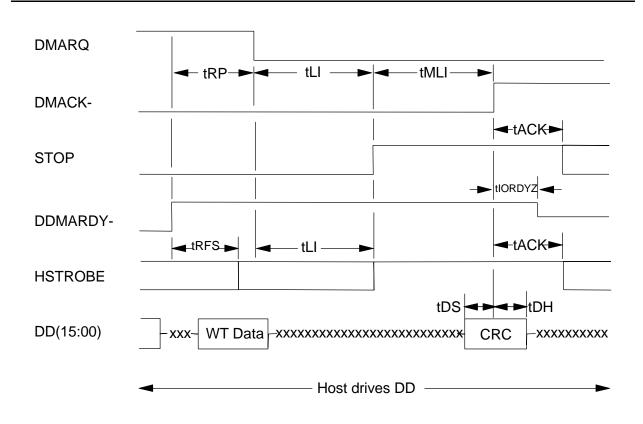
Figure 38. Ultra DMA cycle timing chart (Device Terminating Write)
