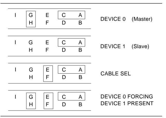
Figure 45. Jumper positions for 15 logical head default
