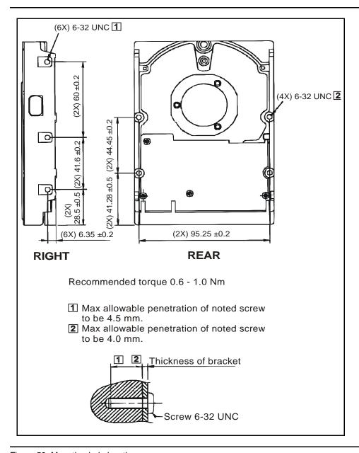
Figure 59. Mounting hole locations
