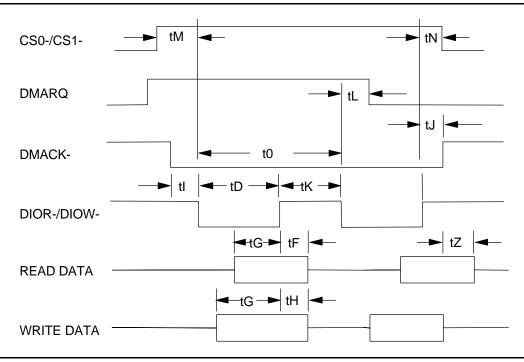
Figure 24. Multiword DMA cycle timing chart
