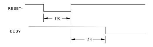
Figure 20. System reset timing chart
