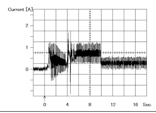
Figure 53. Typical Current Form of 12V at Start Up of DTLA-305010/305020/305030/305040
