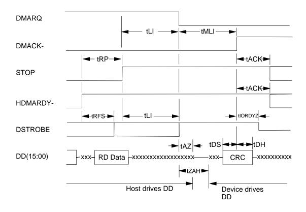
Figure 30. Ultra DMA cycle timing chart (Host terminating Read)
