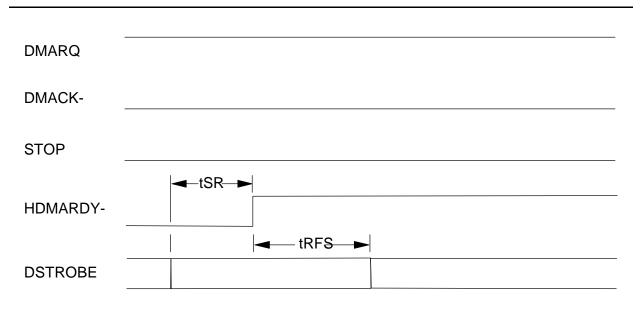
Figure 28. Ultra DMA cycle timing chart (Host pausing Read)
