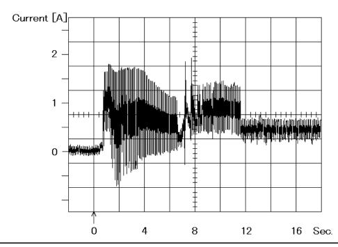
Figure 54. Typical Current Form of 12V at Start Up of DTLA-307015/307020/307030/307045
