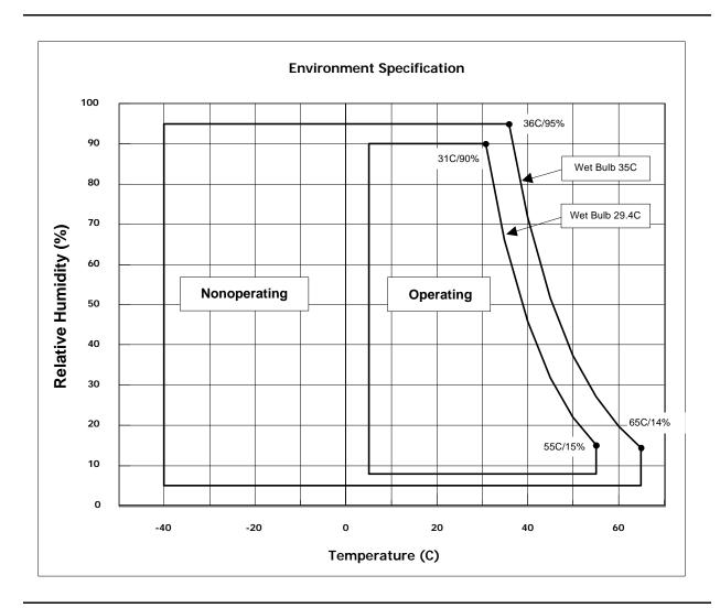
Figure 49. Limits of temperature and humidity
