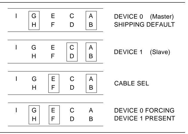
Figure 44. Jumperpositions for normal use
