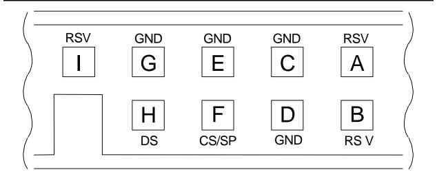
Figure 43. Jumper pin assignment
