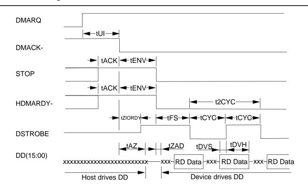
Figure 26. Ultra DMA cycle timing chart (Initiating Read)
