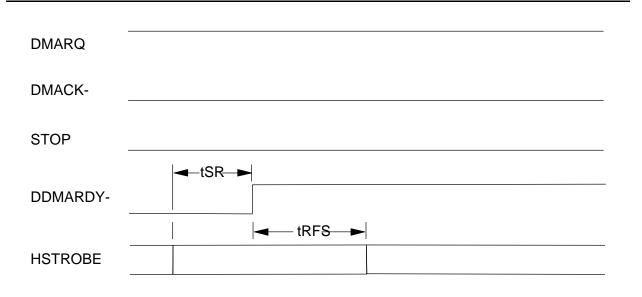
Figure 36. Ultra DMA cycle timing chart (Device Pausing Write)
