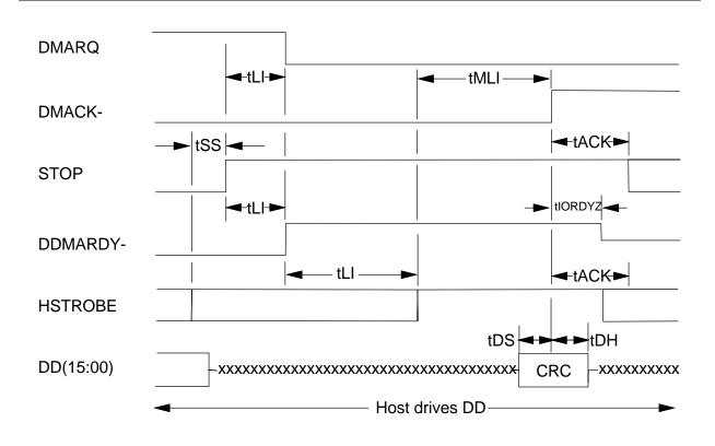
Figure 40. Ultra DMA cycle timing chart (Host Terminating Write)
