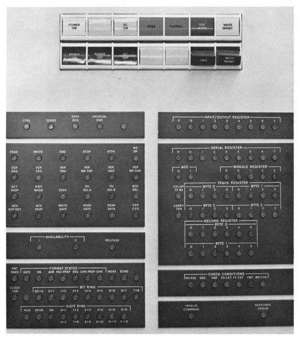
Figure 21. IBM 7631 Model 3 Operator Panel
