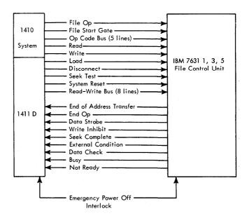
Figure 16. Operating Lines - IBM 1410 Data Processing System to/from IBM 7631 1, 3, and 5
