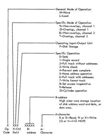
Figure 17. Disk Storage Operation Code Format
