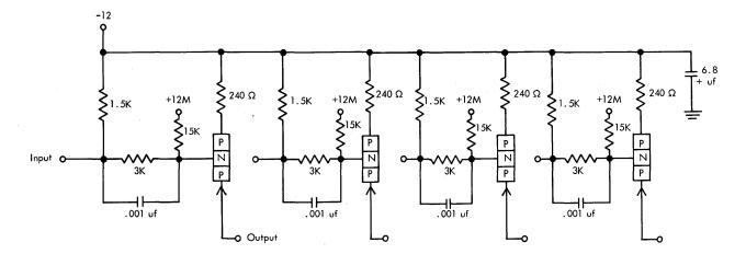
Figure 39. Line Driver - Dispersed Load (TAB)
