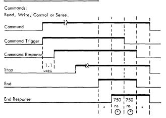
Timings shown are maximum. They are measured from the time a signal rises on the interface cable until the 7631 brings up its responding signal on the interface cable.
