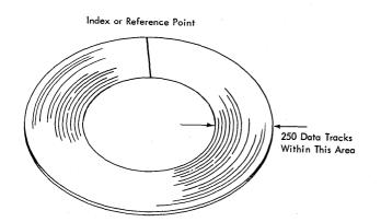
Figure 1. Magnetically Coated Disk
