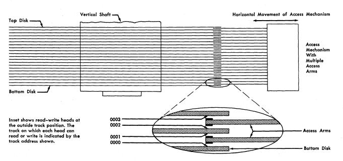
Figure 4. Module and Access Mechanism
