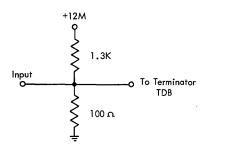
Figure 52. End of Line Terminator (TAC)
