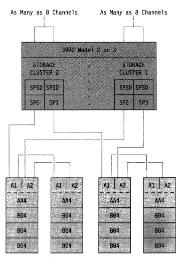
Figure 29. Example of 3380 Model AA4 Strings Attached to a 3990 Model 2 or 3
