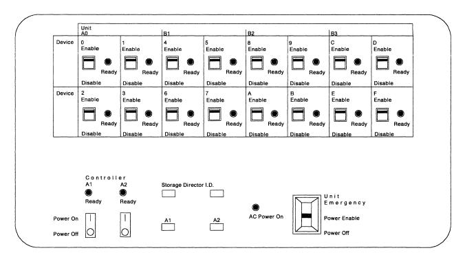
Figure 38. 3380 Model AD4 and AE4 Operator Control Panel
