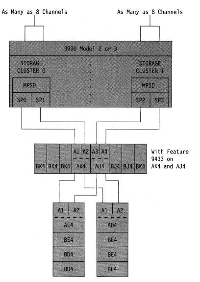
Figure 35 is an example of a 3380 4-path string and AE4 and AD4 strings sequentially connected to two paired storage paths in a 3990 Model 2 or 3.
