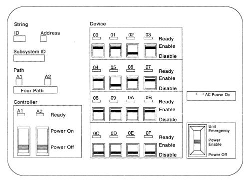
Figure 43. 3380 Model AJ4 or AK4 4-Path Operator Control Panel with Feature 9433. Used for attachment to 3990 Model 2 or 3 Storage Controls. There is a similar panel on the second A-unit that specifies controllers A3 and A4 and devices 10 through 1F.
