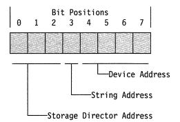
Figure 47. Unit Address Composition for Single or 2-Path 3380 String
