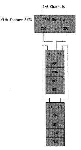
Figure 22. Example of 3380 Model AD4 and AE4 Strings Attached to a 3880 Model 3
