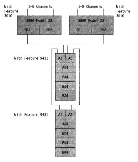
Figure 25. Example of 3380 Model AJ4 and AK4 2-Path Strings Attached to Dual-Framed 3880 Model 23s
