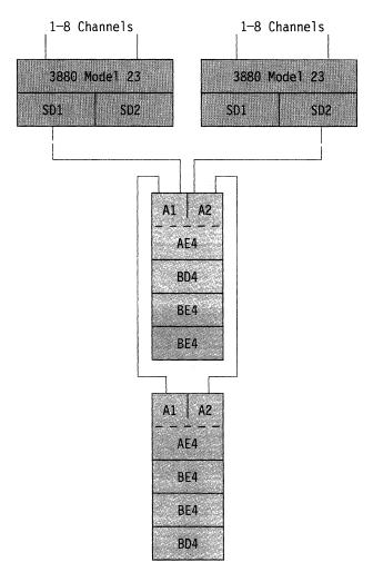
Figure 23. Example of 3380 Model AE4 Strings Attached to Dual-Framed 3880 Model 23s
