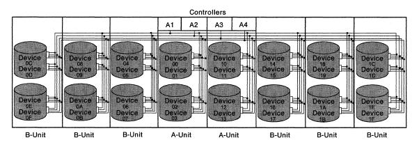
Figure 14. Internal Paths for 3380 Enhanced Subsystem 4-Path String
