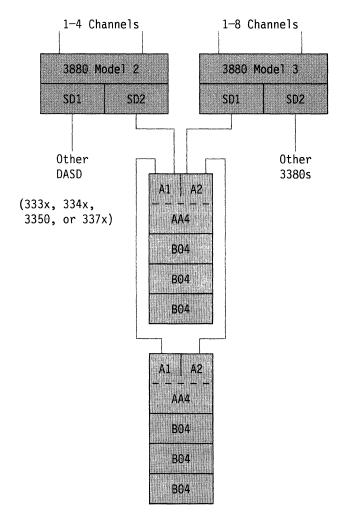
Figure 19. Example of 3380 Model AA4 Strings Attached to 3880 Model 2 and 3 Storage Directors
