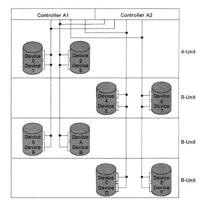
Figure 12. Internal Paths for Standard Model AA4 String
