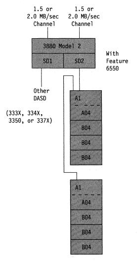
Figure 18. Example of 3380 Model A04 Strings Attached to a 3880 Model 2
