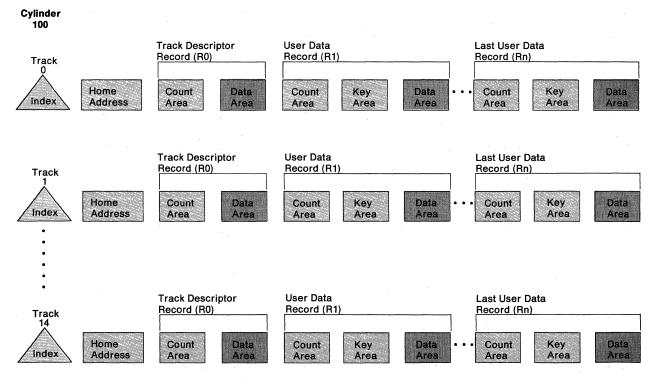
Figure 56. Track and Record Format, Simplified Representation (Standard R0)
