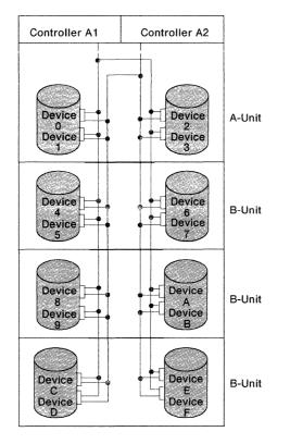
Figure 13. Internal Paths for 3380 Extended Capability String
