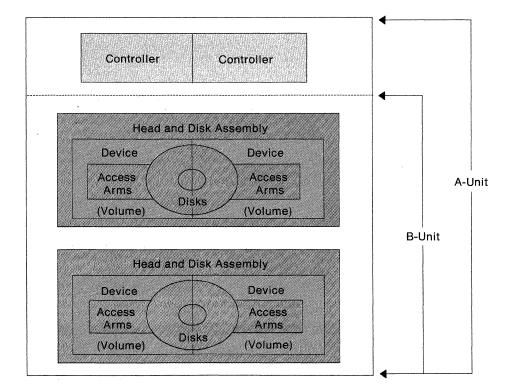
Figure 2. The 3380 A-Unit and B-Unit (excluding Model A04)
