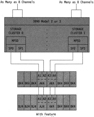
Figure 32 is an example of two 3380 4-path strings sequentially connected to the paired storage paths in the same 3990 Model 2 or 3.
