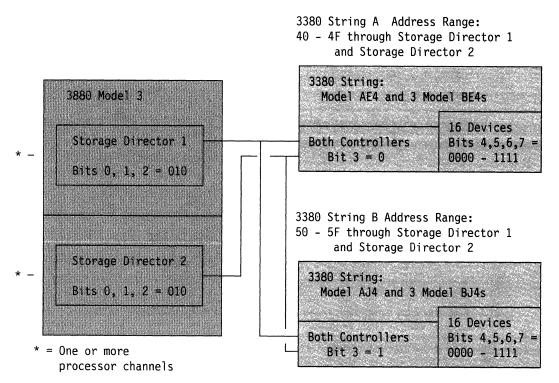
Figure 50. Addressing Example. Two 3380 2-Path Strings (32 Devices) Attached to Two 3880 Storage Directors
