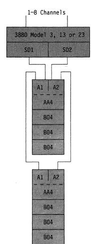
Figure 20 shows two 3380 AA4 strings sequentially connected to both storage directors of a 3880 Model 3, 13 or 23.
