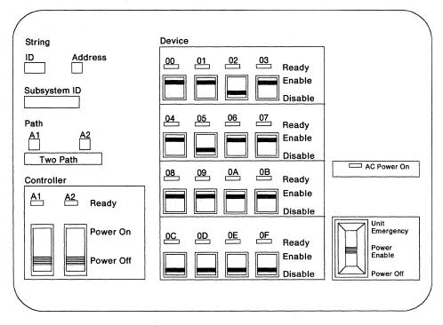
Figure 42. 3380 Model AJ4 or AK4 2-Path Operator Control Panel with Feature 9432. Used for attachment to 3990 Storage Controls.
