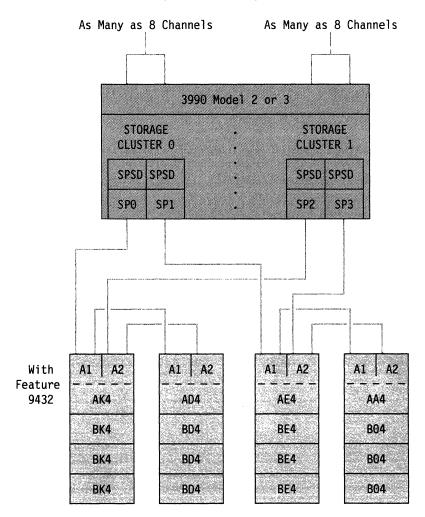
Figure 33. Example of Intermixed 3380 2-Path Strings Attached to a 3990 Model 2 or 3
