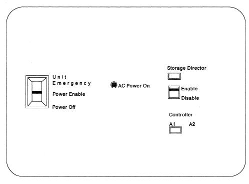
Figure 36. 3380 Model A04 Operator Control Panel
