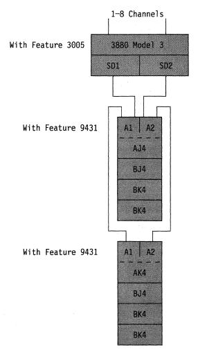
Figure 24. Example of 3380 Model AJ4 and AK4 2-Path Strings Attached to a 3880 Model 3
