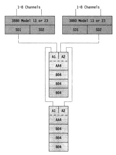
Figure 21. Example of 3380 Model AA4 Strings Attached to Two 3880 Models 13 or 23
