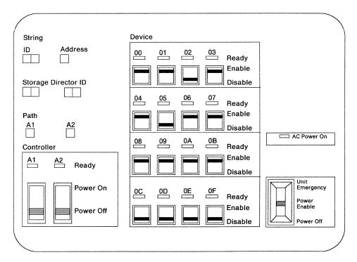
Figure 41. 3380 Model AJ4 or AK4 2-Path Operator Control Panel with Feature 9431. Used for attachment to 3880 Storage Controls.
