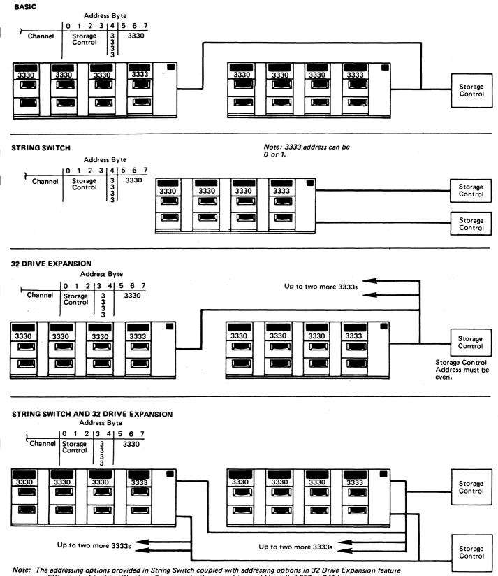
can cause difficulty in drive identification. For example, the same drive could be called 559 or 241 by system messages, dependent upon how the 3333 was plugged on installation. 3333 String Switch Addresses should be plugged both odd (1-3) or even (0-2).
