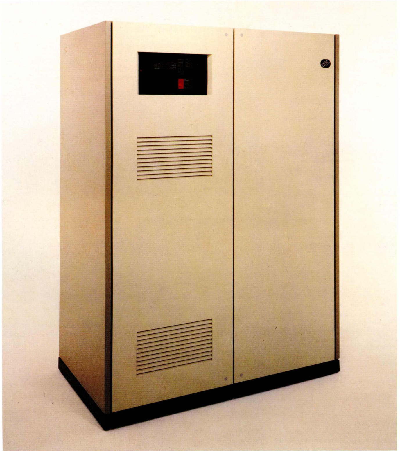
IBM 3745 Communication Controller Model 210 base unit – offering attachment capability for up to eight host computers, as well as up to 128 low/medium speed lines, eight T1 or 2 Mbps lines, eight IBM Token-Ring networks, or certain combinations of these
