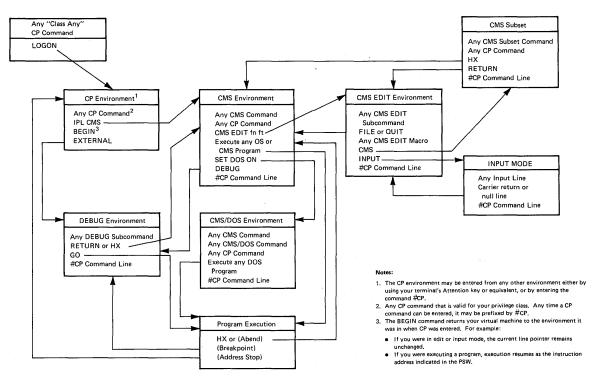
Figure 1. VM/SP Environments and Mode Switching
