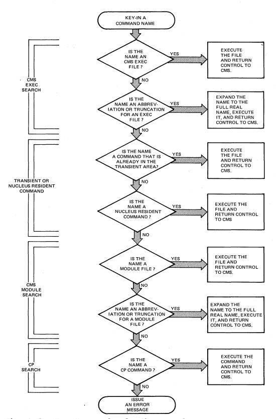
Figure 4. How CMS Searches for the Command to Execute
