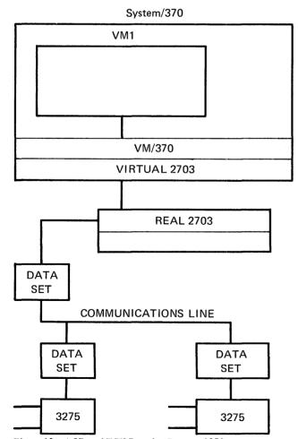
Figure 13. A Virtual TCU Running Remote 3270s
