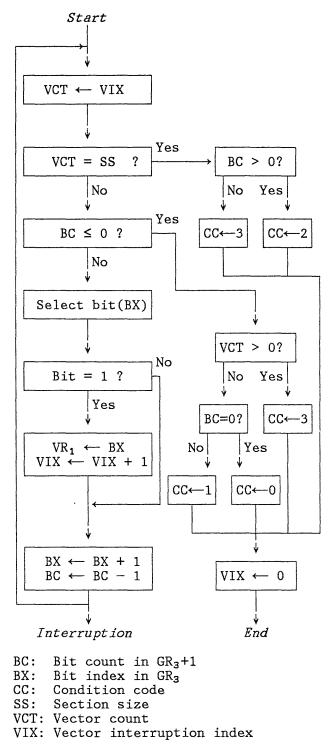
Figure 3-1. Execution of LOAD BIT INDEX
