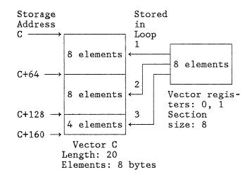
Since all vectors are stored contiguously, the stride for the three vector instructions VLD, VAD, and VSTD is set to one by specifying a value of zero in the  $RT_2$  subfield. This may be done in the assembler language either by placing a zero inside the parentheses of the stride subfield, as in:
