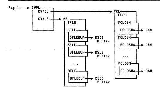
Figure 17. Control Blocks Required for CVAF Filter Services
