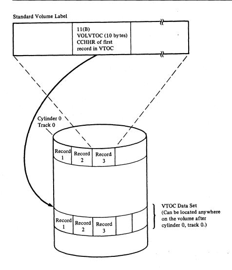
Figure 1. Locating the Volume Table of Contents (VTOC)
