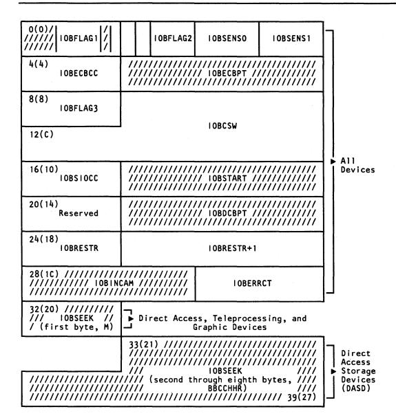
Figure 21. Input/Output Block (IOB) Format
