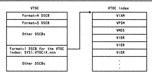
Figure 3. Relationship of a VTOC to Its Index
