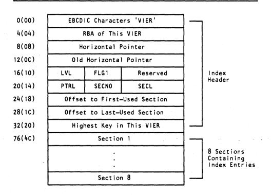
Figure 4. Format of the VTOC Index Entry Record (VIER)
