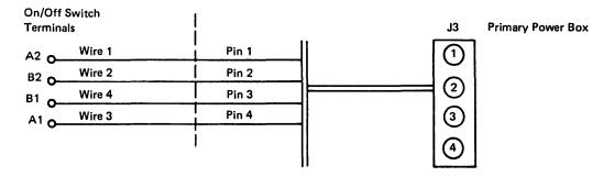
Figure E-1 (Part 2 of 2). Operator Panel Connections
