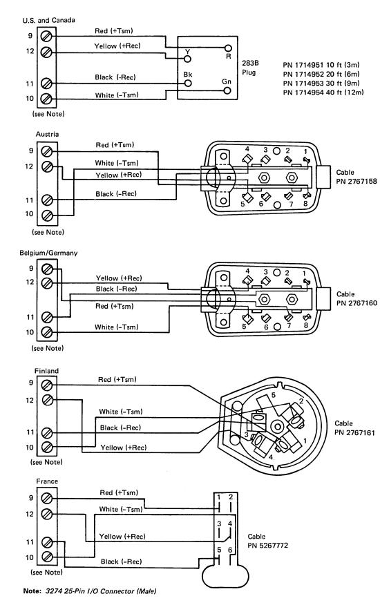
Figure 5-9. Communication Cable Plugs — Four-Wire, Nonswitched
