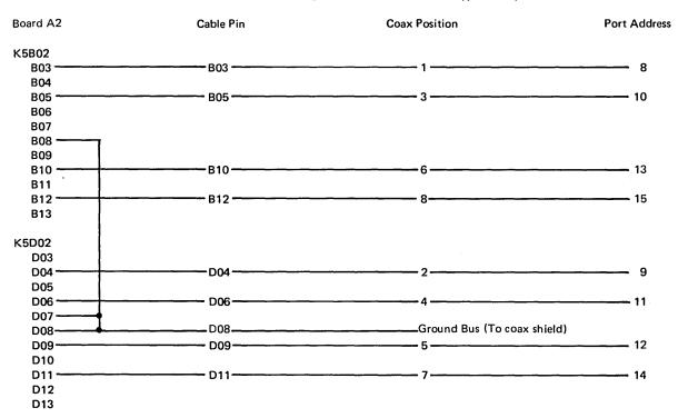
Figure C-6 (Part 7 of 8). Logic Board Cables
