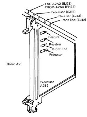
Figure 5-11. 4800-bps Integrated Modem Card LED Locations and Test Results
