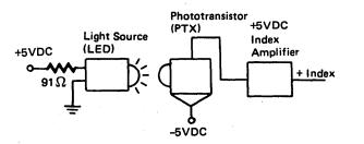
If a scope is available, turn AC power on and check for an index pulse width of 1.7 to 8.0 ms.
