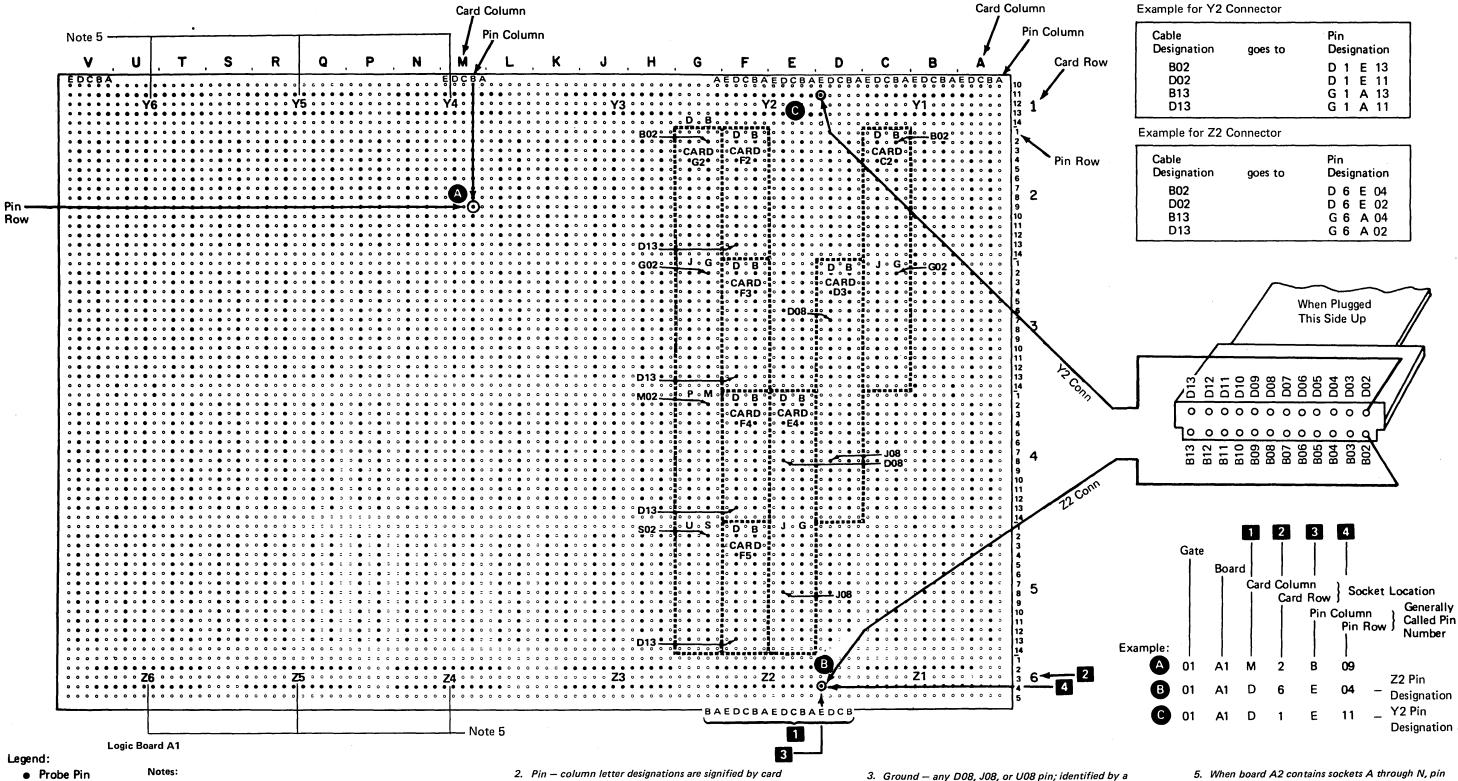
1. For multiple-socket cards (such as cards G2, E4, D3, and C2 in illustration), card location designation is specified by the uppermost row. Example: The location of card G2 (which actually occupies four sockets) is specified by the uppermost row, G2. If this card is located on board A1, its location is identified as A1G2.
