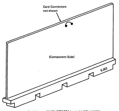
Note: Card Jumper (1) PN 2731801 is required for proper operation of the modem.
