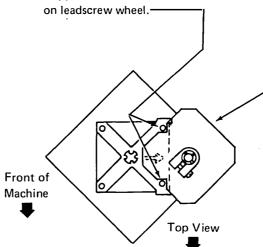
Slide stepper motor toward leadscrew until pins contact notches. No clearance is allowed.
