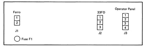
Figure B-5. Primary Power Box Connections
