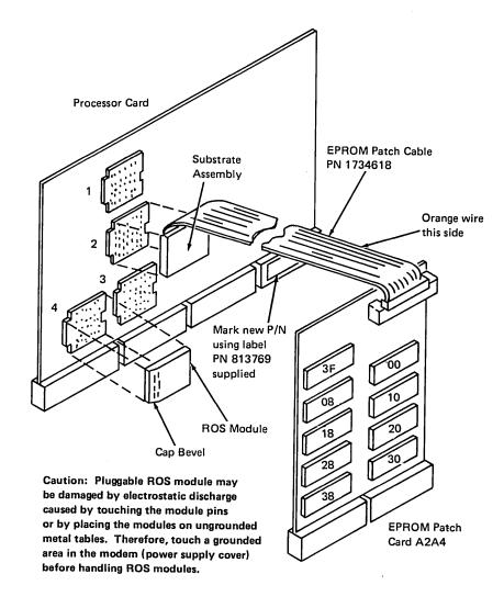
Note: The PROM patch card is used when functional changes are required for the Integrated Modem. The PROM card connects via a cable to the processor card module socket. All pluggable ROS modules removed from the processor card are stored in a plastic box in the 3274. Some of these modules may be used again when the field change updates the processor card with the released level part numbers.
