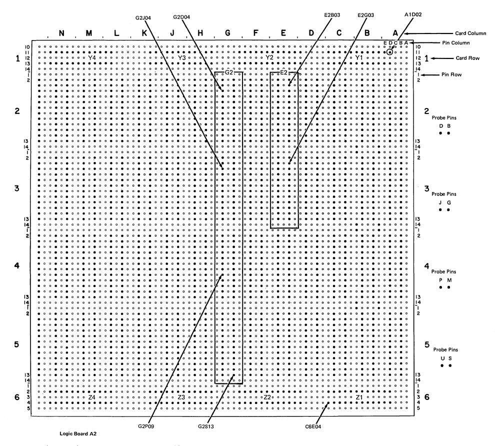
Figure C-7 (Part 2 of 2). Logic Board Card, Connector, and Pin Locations
