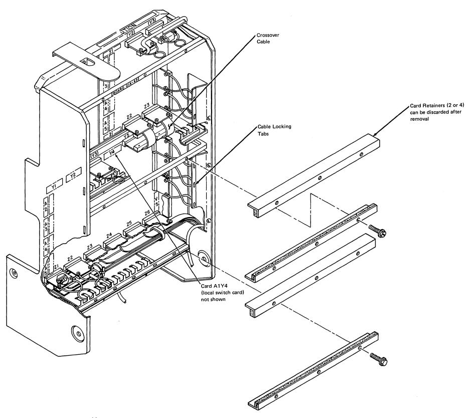
Figure 4-10. Logic Gate Assembly
