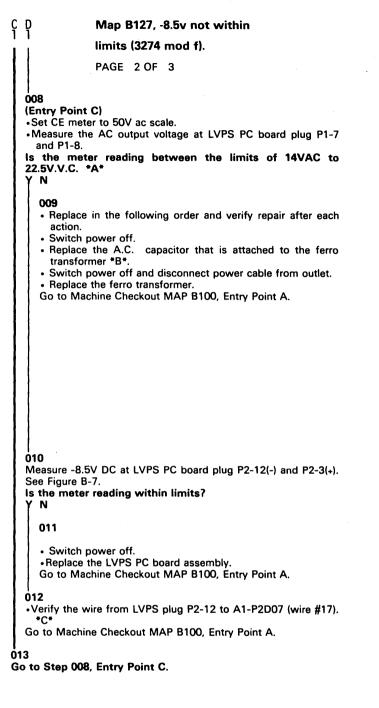
Short Circuited power supply diode can also cause a low A.C. meter reading.
