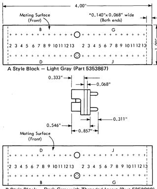
B Style Block — Dark Gray with Threaded Insert (Part 5353868) B-Style Block — Dark Gray, No Threaded Insert (Part 5353869)
