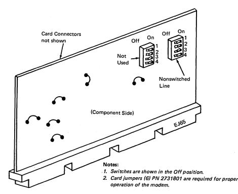
Figure 5-17. 9600-bps Integrated Modem Front-End Card (A2E2)
