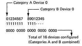
In the preceding example the machine has one type A and two type B driver/receiver cards installed in sockets A through K of board A2. The indications from line 2 are: category A devices 0–7 are powered on; category B devices 0–3 are powered on; category B devices 4–7 are disabled. The most likely repair action would be to replace the driver/receiver card for category B devices 4–7 (A2J2).
