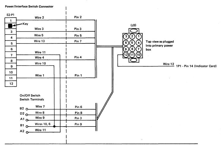
Cable —Primary Power Box to Operator Panel (Model C)
