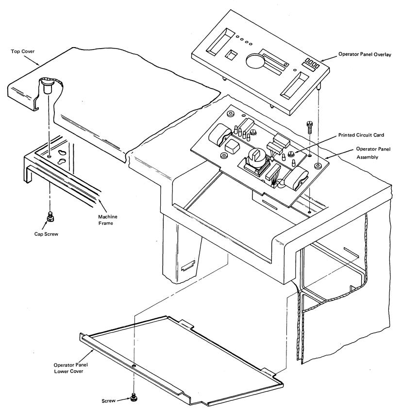
Figure 4-8. Operator Panel and Cover
