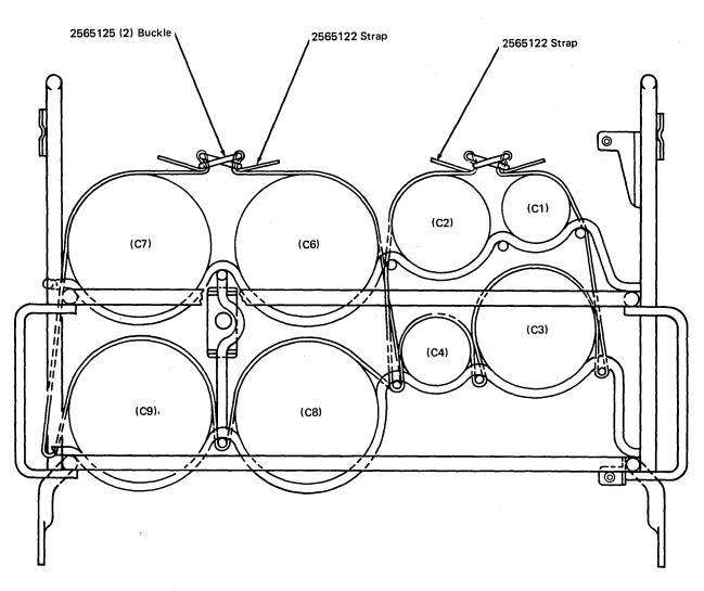
Figure B-13. Capacitor Strapping
