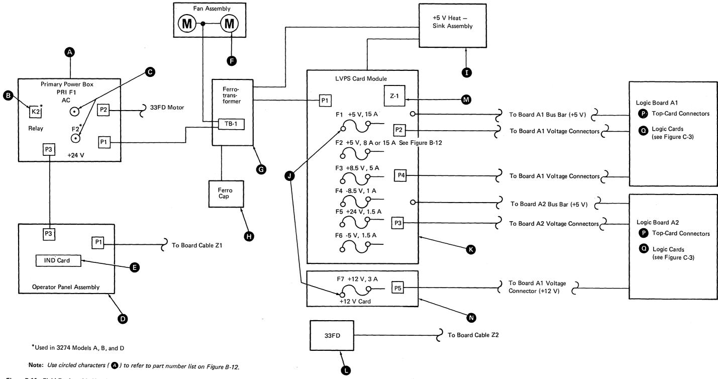
Figure B-11. Field Replaceable Unit Power Locations and Connections
