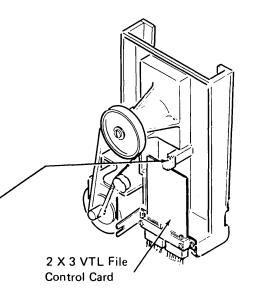
2 X 3 VTL Test Points (only the major components are shown, as an aid in locating pins)
