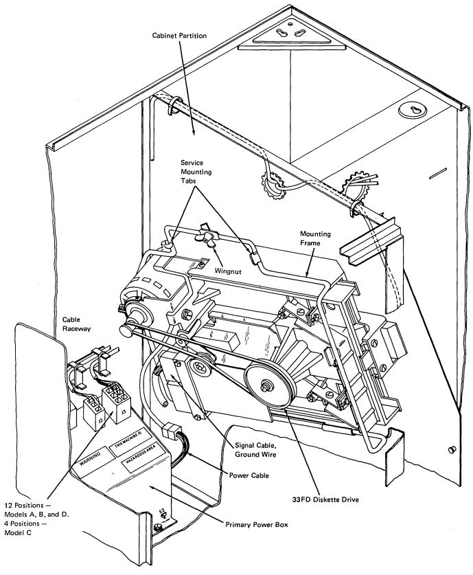
Figure A-2. Field Replaceable Unit Location — Diskette Drive
