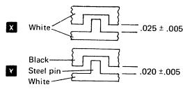
Note: When the stepper motor is replaced, ensure that the leadscrew wheel is the new style (black). The old style leadscrew wheel (white) will wear excessively if used with the new steel pin stepper motor drive.
