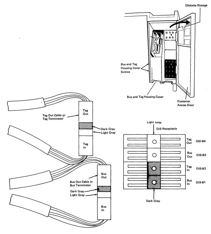
Figure 4-9. Bus and Tag Cables
