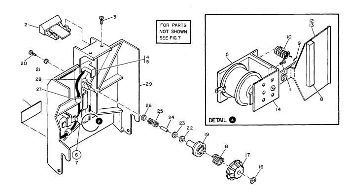
FIGURE 8. CLAMPING PLATE ASSEMBLY—ANGLE MOUNT. SEE LIST 8.
