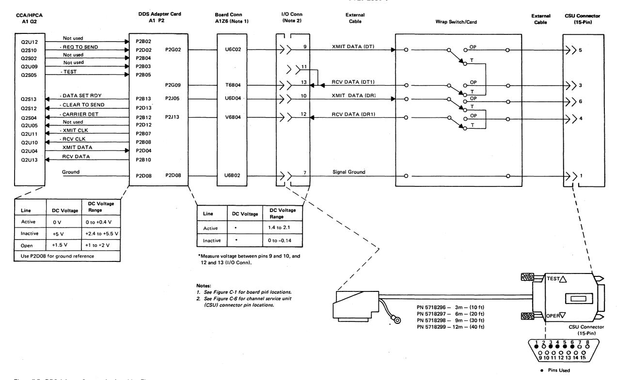
Figure 5-5. DDS Adapter Communications Line Flow
