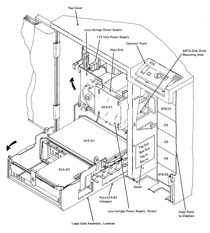
Figure A-1. Field Replaceable Unit Locations — Logic Gate Lowered
