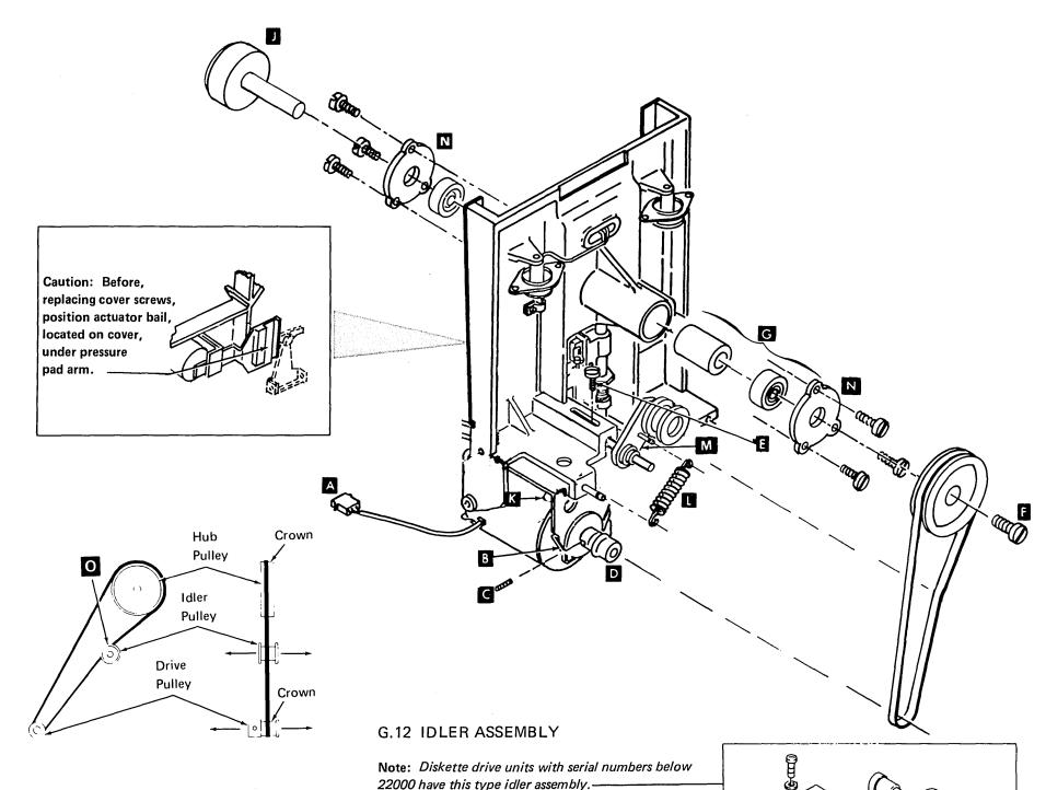
Note: Late-model diskette drives have an idler pulley with a narrow groove. To adjust belt tracking, loosen screw and slide idler until belt rides in center of hub pulley. Since the drive pulley does not have a crown, the belt does not have to be centered exactly on the drive pulley on these drives.
