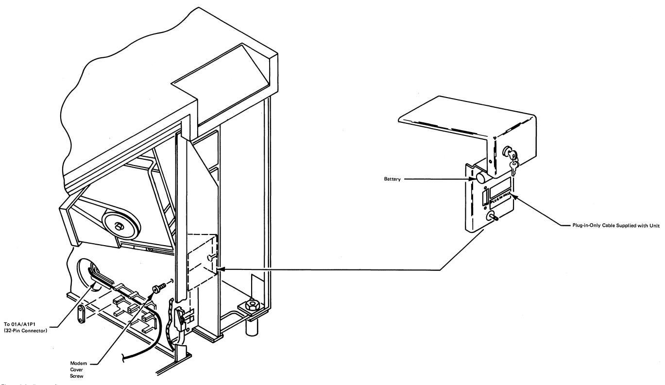
Figure 6-1. Encrypt/Decrypt Feature Component Locations
