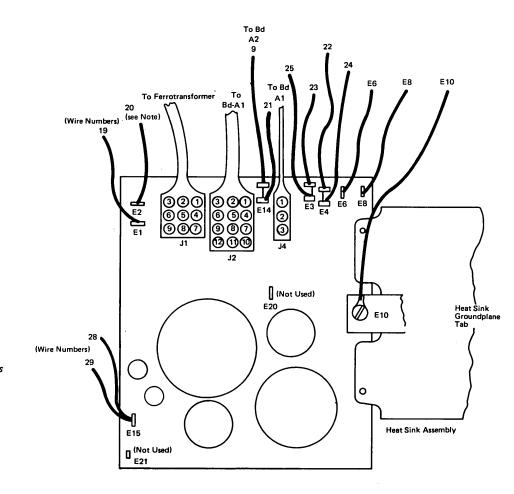
Note: Wire 20 is terminated at E2 on Models A, B, and D. It is not functional on Model C.
