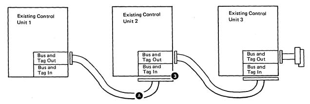
Note: Bus and Tag Out and Bus and Tag In receptacle locations may vary from control unit to control unit.
