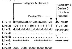
Line 1 shows coax port addresses (0-31). In this example, the 3274 is configured for 32 devices (24 category A displays and 8 category B printers). Category A devices are always shown first, followed by printer and category B devices (separated by two spaces).
