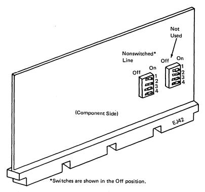
Figure 5-16. 4800-bps Integrated Modern Front-End Card (A2E2)
