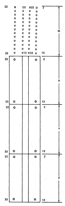
Figure C-8. Top-Card Connector Pin Locations
