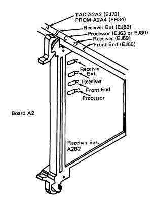
Figure 5-12. 9600-bps Integrated Modem Card LED Locations and Test Results
