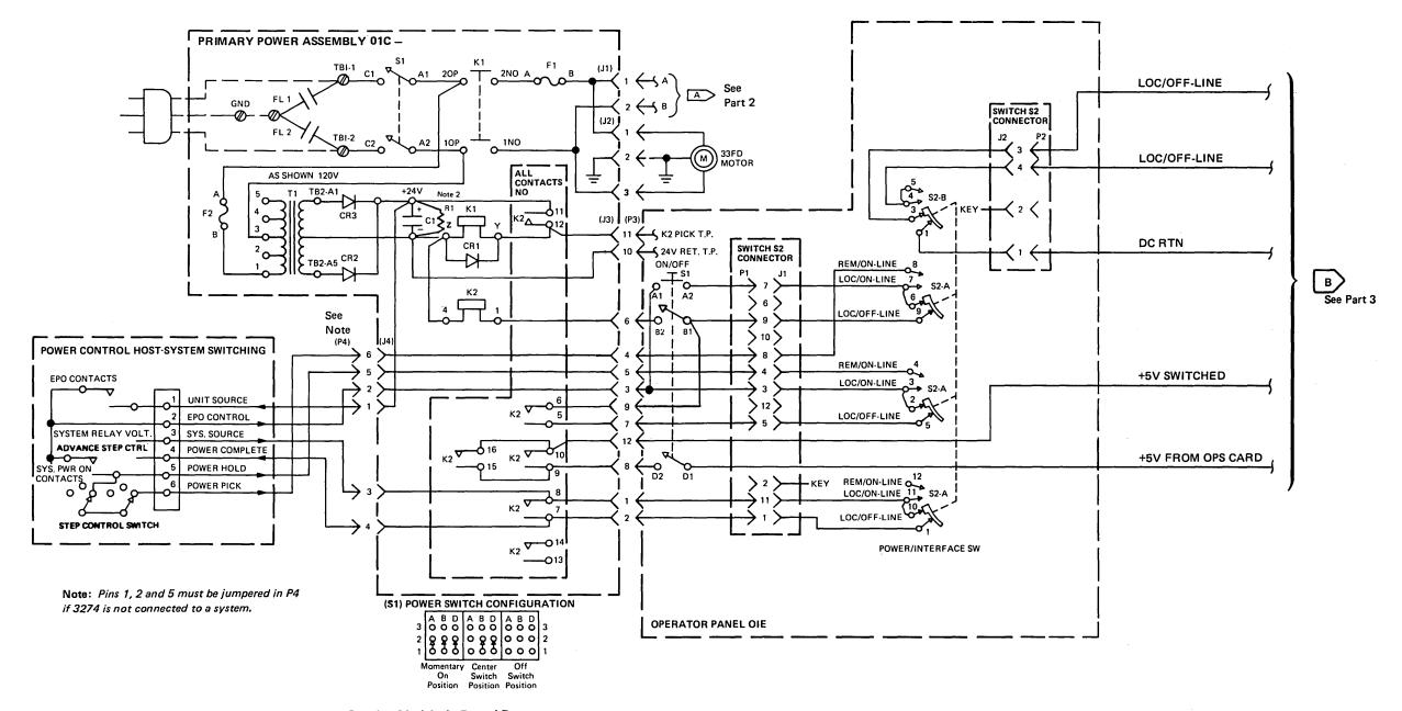
Figure B-1 (Part 1 of 3). Power Supply and Operator Panel — Models A, B, and D
