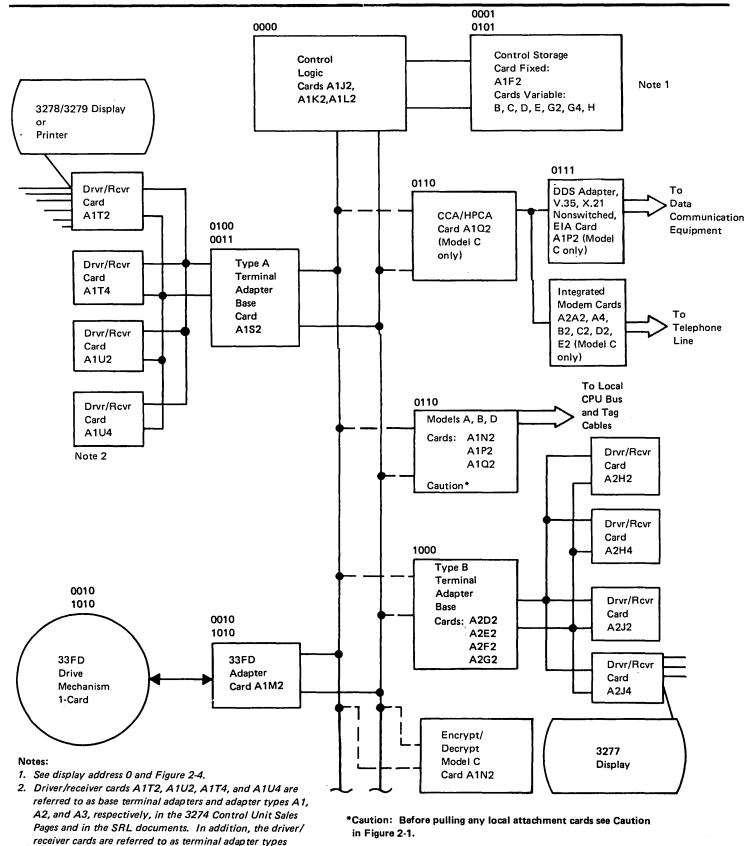
Figure 2-2. 3274 Hardware Block Diagram
