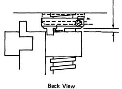
Note: Doing the lower and upper limit stop adjustments ensures that the head carriage can always access tracks 0 and 76, but will not overtravel.
