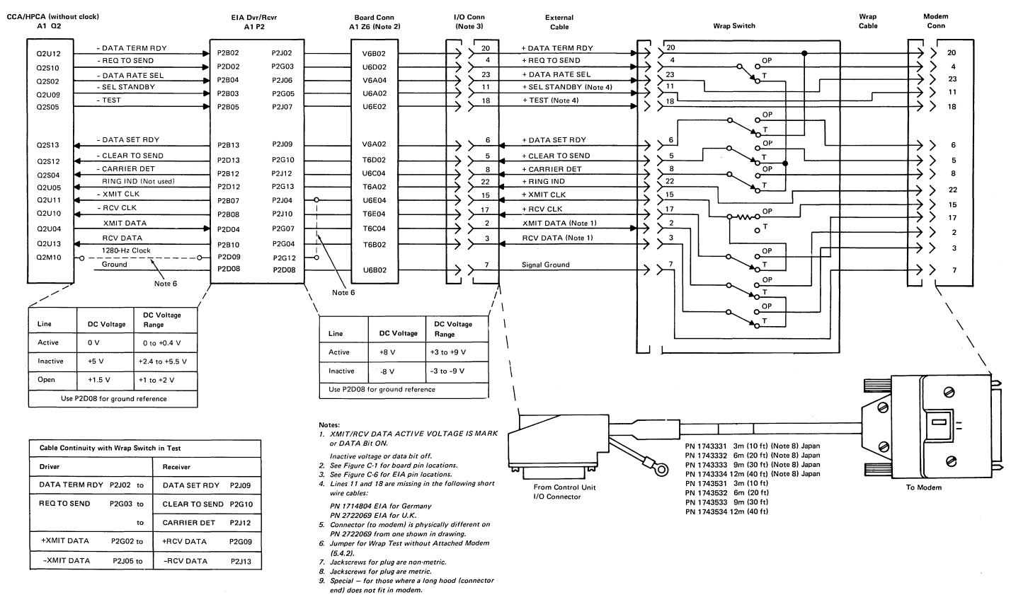
Figure 5-4. EIA Communications Line Flow for Modems
