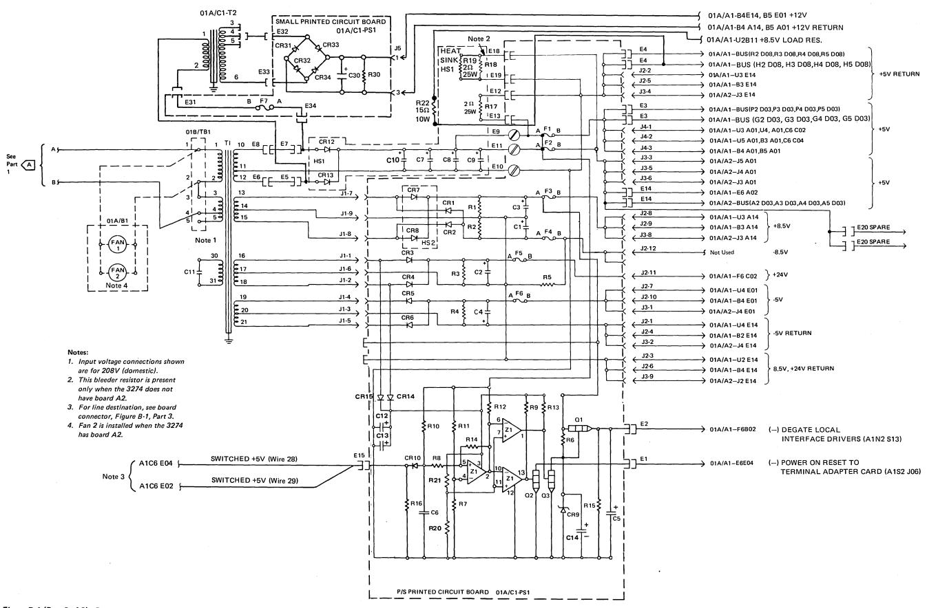
Figure B-1 (Part 2 of 3). Power Supply and Operator Panel — Models A, B, and D
