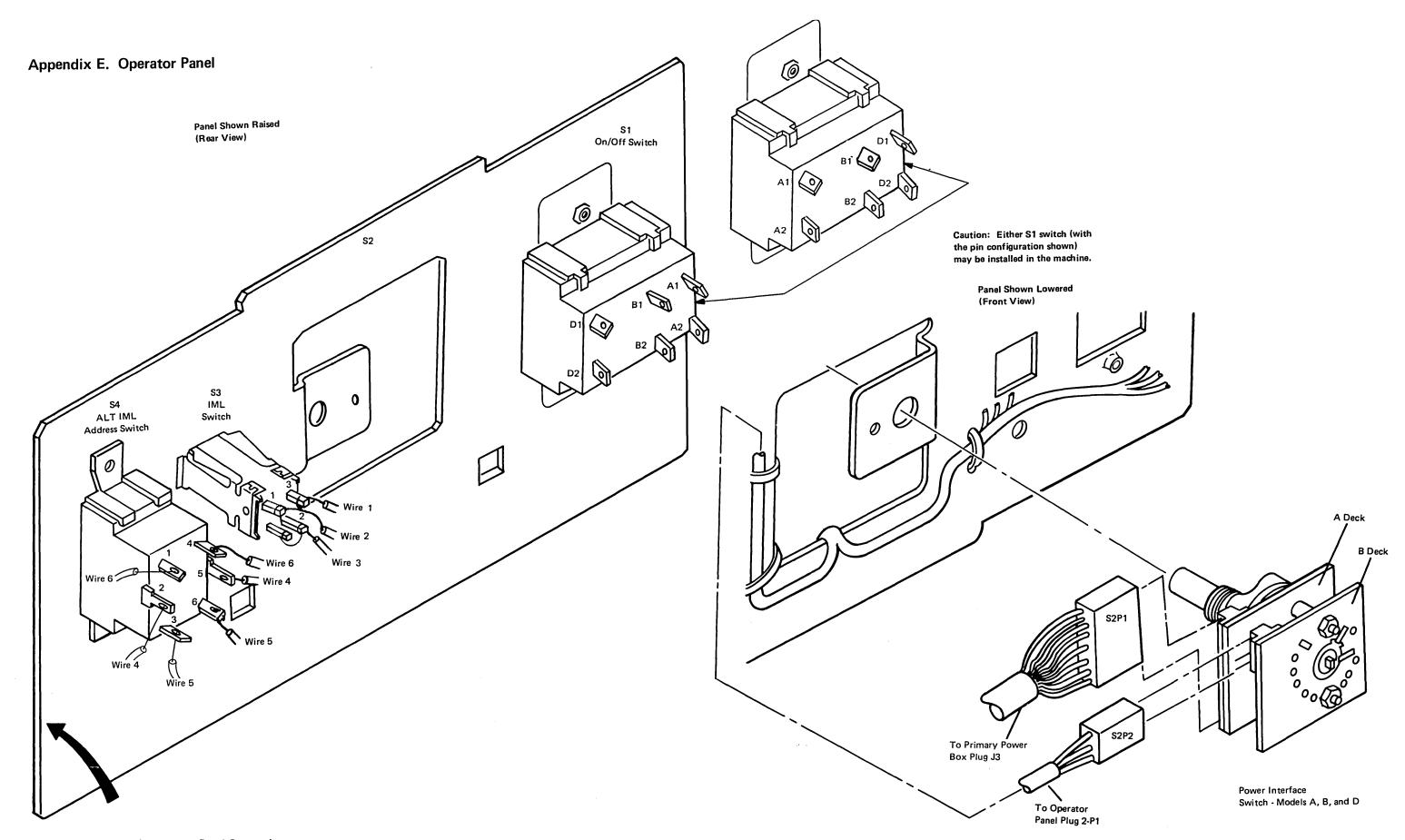
Figure E-1 (Part 1 of 2). Operator Panel Connections
