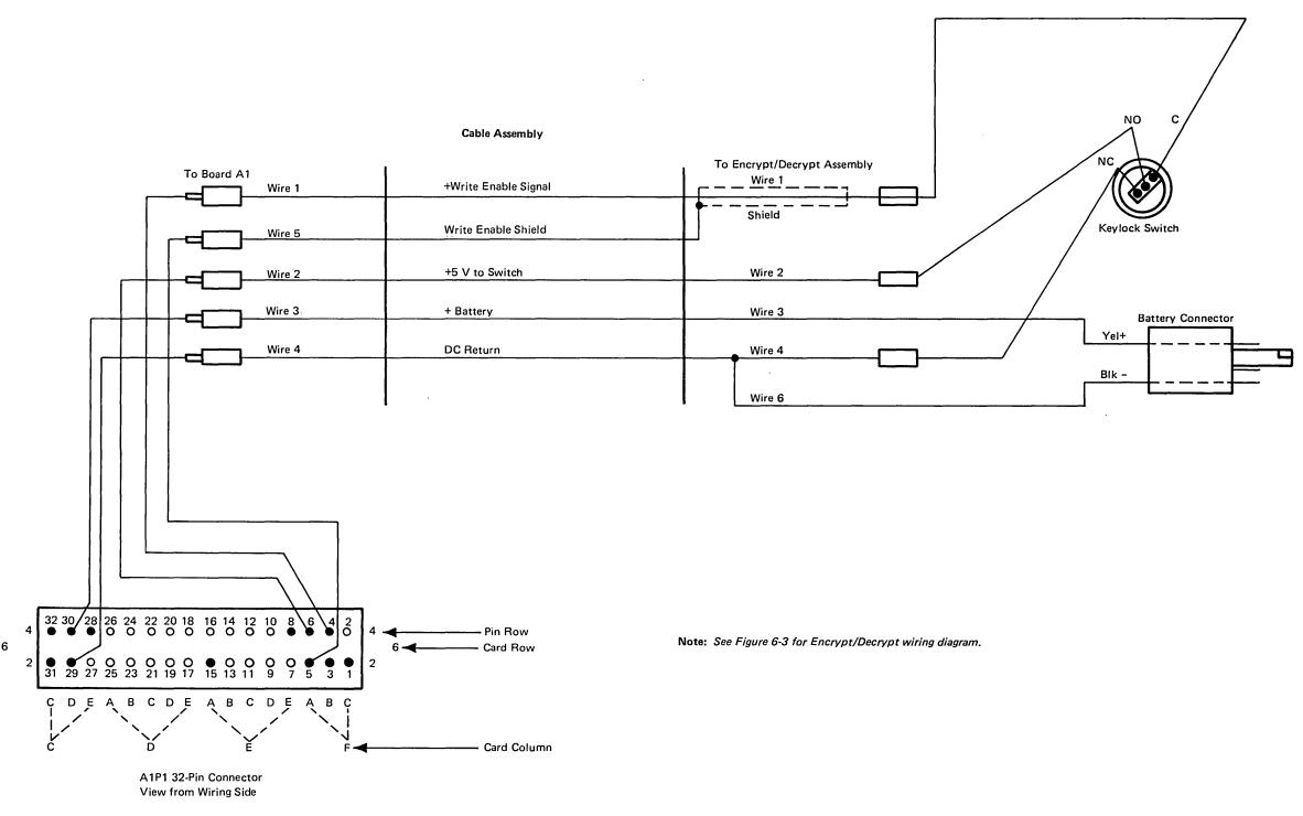
Figure 6-2. Encrypt/Decrypt Cable Connections
