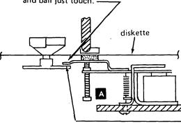
Rotate adjusting screw clockwise 1/2 to 3/4 turn and check for clearance between arm and bail at all tracks ....
