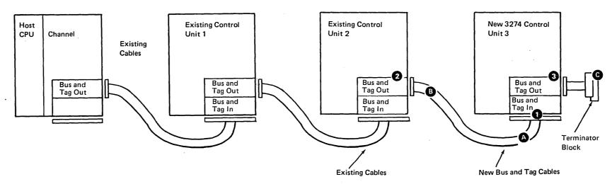
Caution: Before removing any terminator block from an existing control unit, ensure that the CPU/channel state will permit removal of the block with no adverse effect.
