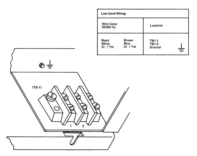
Figure B-4. Primary Power Box, -24 V Transformer Wiring and Line Cord Connections
