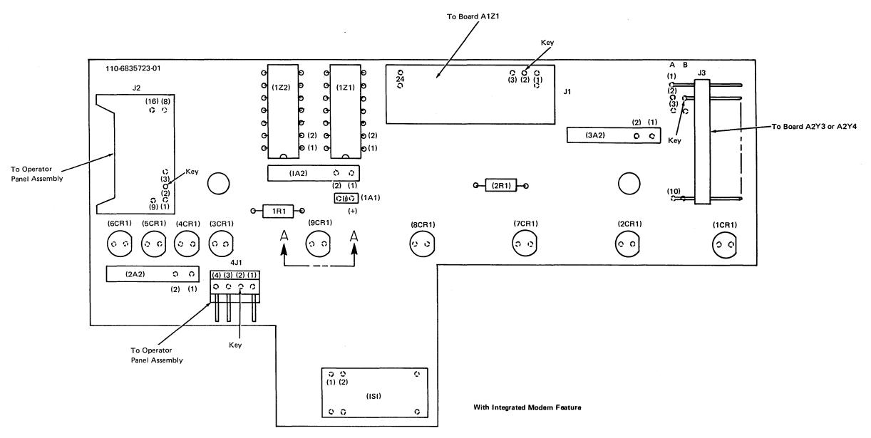
Figure E-2 (Part 2 of 2). Operator Panel Indicator Card
