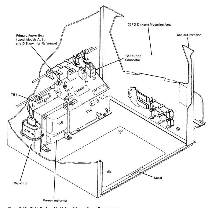
Figure B-10. Field Replaceable Unit — Primary Power Components
