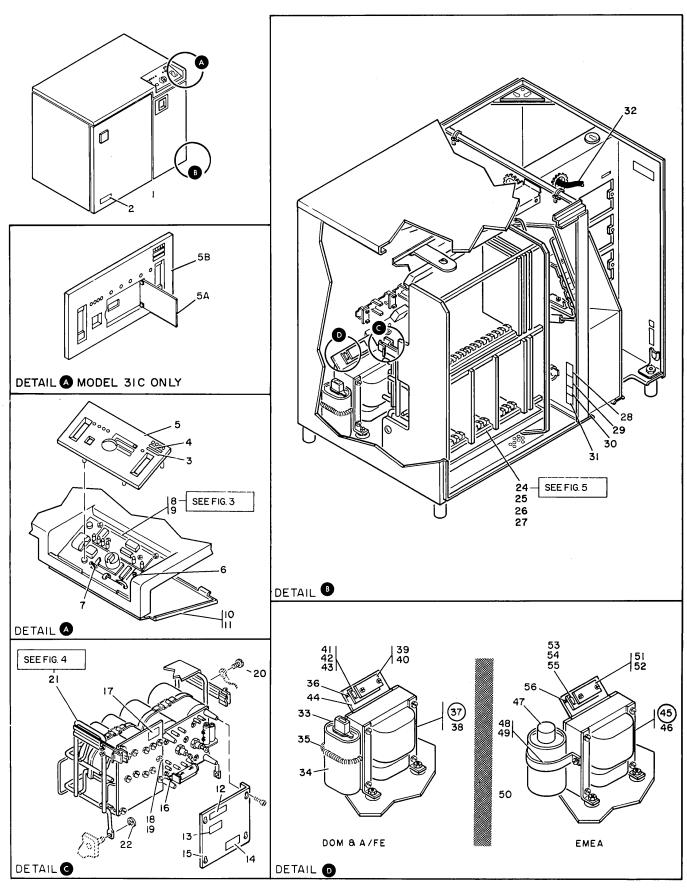
FIGURE 2. FINAL ASSEMBLY. SHEET 1 OF 2. INDEX NOS. 1-56. SEE LIST 2.
