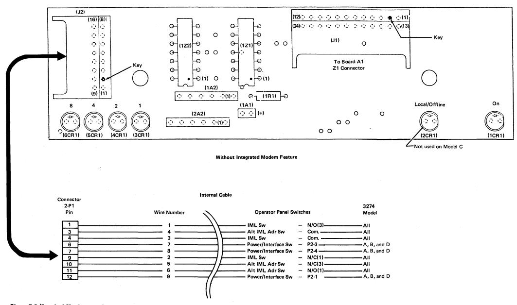
Figure E-2 (Part 1 of 2). Operator Panel Indicator Card
