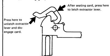
(b) Replacement — Open both extractor levers fully. Insert the card holder tracks into the front guide fingers (card components toward right). Do not use the extractor levers to reseat the card. Apply firm finger pressure to the card holder (or connector housing for double-ended cards) to ensure proper contact seating.
