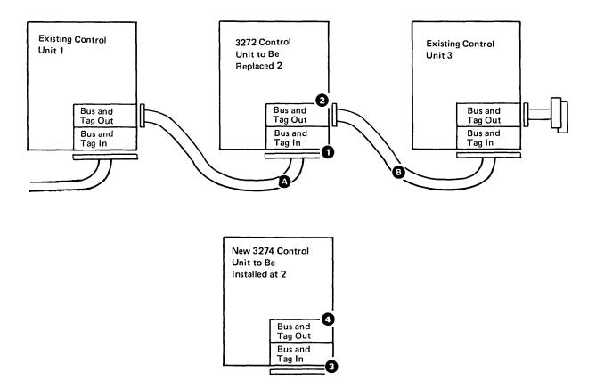
Caution: Before removing any Bus and Tag cables from an existing control unit, ensure that the CPU/channel state will permit removal of the cables.
