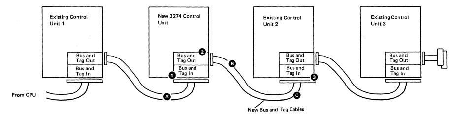
Caution: Before removing any Bus and Tag cables from an existing control unit, ensure that the CPU/channel state will permit removal of the cables.
