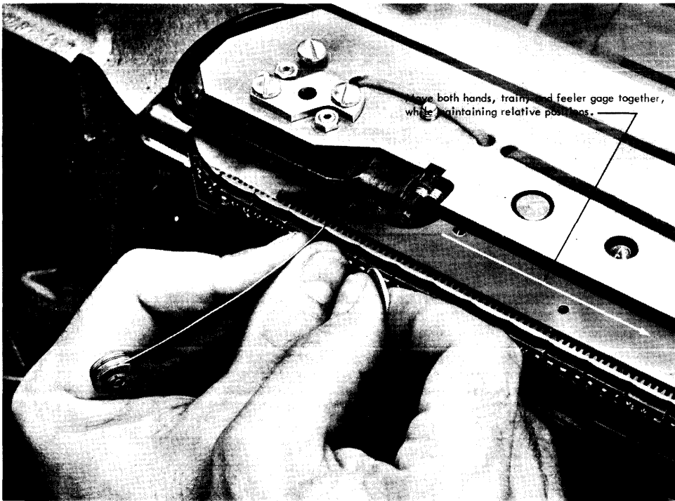
Figure 77. Method of Checking Accumulated Interslug Gap
