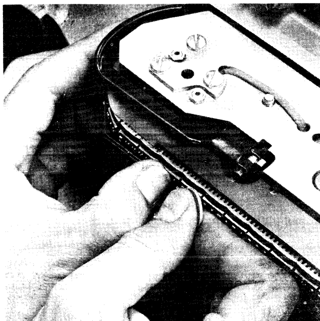
Figure 75. Method of Separating Type Slugs
