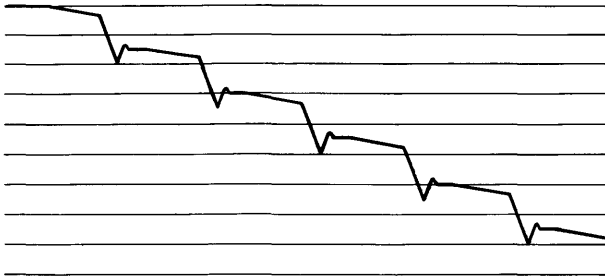
Figure 51. Bypass Adjusted too Tight (Hydraulic Bounce)
