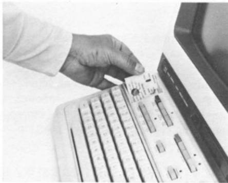
B. INSTALLING BAUDRATE OVERLAY
