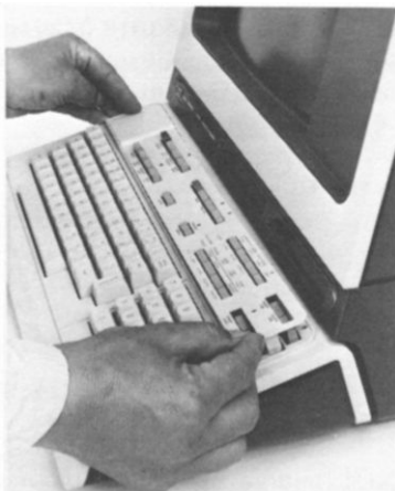
C. INSTALLING KEYBOARD OVERLAY
