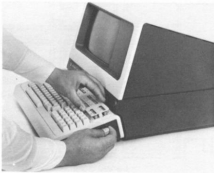
A. REMOVING A KEYBOARD OVERLAY
