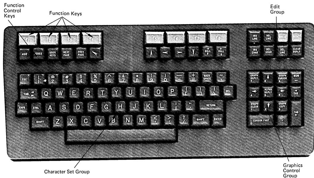
Figure D-23. HP2623A and HP2627A Keyboard
