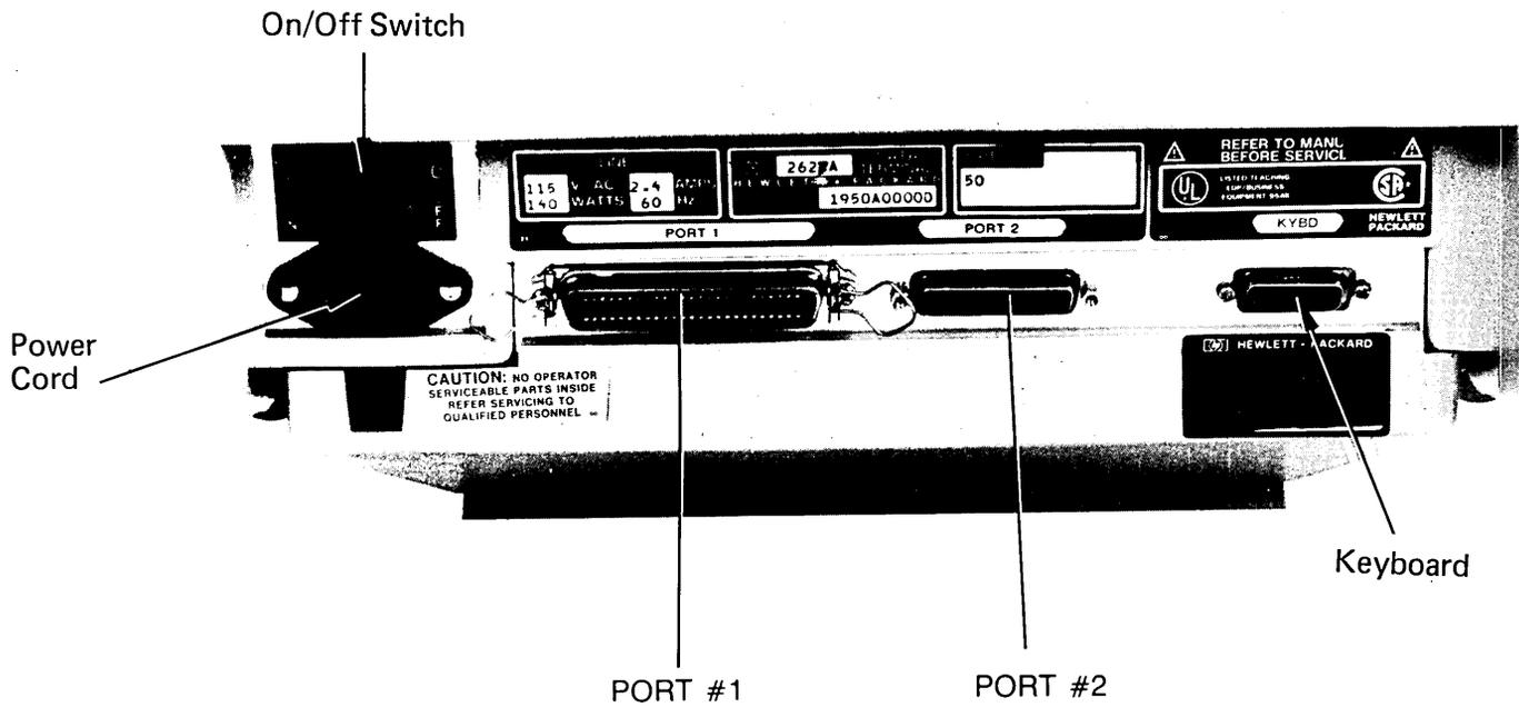
Figure D-22. HP2623A and HP2627A Rear View
