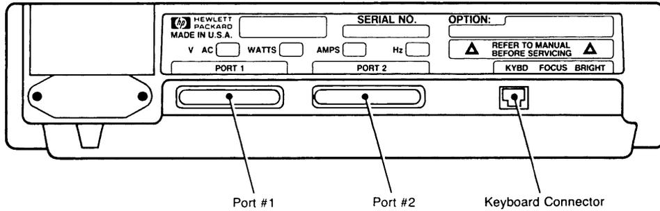
Figure D-24. HP2625A and HP2628A Rear View
