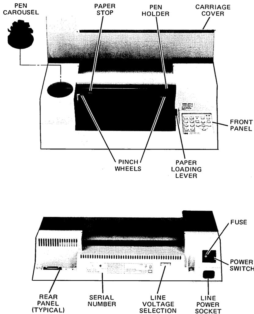
Figure D-13. Front and Rear View
