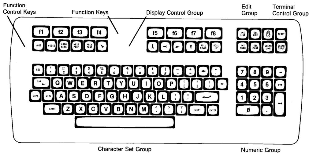
Figure D-25. HP2625A and HP2628A Keyboard
