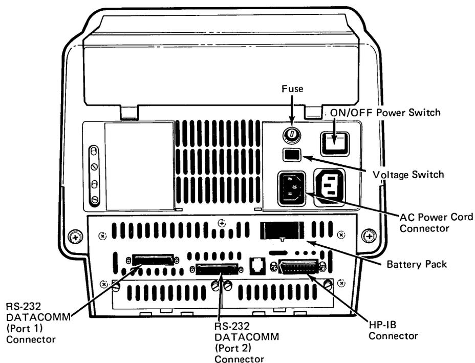
Figure D-27. HP 150 Rear View
