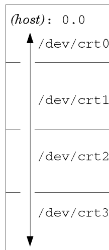
Figure 4-6. Four Physical Displays, Single Logical Screen (4×1)
