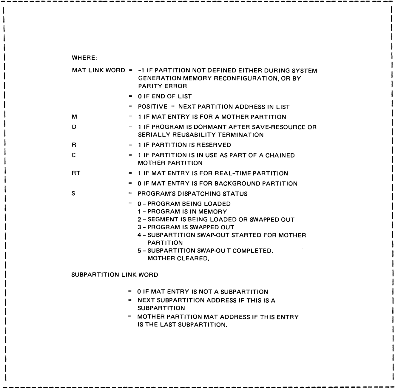
Figure I-4. Memory Allocation Table Entry Format
