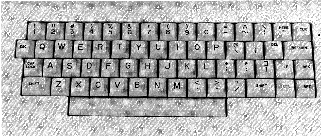
Figure 7-3. TWU9104/9106 Keyboard Configuration
